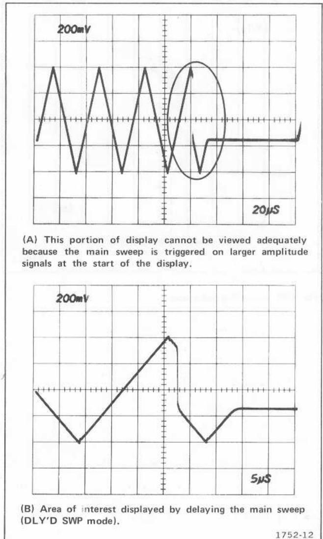
Fig. 2-11. Displaying a complex signal using delayed sweep.
