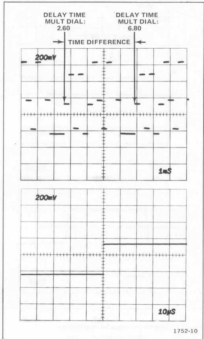
Fig. 2-9. Measuring time difference using delayed sweep.
