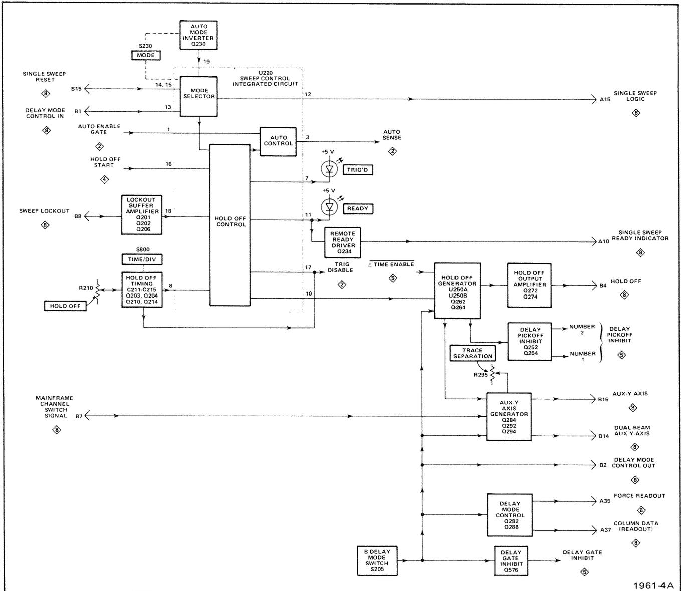
Fig. 3-5. Detailed block diagram of Logic circuit.
