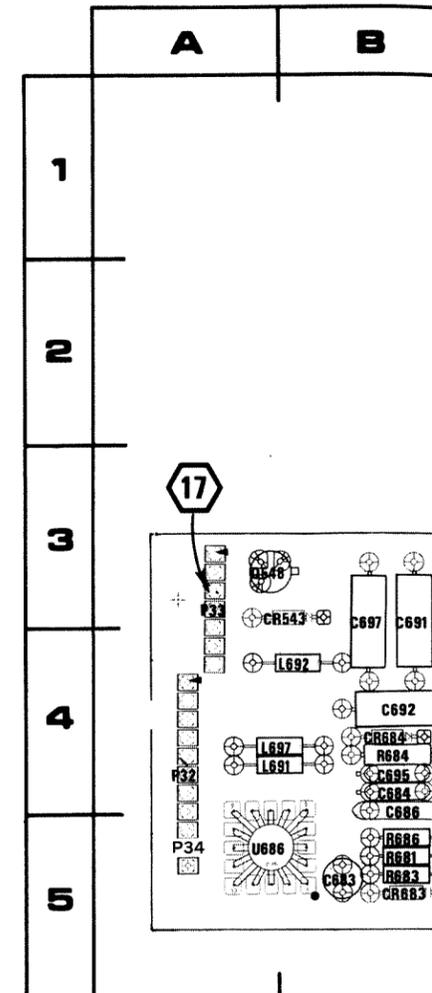
Fig. 8-9A. A4—(SN B088750 & Up) Digital Voltmeter circuit board assembly.
