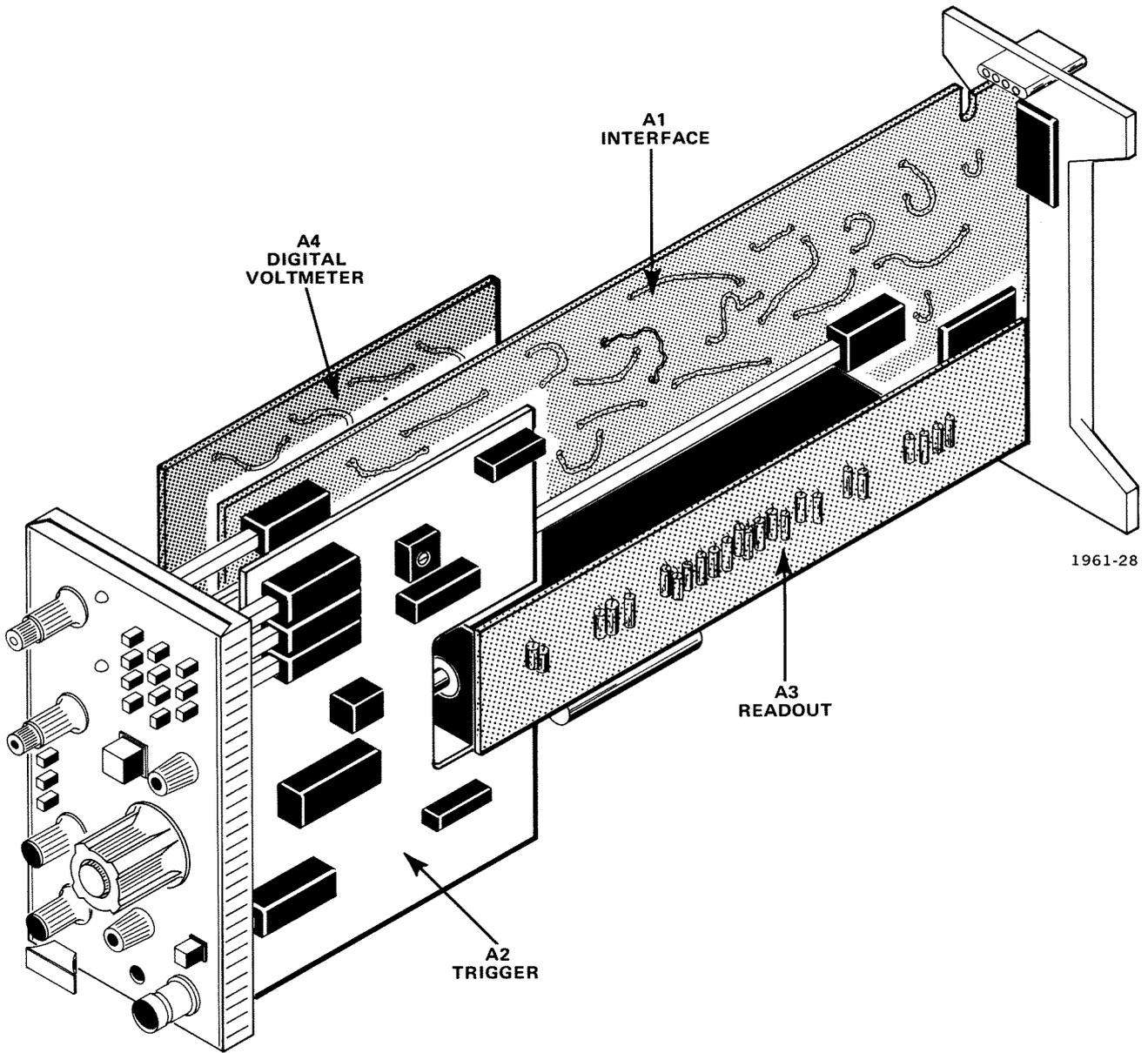
Fig. 8-2. Location of circuit boards in the 7B85.
