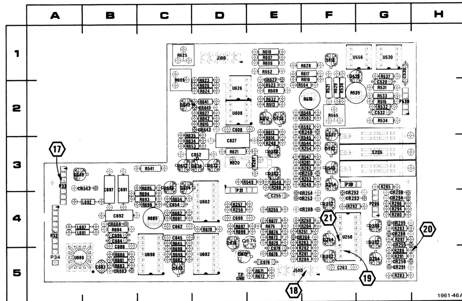
Fig. 8-9B. A4--(SN B088749 & Below) Digital Voltmeter circuit board assembly.
