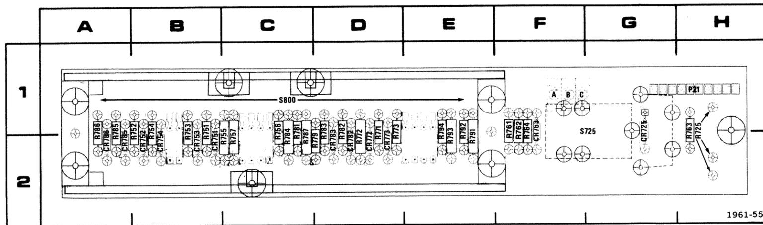
Fig. 8-10. A3-Readout circuit board assembly.
