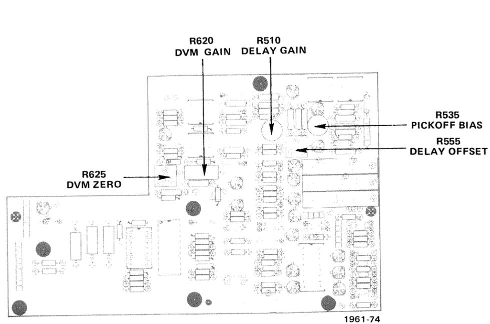
Fig. 8-13A. (SN B088750 & Up) Location of Digital Voltmeter adjustments.
