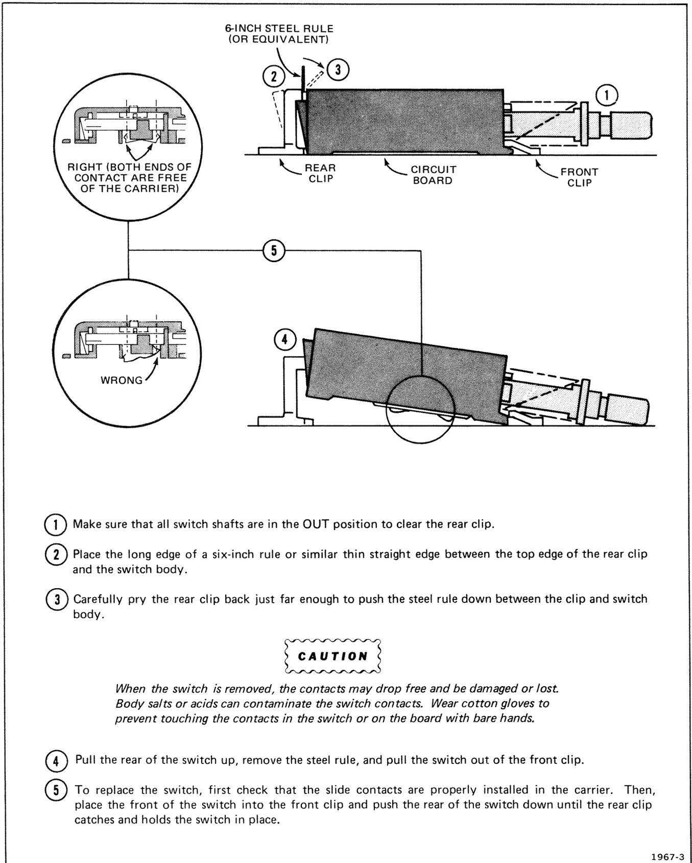
Fig. 4-10. Removal procedure for typical push-button switch.
