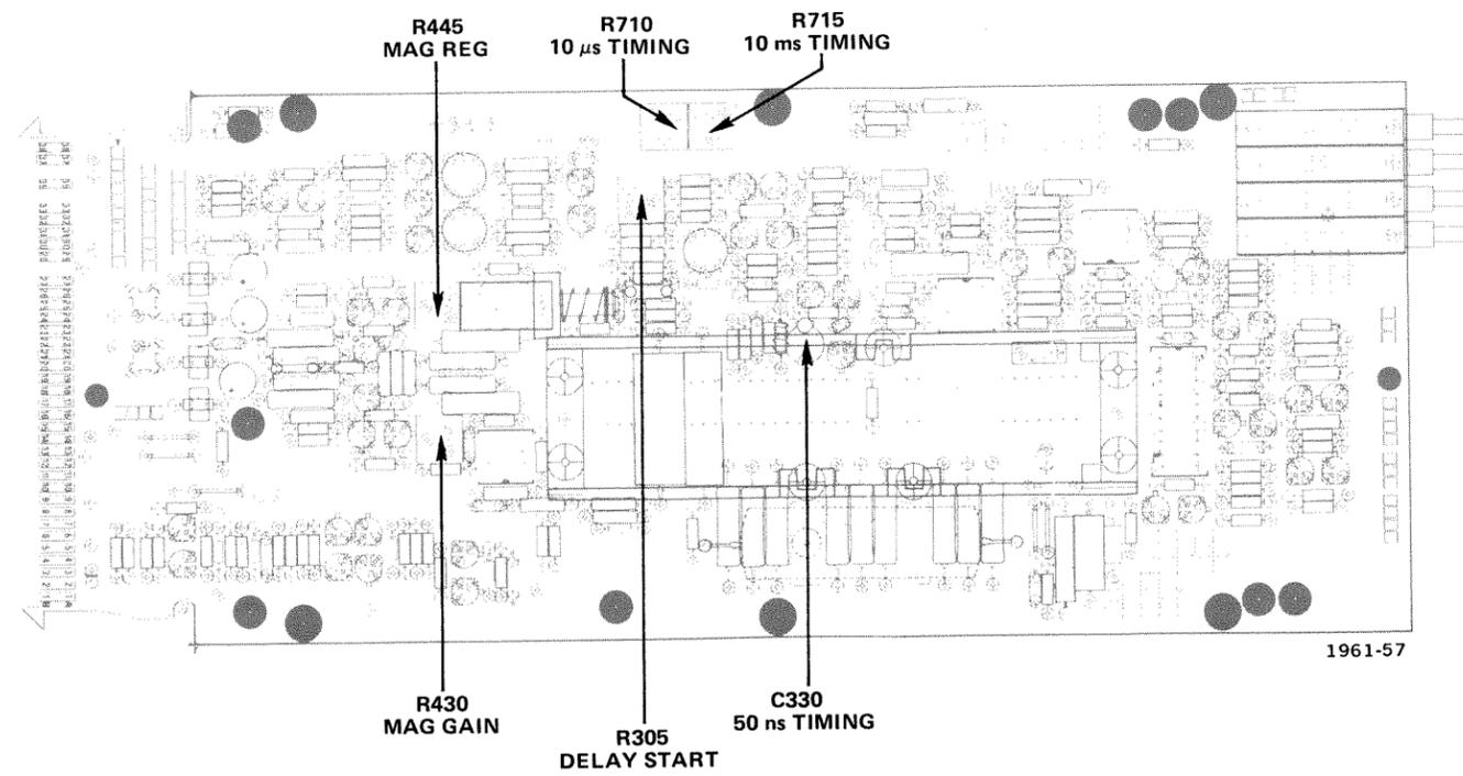
Fig. 8-11. Location of Sweep Timing adjustments.
