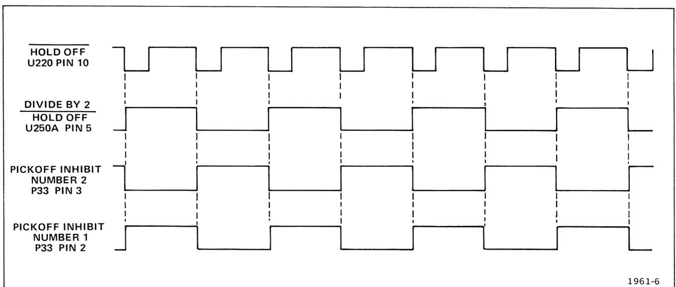
Fig. 3-6. Timing diagram for Delay Pickoff Inhibit stage.
