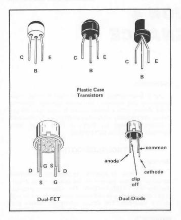
Fig. 4-1. Electrode configuration for semiconductors in the 7A15A/ 7A15AN.
