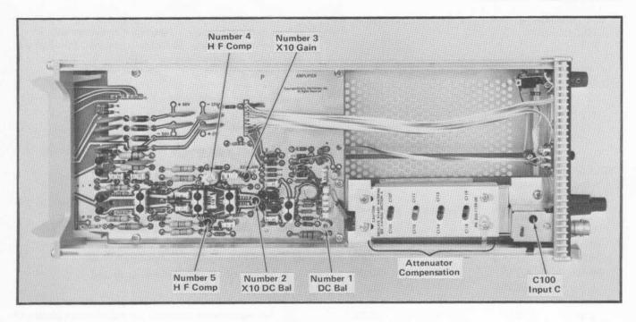
Fig. 5-1. Location of adjustments for 7A15A/7A15AN. (7A15A shown)
