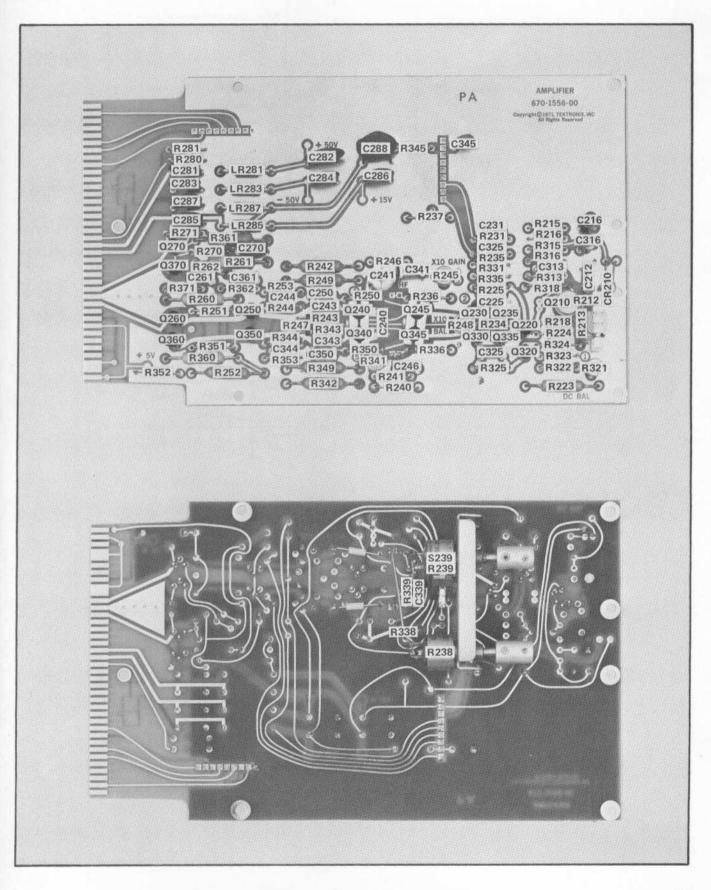
Fig. 7-2. Amplifier circuit board and component location.
