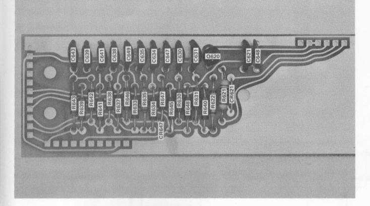
Fig. 7-1. Readout circuit board with component location (7A15A Only).
