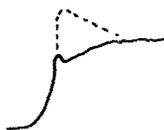
First nanosecond of waveform too positive or negative may be corrected by changing length of L730 and L731. (See Fig. 5-4 for location.)
