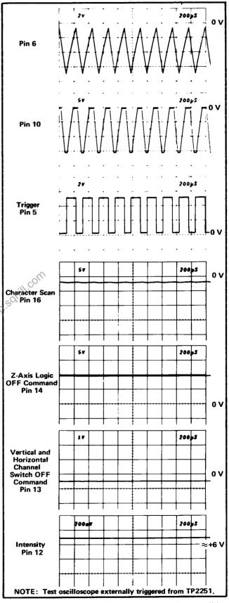
Fig. 3-30. Timer stage operation when Display-Skip condition occurs.
