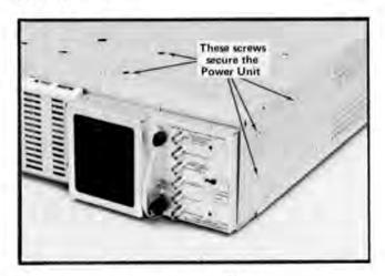
Fig. 4-1. Power unit removal for the R7613.
