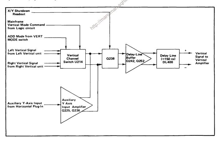
Fig. 3-16. Vertical Interface detailed block diagram.
