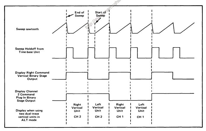
Fig. 3-11. Idealized waveforms showing relationship between input and output waveforms for Vertical Binary and Plug-In Binary stages when operating in ALT mode.
