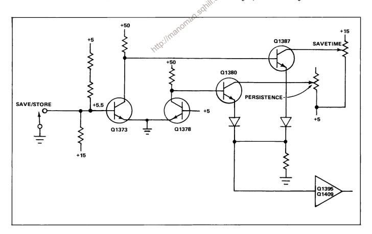
Fig. 3-39. Variable Persistence and Save switching circuit.
