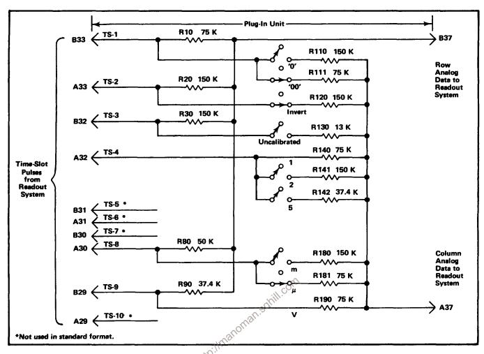
Fig. 3-32. Typical encoding scheme for voltage-sensing amplifier plug-in unit. Coding shown for deflection factor of 100 microvolts.
