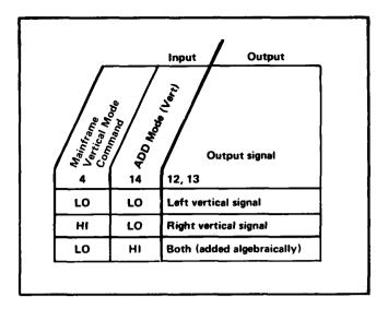
Fig. 3-17. Input/output table for Vertical Channel Switch.
