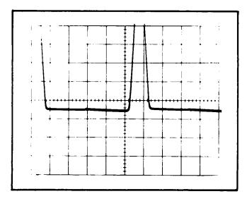
Fig. 2-5. Test oscilloscope waveforms when horizontal limit centering is properly adjusted.
