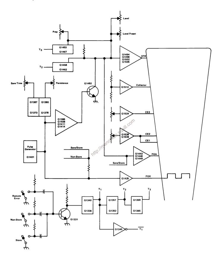
Fig. 3-38. Basic Storage Block Diagram.
