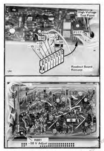
Fig. 2-1. (A) Location of power supply and high-voltage test points (right side of instrument); (B) Location of -50 V adjustment (Low Voltage Regulator board).
