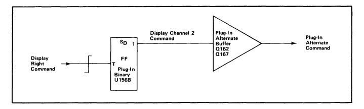
Fig. 3-12. Logic diagram of Plug-In Binary and Plug-In Alternate Buffer stages.
