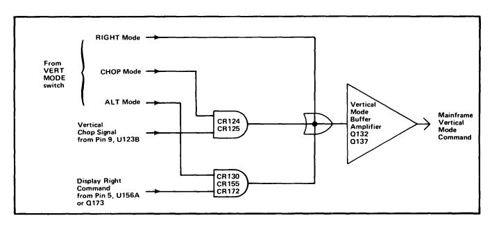
Fig. 3-9. Logic diagram of Vertical Mode Control and Vertical Mode Buffer Amplifier stages.
