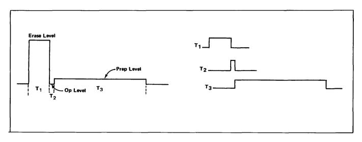
Fig. 3-41. Erase cycle out of Storage Target Backplate.
