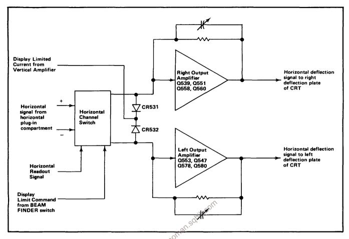
Fig. 3-19. Horizontal Amplifier detailed block diagram.
