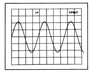
Fig. 3-26. Typical readout display where only channel 1 of the Right Vertical and Horizontal units is displayed.
