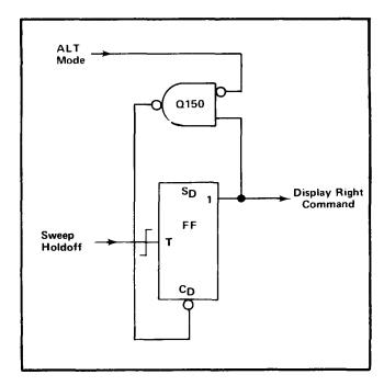
Fig. 3-10. Logic diagram of Vertical Binary stage.
