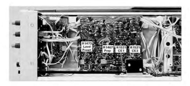
Fig. 2-9. Location of adjustment on storage board.
