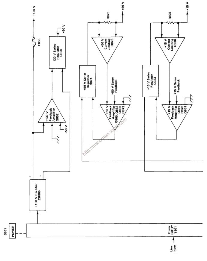
Fig. 3-22. Low-Voltage Power Supply detailed block diagram.
