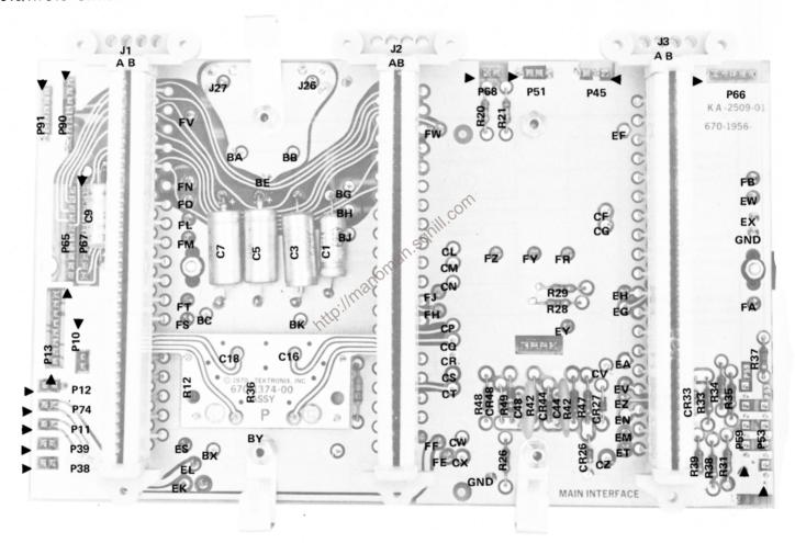
FIG. 6-2A. A1-Main Interface (front) circuit board SN B240000 & up.
