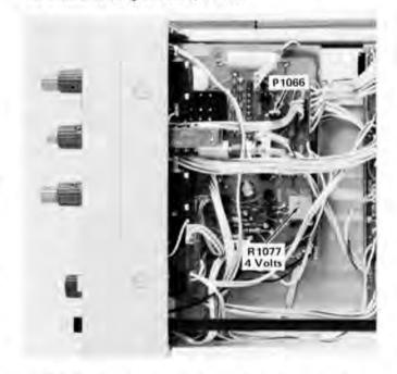
Fig. 2-8. Location of Calibrator adjustments (Calibrator board).
