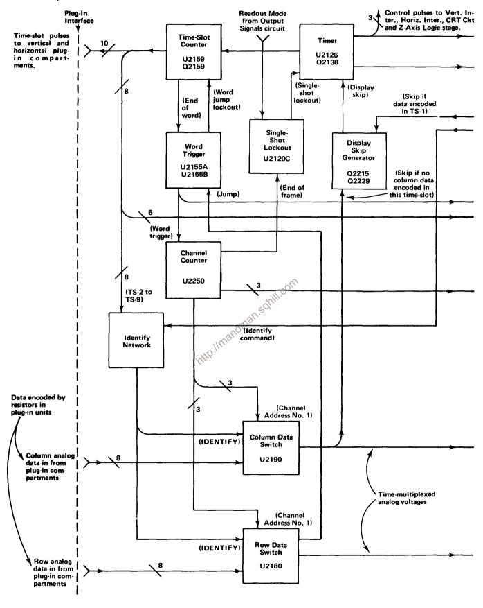
Fig. 3-27. Detailed block diagram of Readout System.
