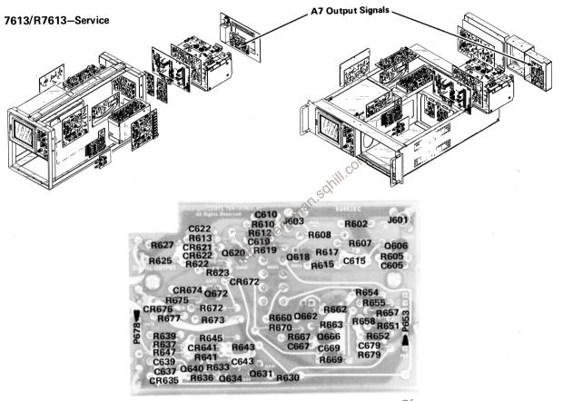
Fig. 6-9. A7. Signal Output circuit board.
