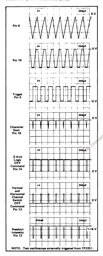
Fig. 3-28. Output waveforms of Timer stage.
