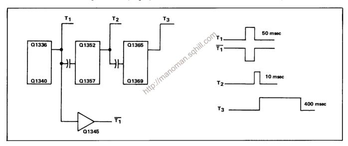
Fig. 3-40. Erase timing pulse generator.
