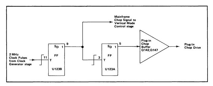
Fig. 3-7. Detailed logic diagram of Chop Counter stage.
