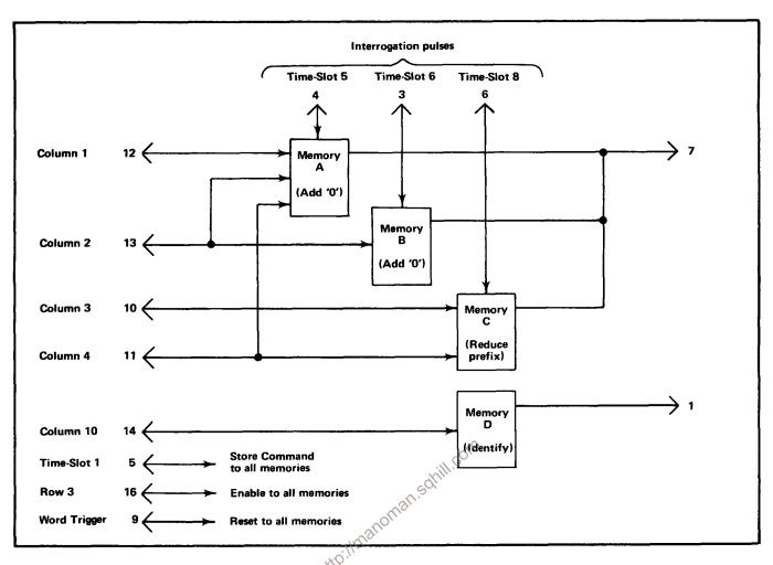
Fig. 3-34. Block representation of memory sequence in U2232.
