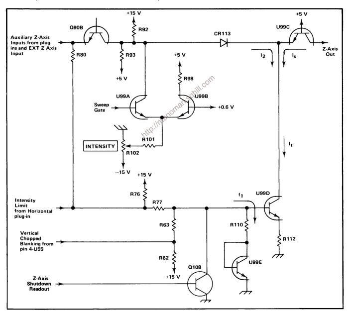
Fig. 3-3. Simplified schematic of Z-Axis Logic stage.
