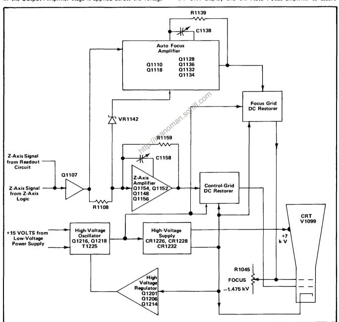
Fig. 3-21. CRT Circuit detailed block diagram.
