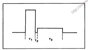
Fig. 2-10. Erase pulses from Storage Target Backplate Amplifier.
