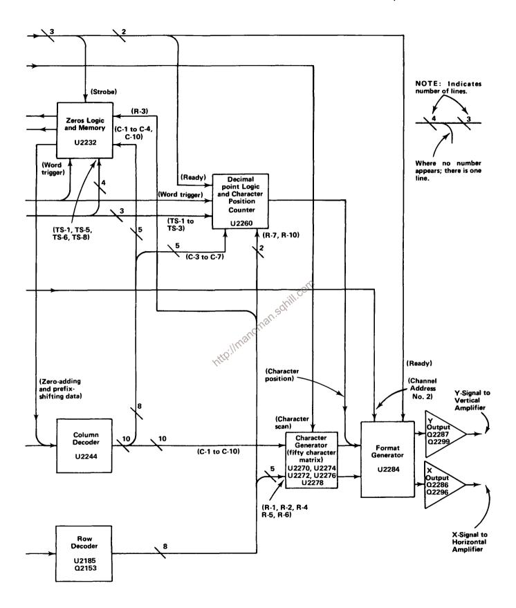
Fig. 3-27. Detailed block diagram of Readout System (cont).
