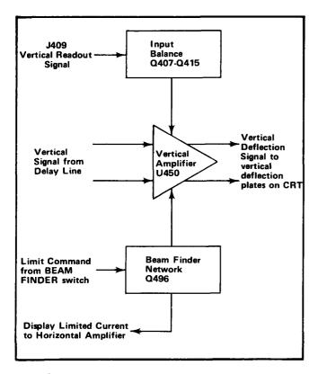
Fig. 3-18. Vertical Amplifier detailed block diagram.
