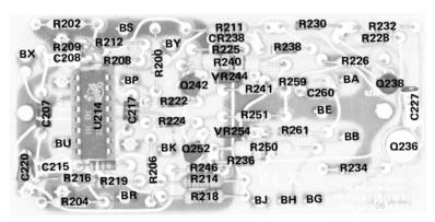
Fig. 6-6. A3. Vertical Interface circuit board.
