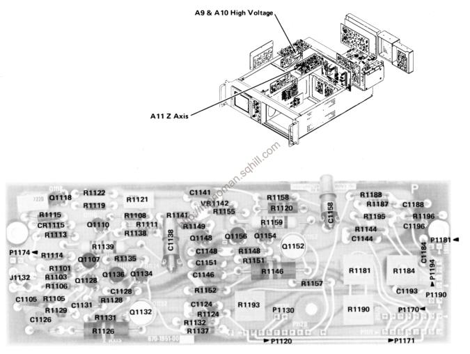
Fig. 6-12. A11. Z Axis circuit board.
