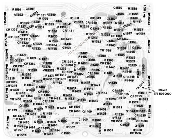
Fig. 6-15. A15. Storage circuit board.
