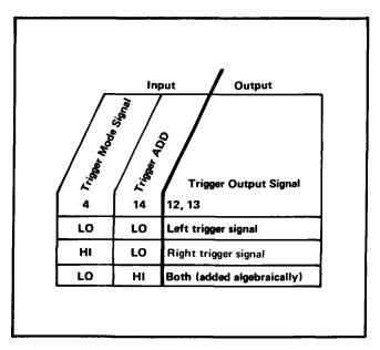
Fig. 3-15. Input/output table for Trigger Channel Switch stage.
