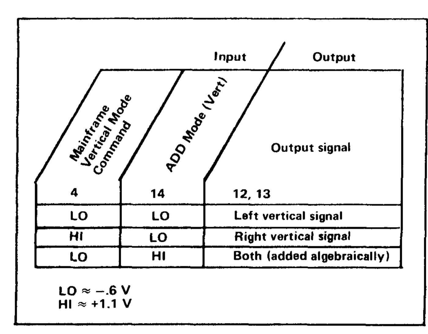
Fig. 3-17A. Input/output table for Vertical Channel Switch.
