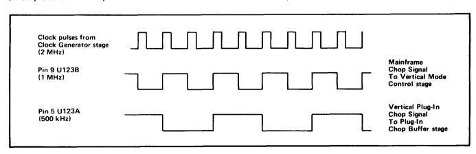
Fig. 3-8. Idealized input and output waveforms for Chop Counter stage.
