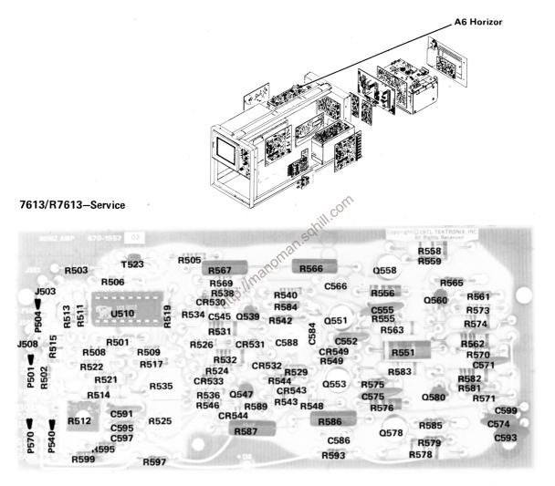
Fig. 6-8A. A6. Horizontal Amplifier circuit board, SN B070000-up. REV. MAY 1974 (A)
