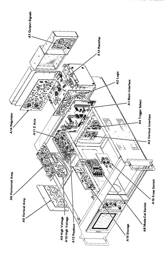
Fig. 4-3. Location of circuit boards in the R7613.
