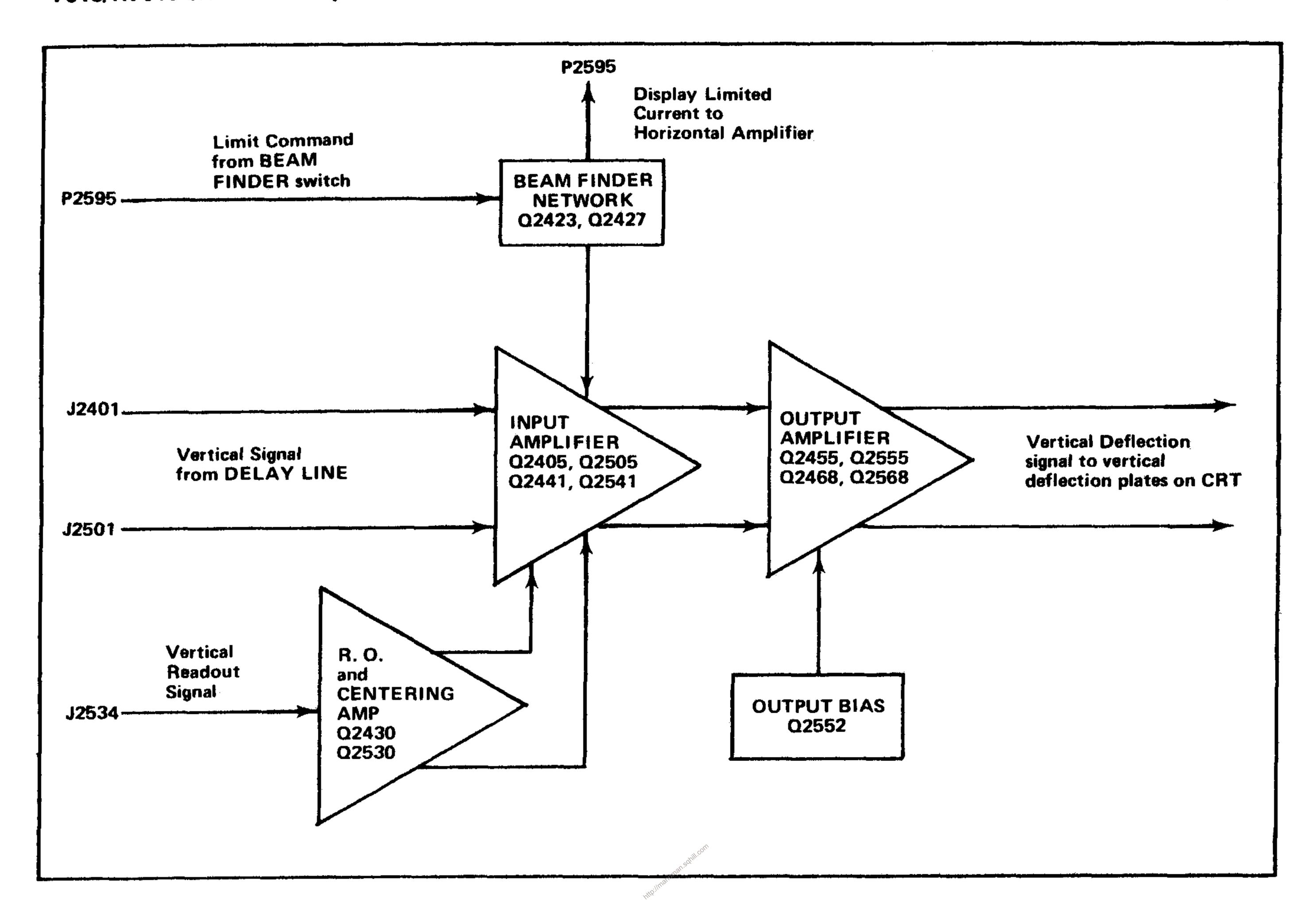
Fig. 3-18A. Vertical Amplifier detailed block diagram for SN B150000 and up.
