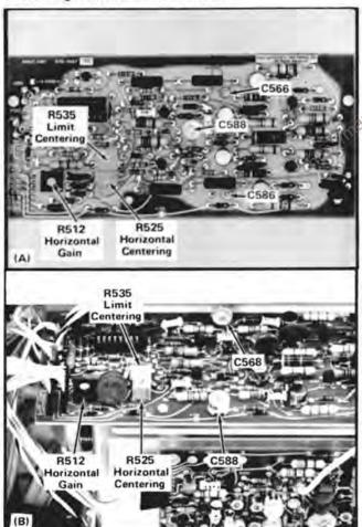
Fig. 2-6. Location of Horizontal adjustments (Horizontal Amplifier board (A) SNB020000-up; (B) Below SNB020000,
