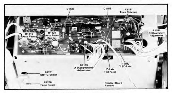
Fig. 2-2. Location of Display and Z Axis adjustments and test points.
