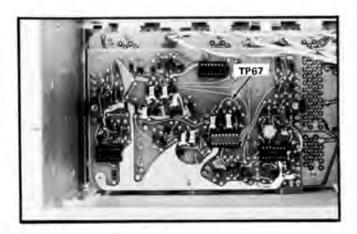
Fig. 2-4. Location of TP67 on Logic board (shown with power unit removed).
