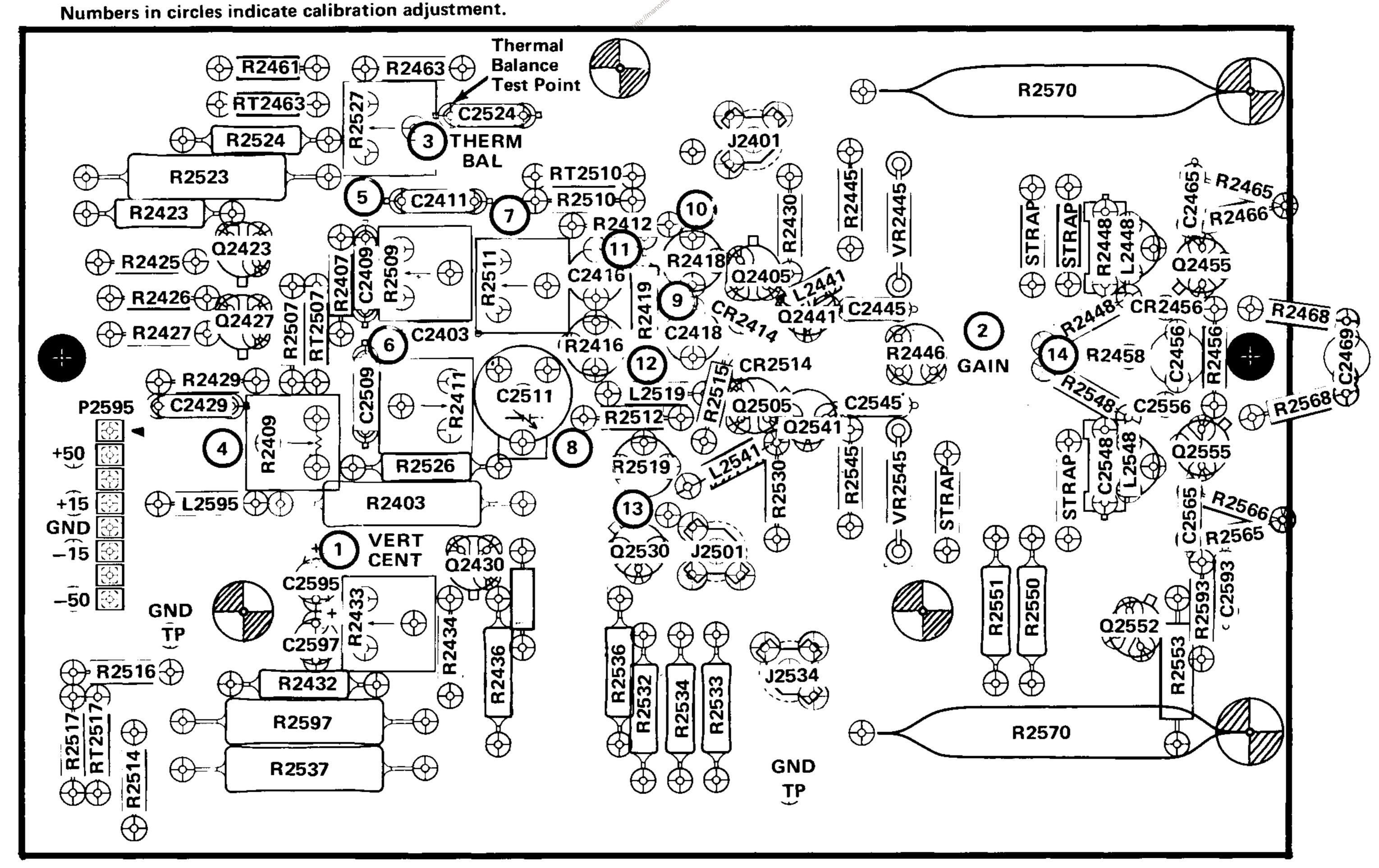
Fig. 6-7A. A5. Vertical Amplifier circuit board, SN B150000-up
