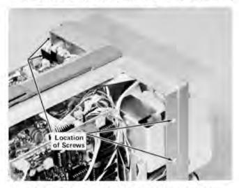
Fig. 4-7. Location of screws holding Low Voltage sub-chassis.
