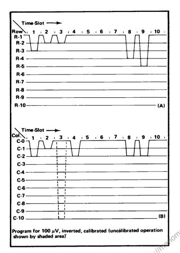
Fig. 3-33. Idealized current waveforms of: (A) Row analog data, (B) Column analog data.
