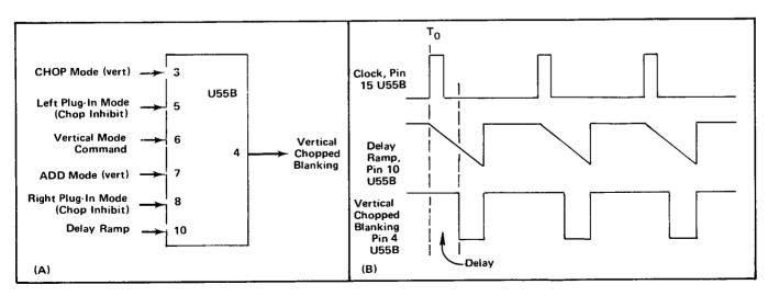
Fig. 3-5. (A) Input and output pins for Vertical Chopped Blanking stage, (B) Idealized waveforms for Vertical Chopped Blanking stage.
