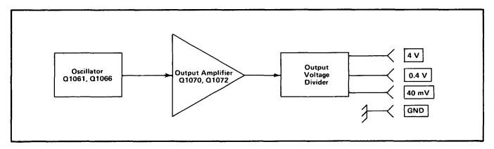
Fig. 3-20. Calibrator detailed block diagram.
