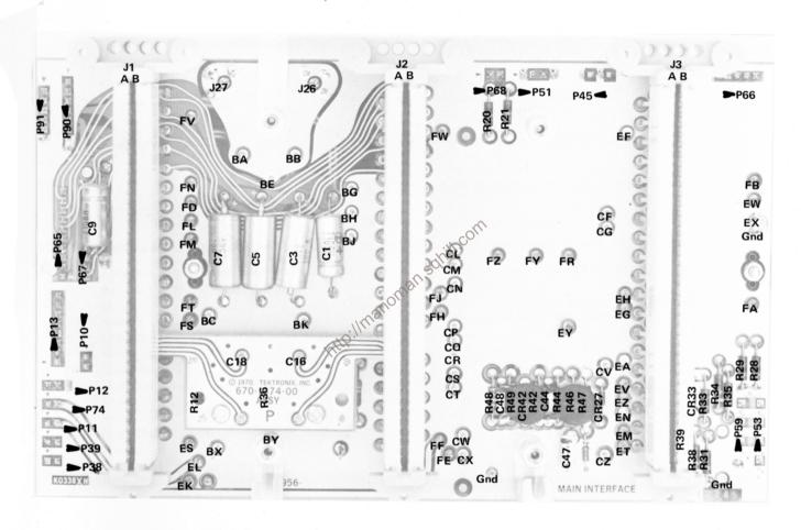
FIG. 6-2B. A1-Main Interface (front) circuit board below SN B240000.
