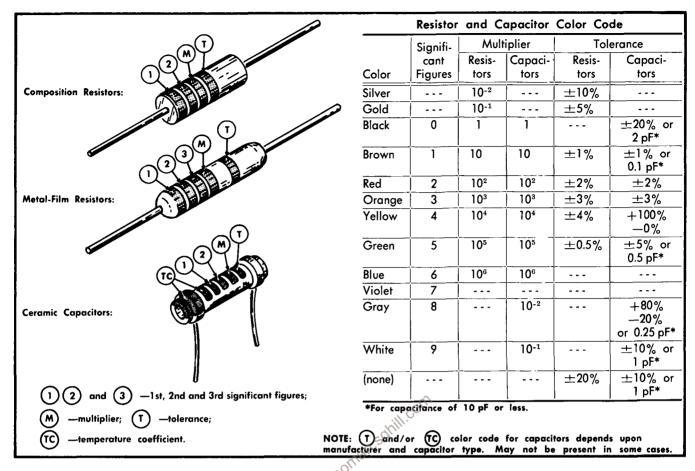
Fig. 4-4. Color code for resistors and ceramic capacitors.
