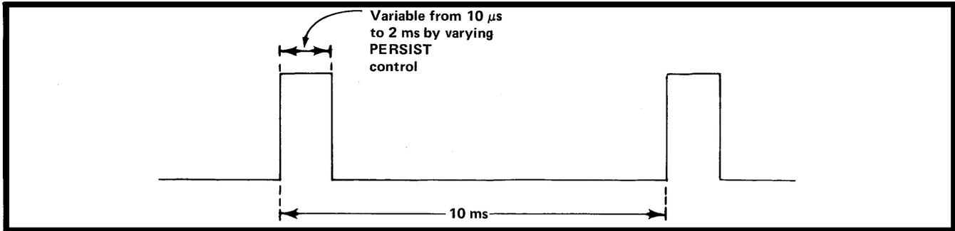
Fig. 2-2. Variable Persistence and Save circuit output waveform.
