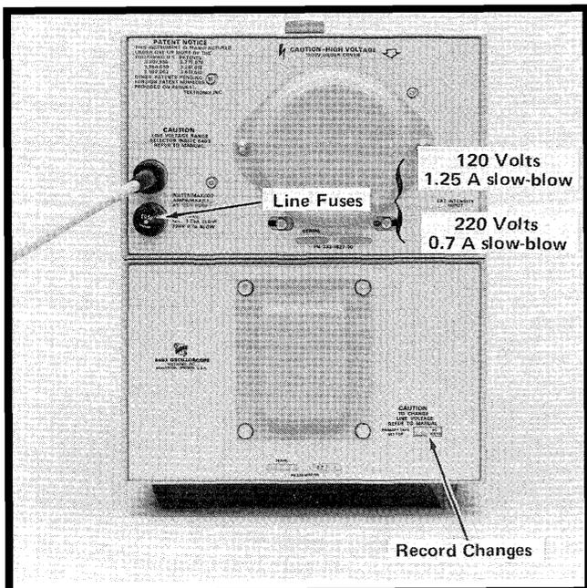
**Fig. 0-3. View showing rear-panel of power supply/amplifier module.**
