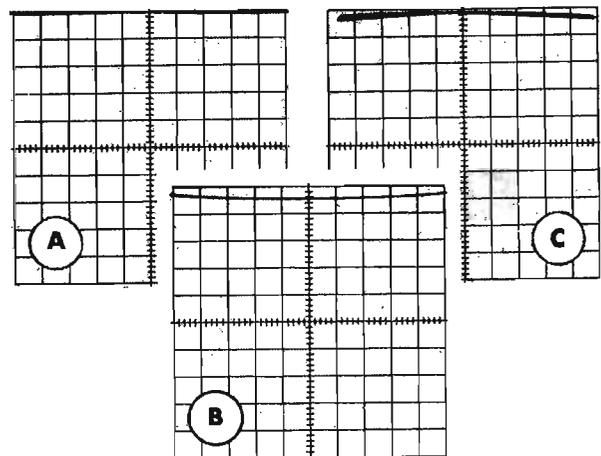
Fig. 6-3. Checking the geometry of the crt.
