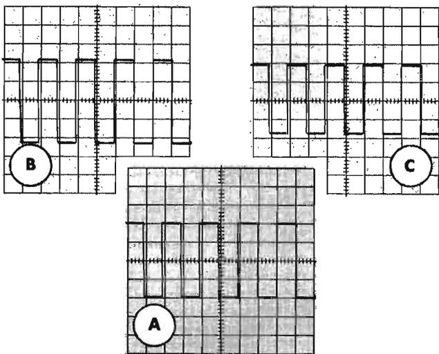
Fig. 6-4. Checking the gain of the vertical amplifier.
