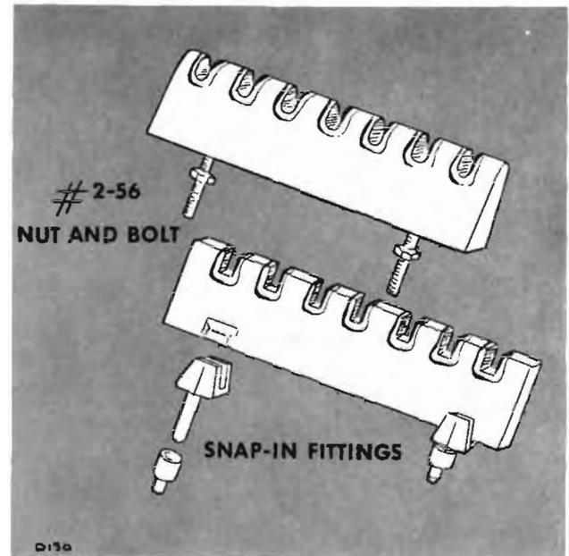
Fig. 5-7. Two types of ceramic strip mountings.
