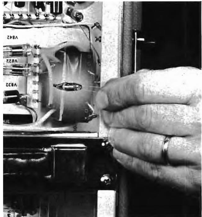
Fig. 5-9. Using a neon lamp to check for energy in the field of the high-voltage transformer.
