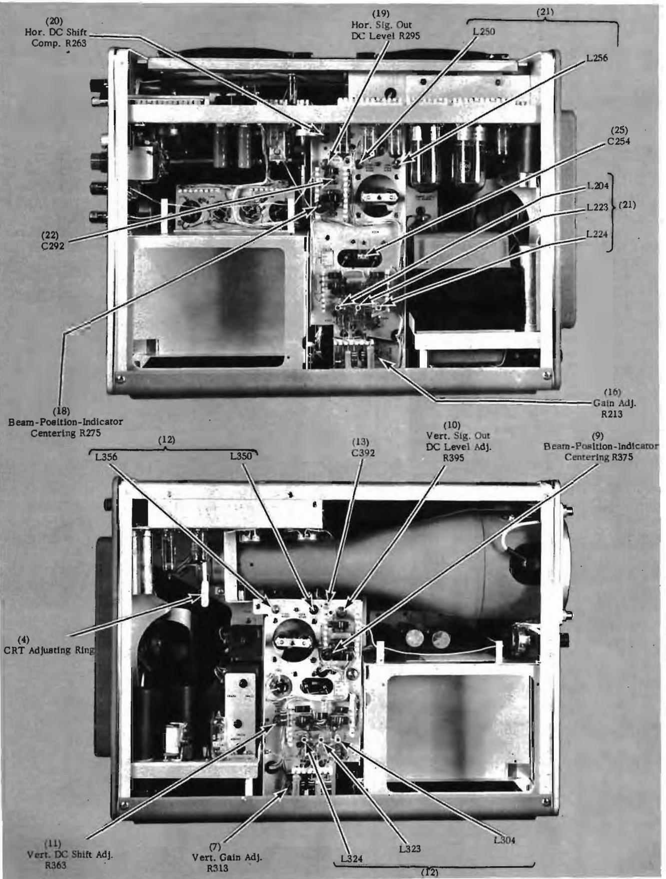
Fig. 6-16 Physical location of the circuits which compose the Type 536.
