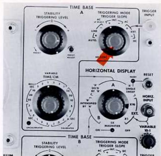
In this mode, the black TRIGGERING LEVEL control is not used. Final setting of the red STABILITY knob depends upon the nature of the synchronizing signal.
