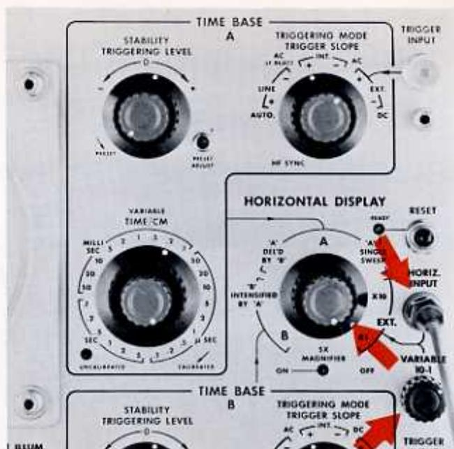
In this mode of operation, set the TRIGGERING MODE switch to some position other than AUTO. Also, set the red STABILITY knob as far to the left as possible, without actuating the PRESET switch.
