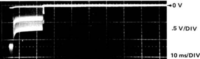
G.) At TP1926. Inverter Current Sens during sampling period with all supplies normal.
