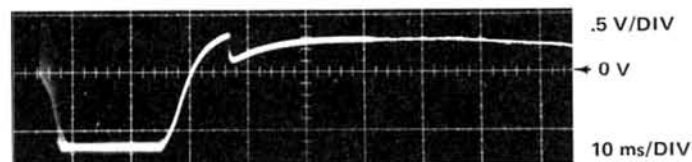
D.) At TP1951. Balance Node with power supply coming up during sampling period then falling off as supply shuts down due to short on +9 V supply.
