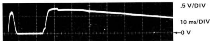
B.) At TP1951. Balance Node during sampling period with all supplies normal (test oscilloscope externally triggered on TP1926) then short applied to -9 V supply to cause second positive swing.
