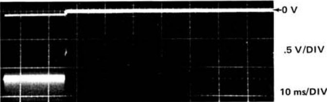
H.) At TP1926. Inverter Current Sens during sampling period with short on +15 supply.
