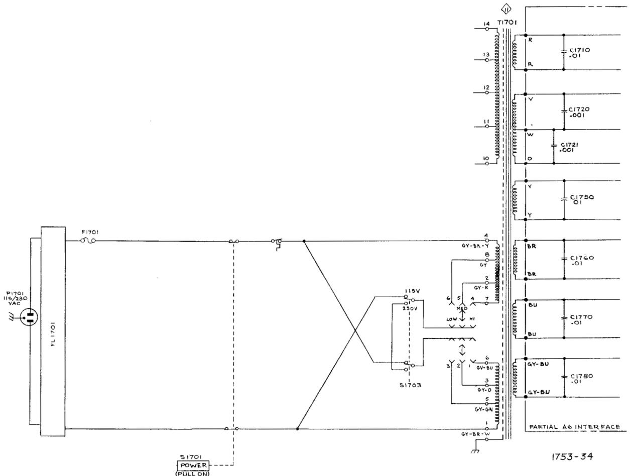
Fig. Option 4-1. 464 Option 4 primary winding with power-line filter.
