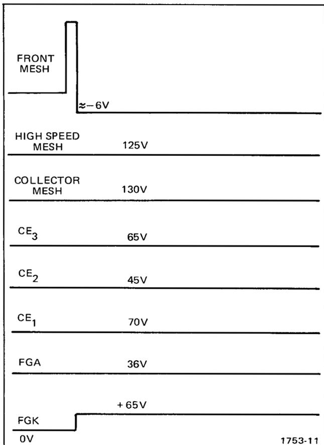
Fig. 3-11. Non-Store Mode—CRT Storage Element Voltage Levels.
