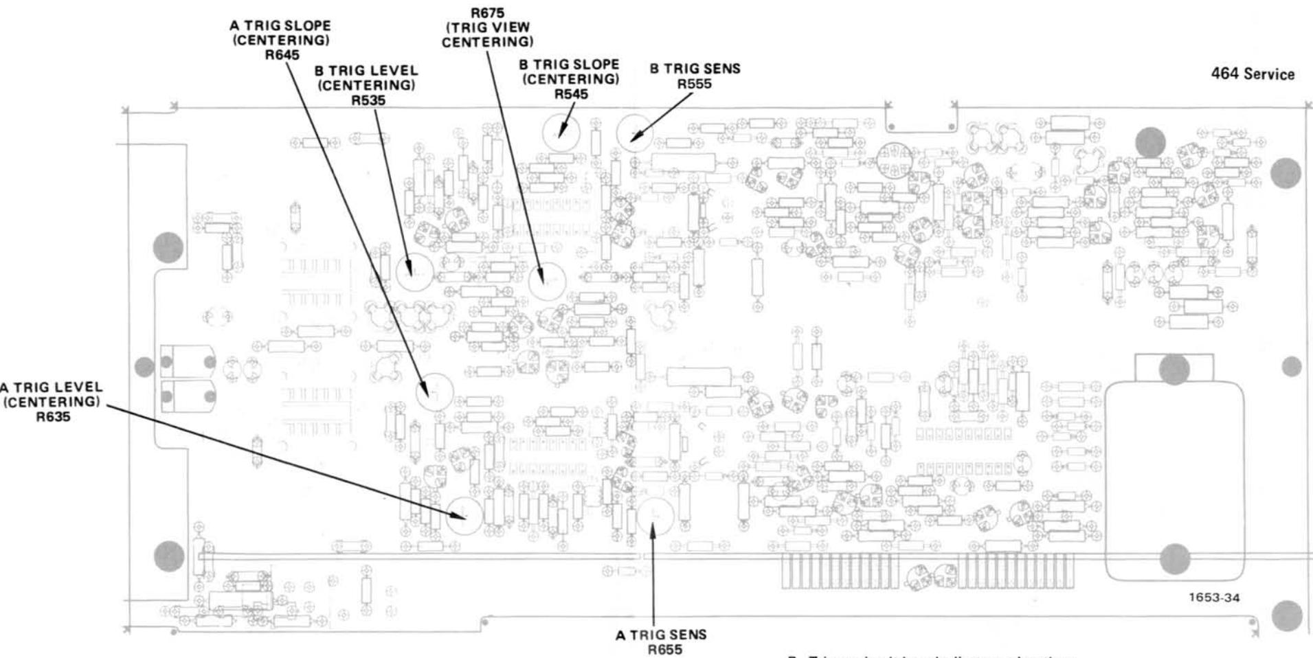
B. Trigger circuit board adjustment locations.
