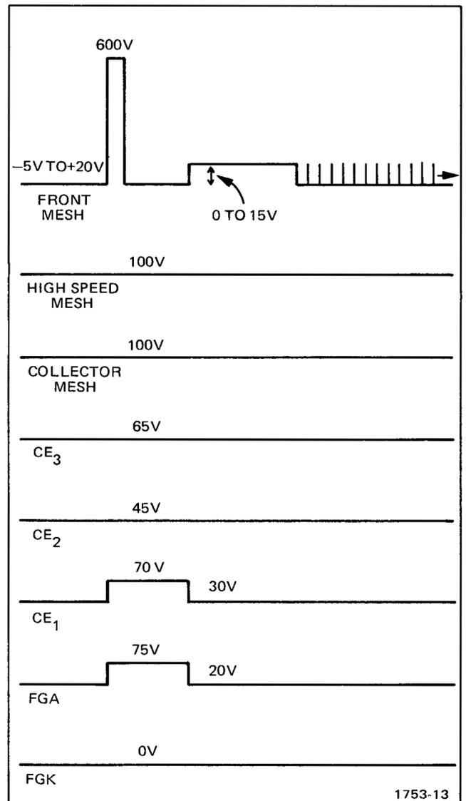
Fig. 3-12. Variable-Persistence Mode—CRT Storage Element Voltage Levels.
