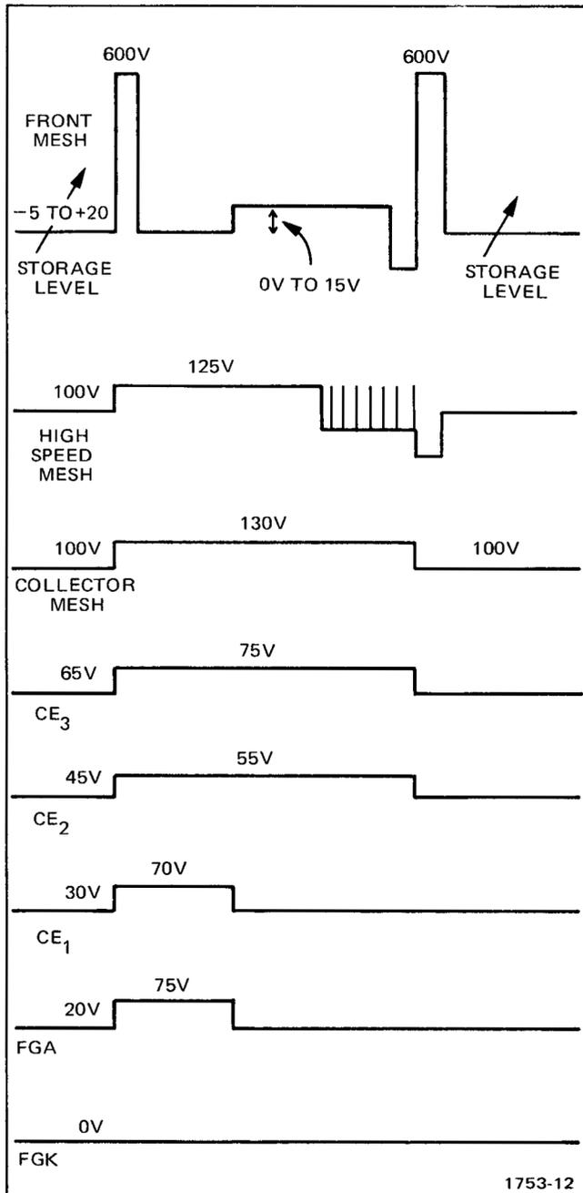
Fig. 3-13. Fast Mode—CRT Storage Element Voltage Levels.
