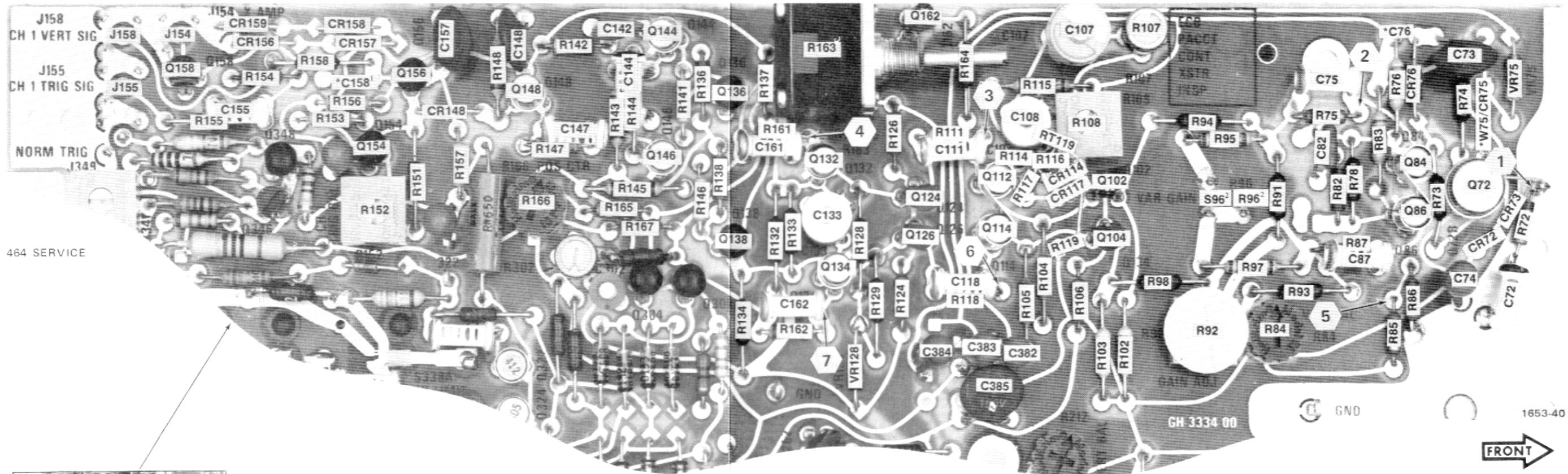
(A) Partial A2 Vertical Preamp circuit board.
