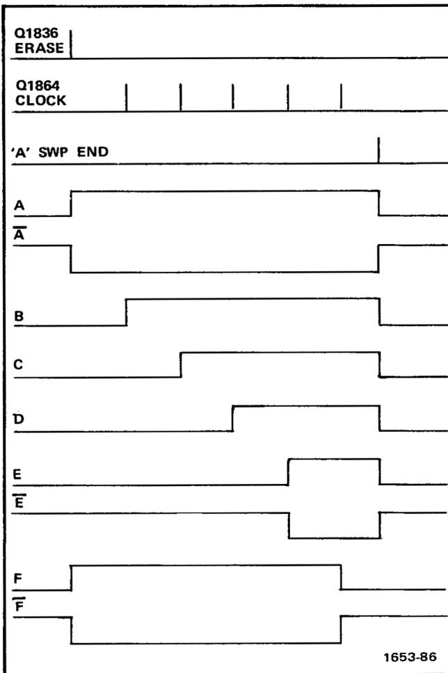
Fig. 3-8A. Shift Register and Storage Logic output.
