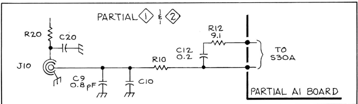
Fig. Option 5-4. Option 5 Vertical Input changes.
