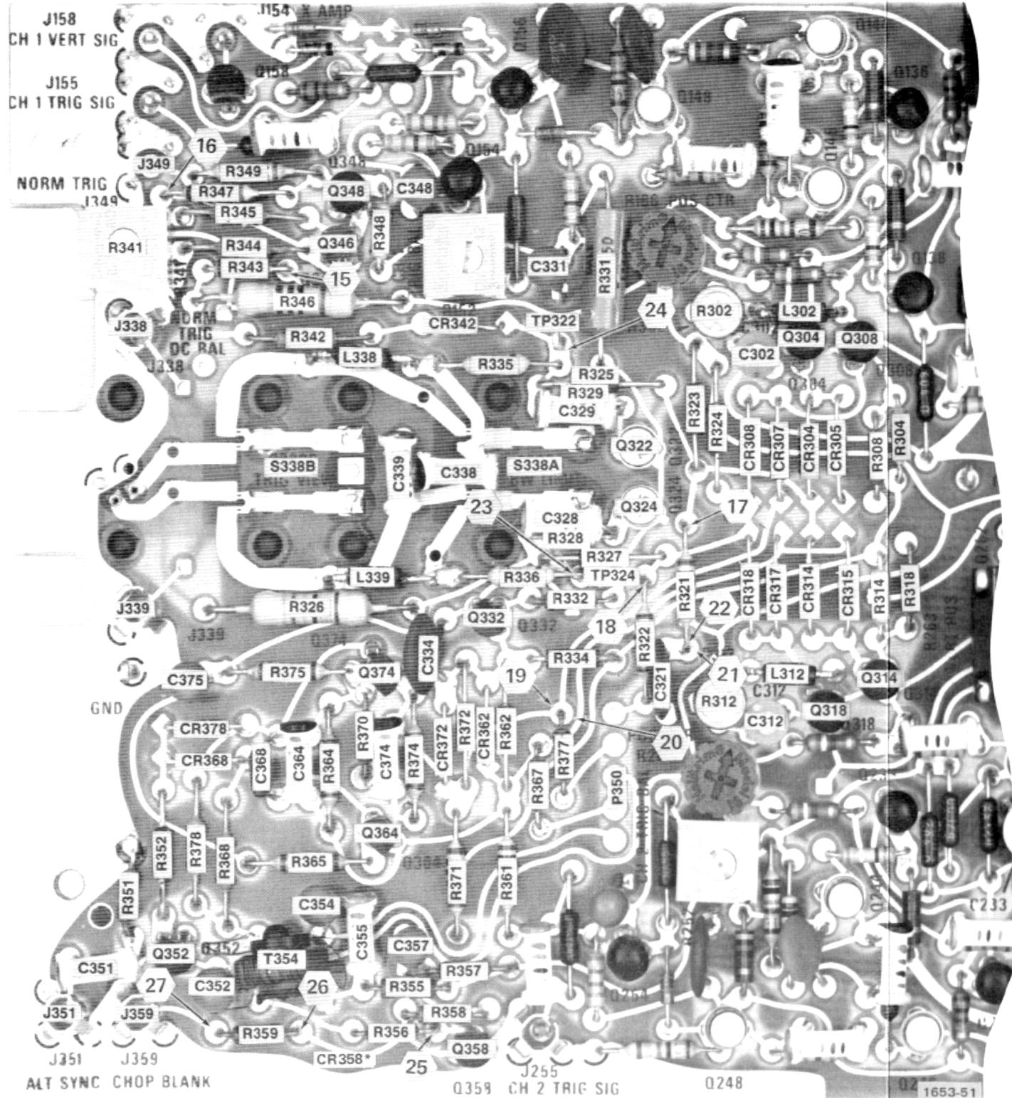
(A) Partial A2 Vertical Preamp circuit board.
