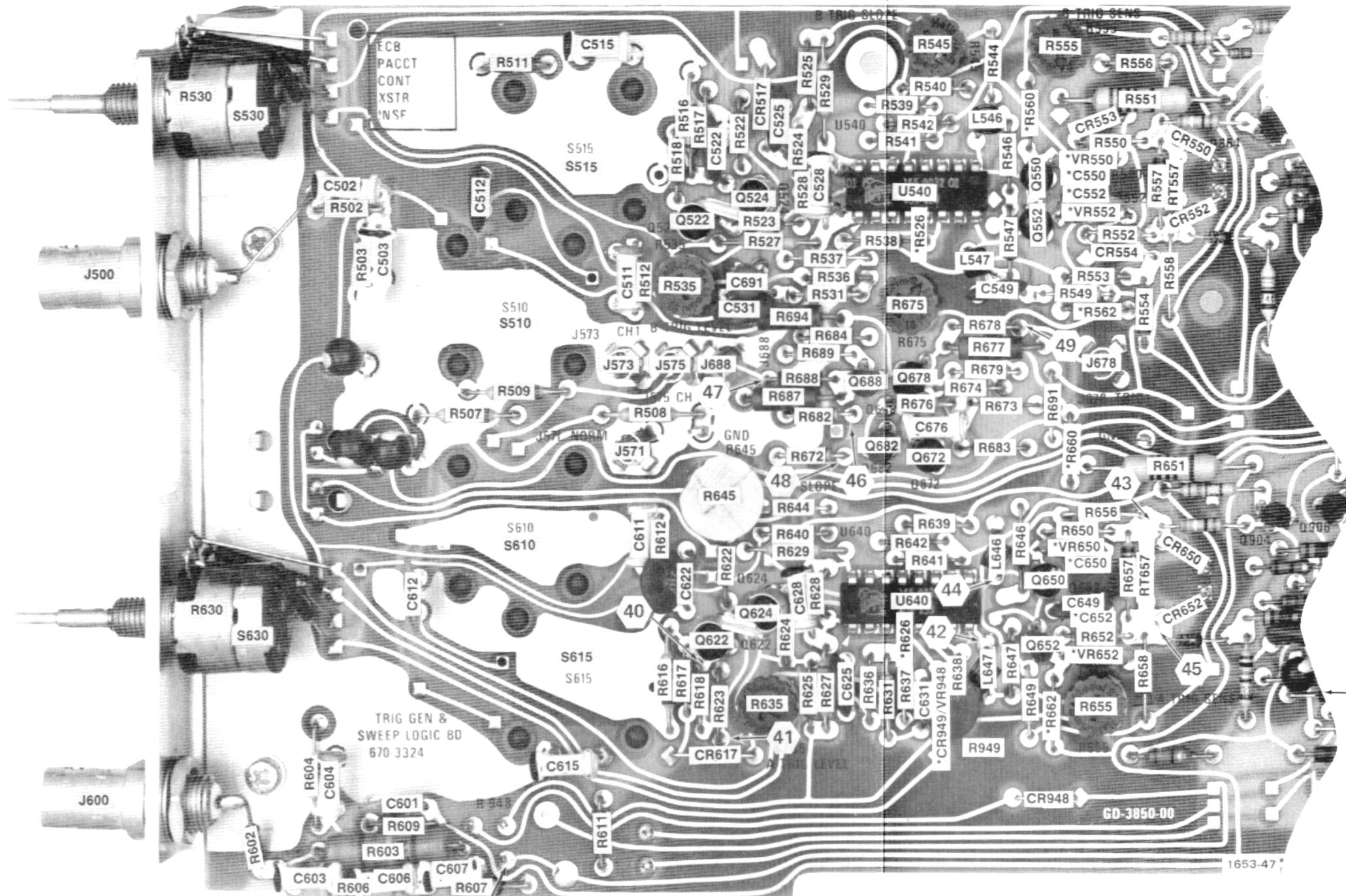
(A) Partial A5 Trigger Generator and Sweep Logic circuit board.
