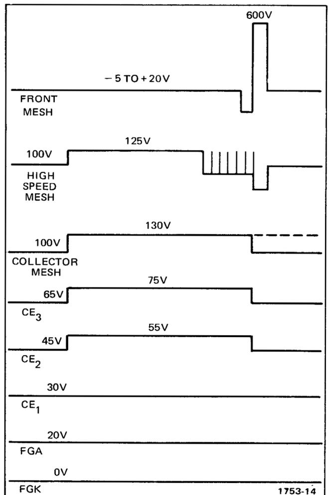
Fig. 3-14. Multi-Fast Mode—CRT Storage Element Voltage Levels.
