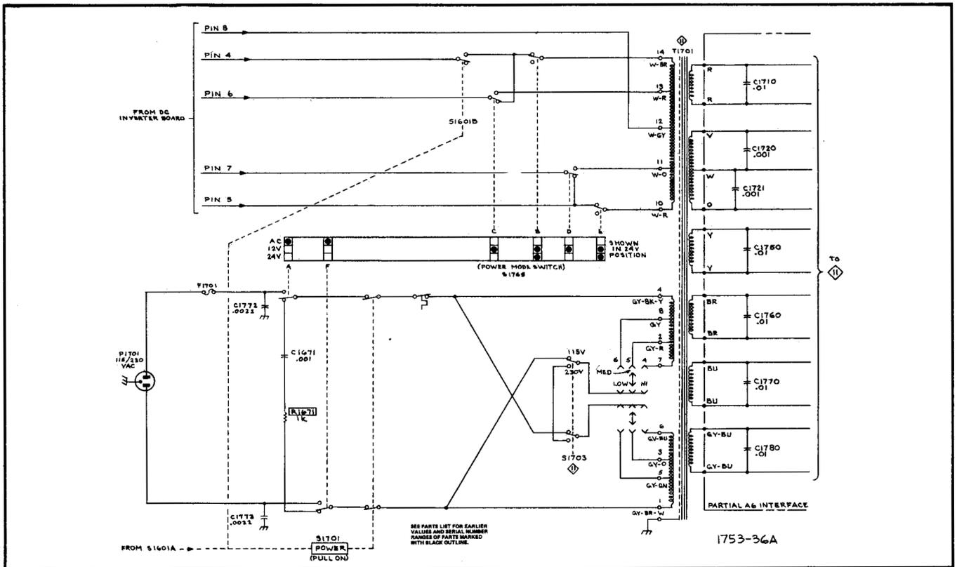
Fig. Option 7-7. 464 Option 7 primary winding.
