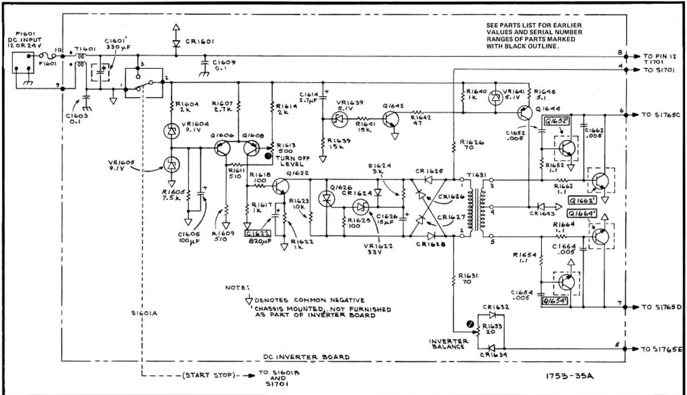
Fig. Option 7-5. 464 Option 7 dc inverter.
