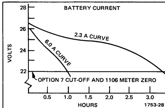
Fig. Option 7-2. Typical battery pack discharge curves.
