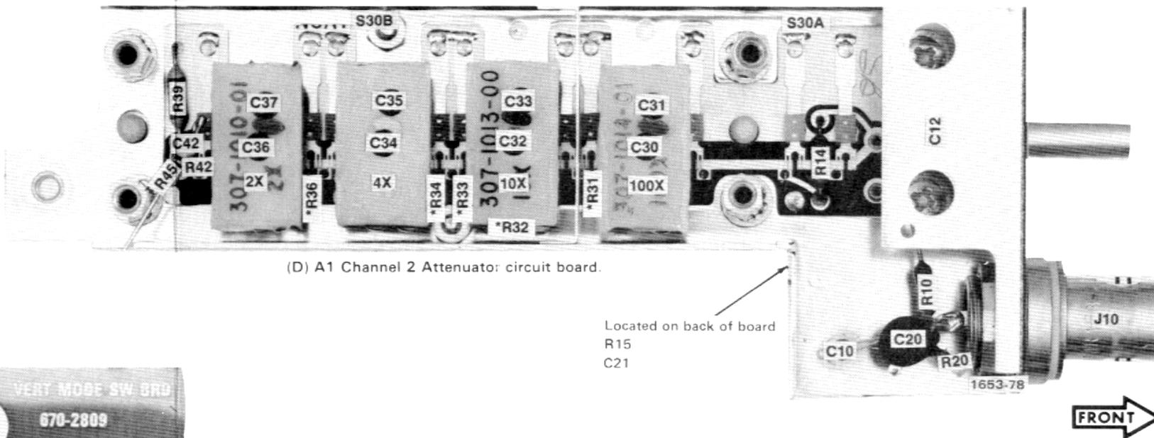
(D) A1 Channel 2 Attenuator circuit board.
