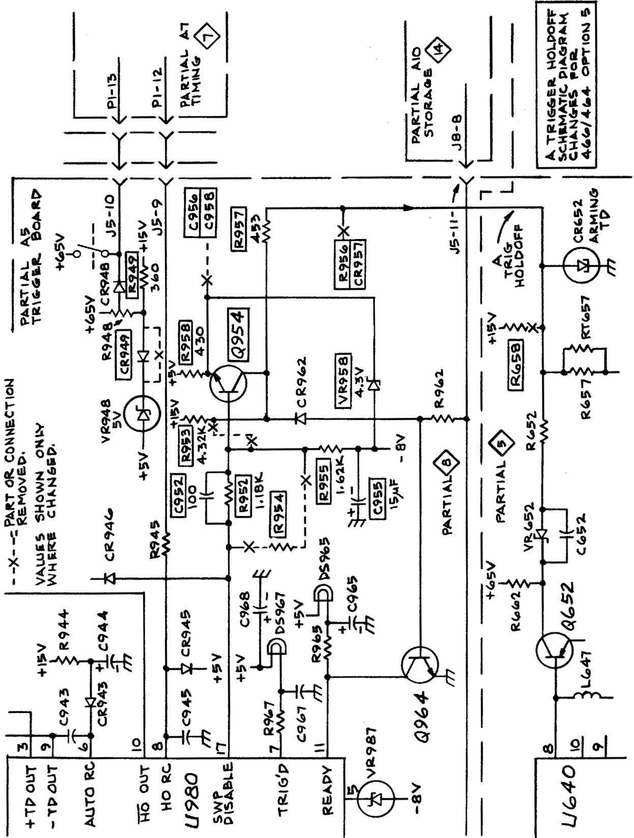
Fig. Option 5-7. Option 5 Trigger Holdoff circuit changes.
