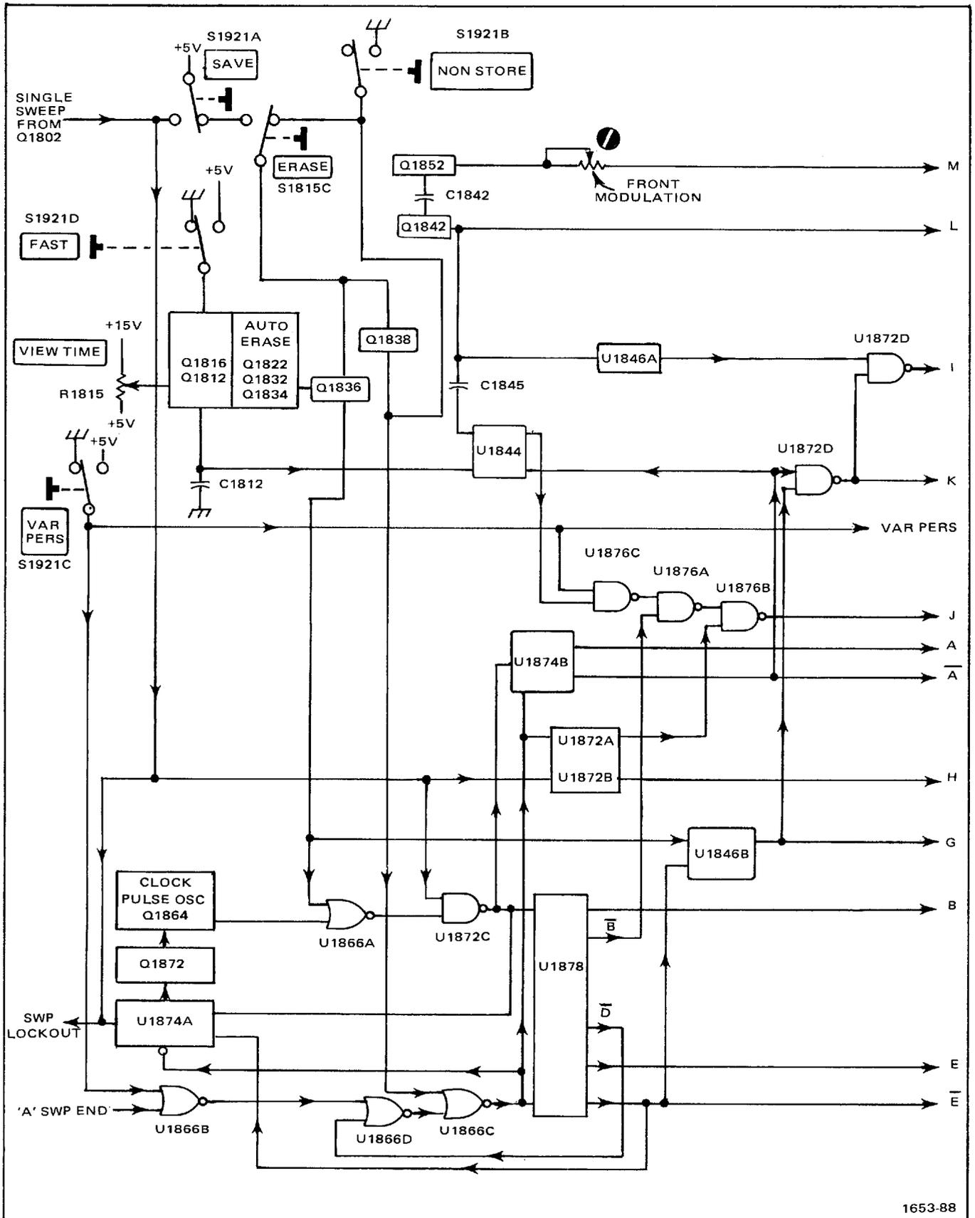
Fig. 3-9. Erase and Timing Circuit Detailed Block Diagram.
