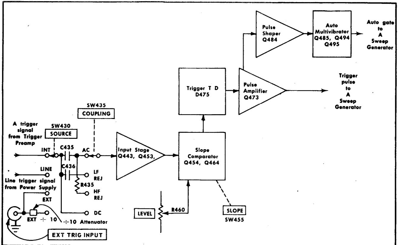
Fig. 3-8. A Trigger Generator detailed block diagram.
