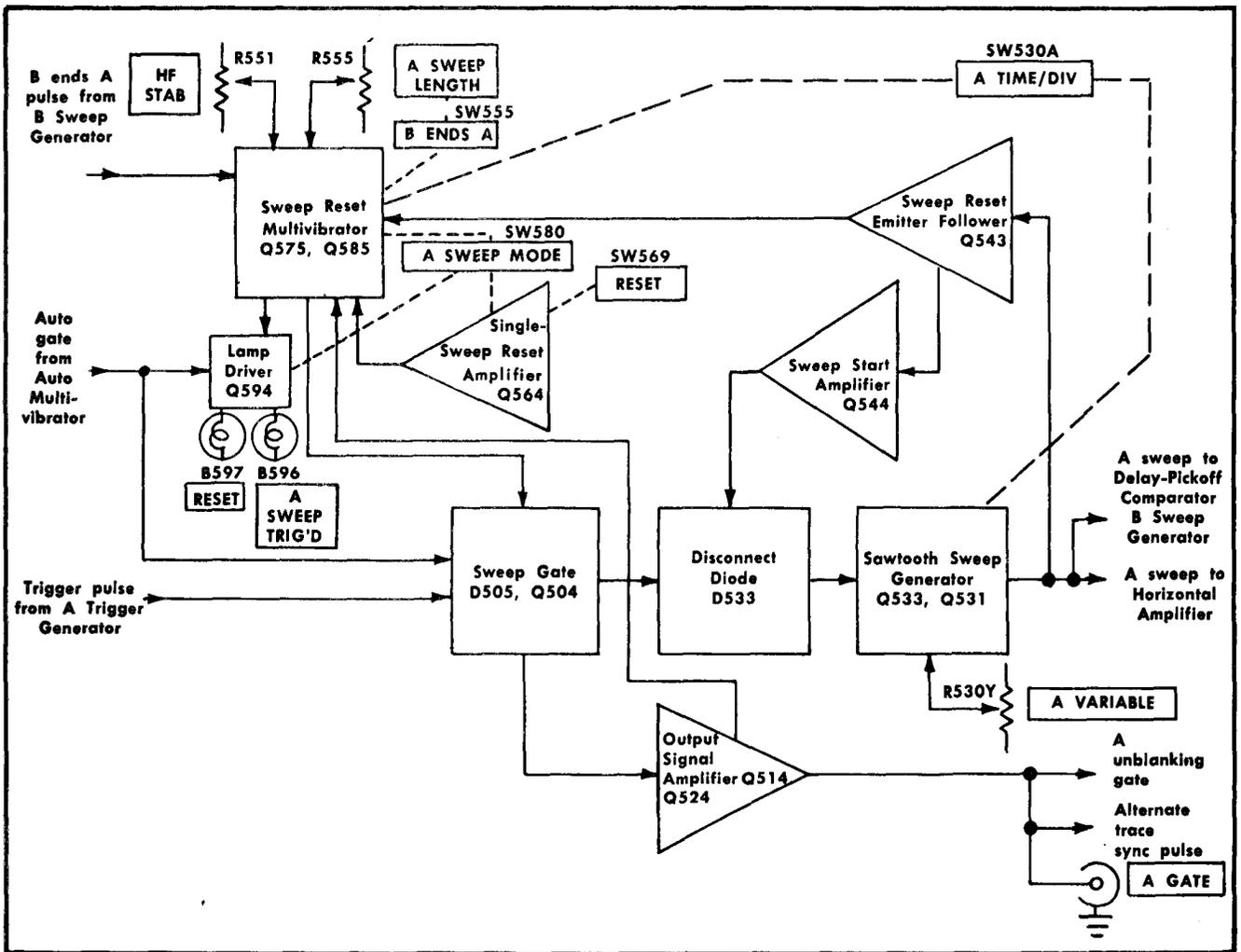
Fig. 3-11. A Sweep Generator detailed block diagram.
