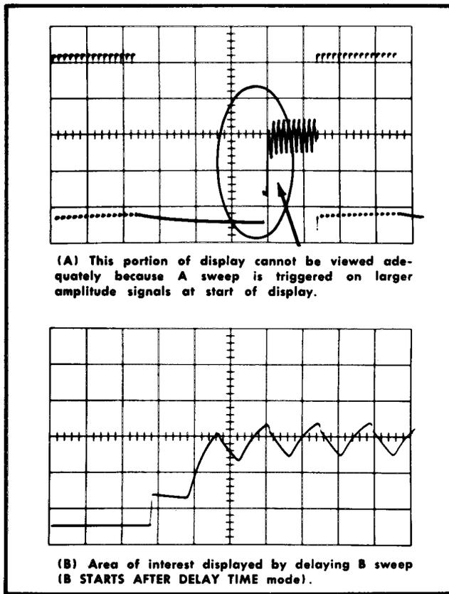
Fig. 2-22. Displaying a complex signal using delayed sweep.
