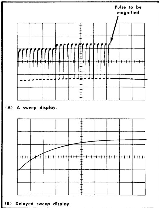
Fig. 2-21. Using delayed sweep for sweep magnification.
