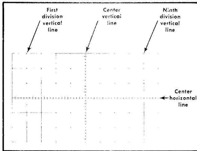
Fig. 2-6. Definition of measurement lines on Type 453 graticule.
