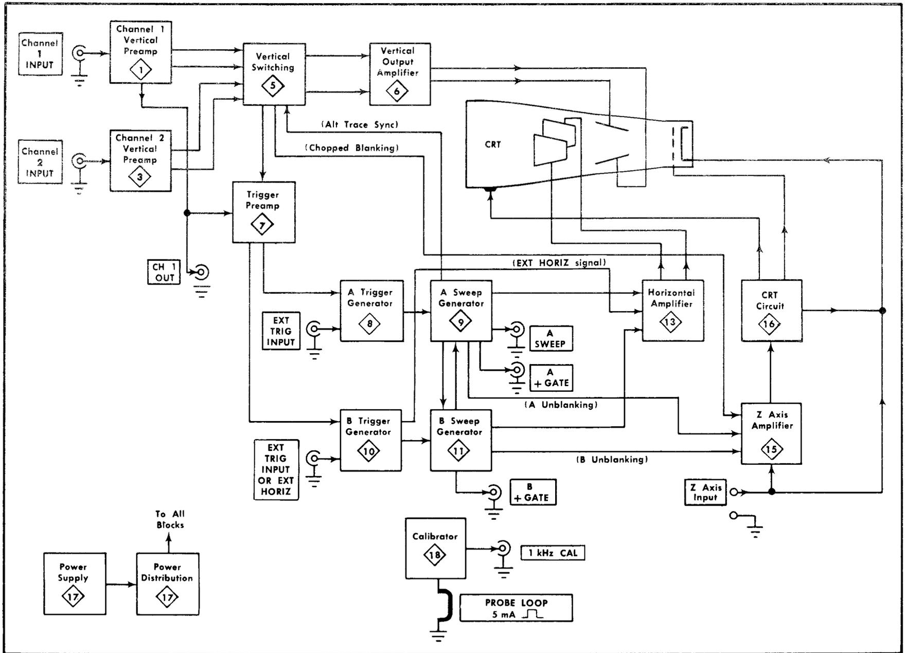
Fig. 3-1. Basic block diagram of the Type 453.
