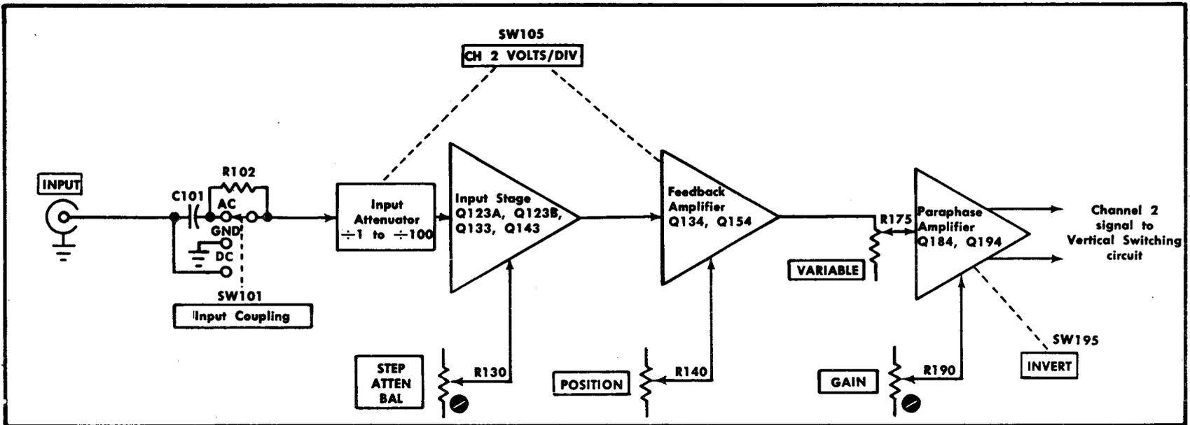
Fig. 3-3. Channel 2 Vertical Preamp detailed block diagram.
