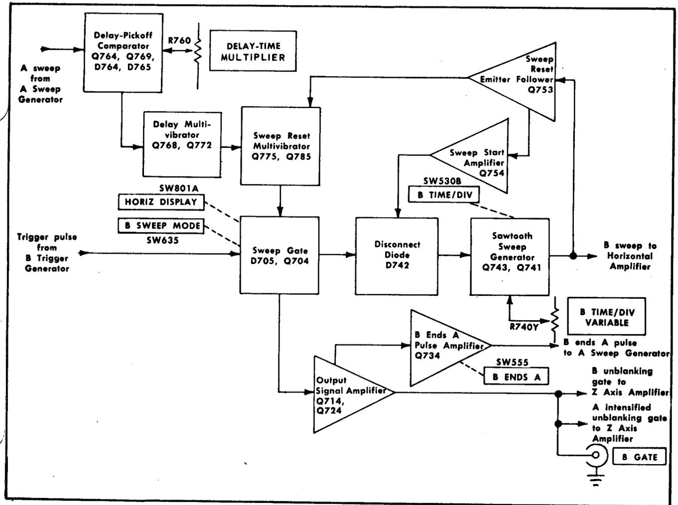
Fig. 3-13. B Sweep Generator detailed block diagram.
