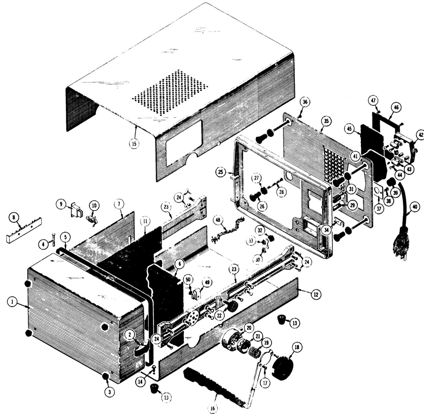
FIG. FO-8 R453 MECHANICAL PARTS
