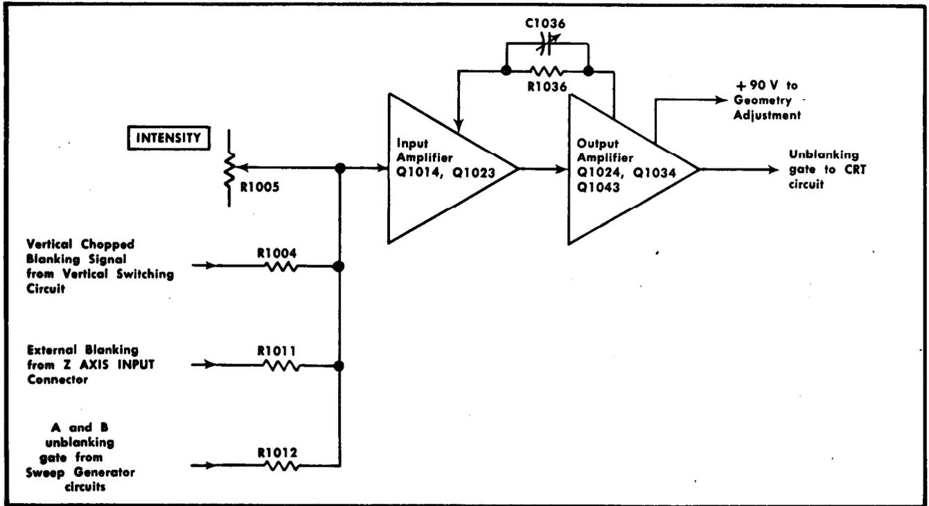
Fig. 3-15. Z Axis Amplifier detailed block diagram.
