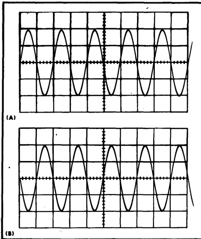
Fig. 6-36. Typical CRT display when checking slope switch operation. (A) SLOPE switch set to +, (B) SLOPE switch set to -.
