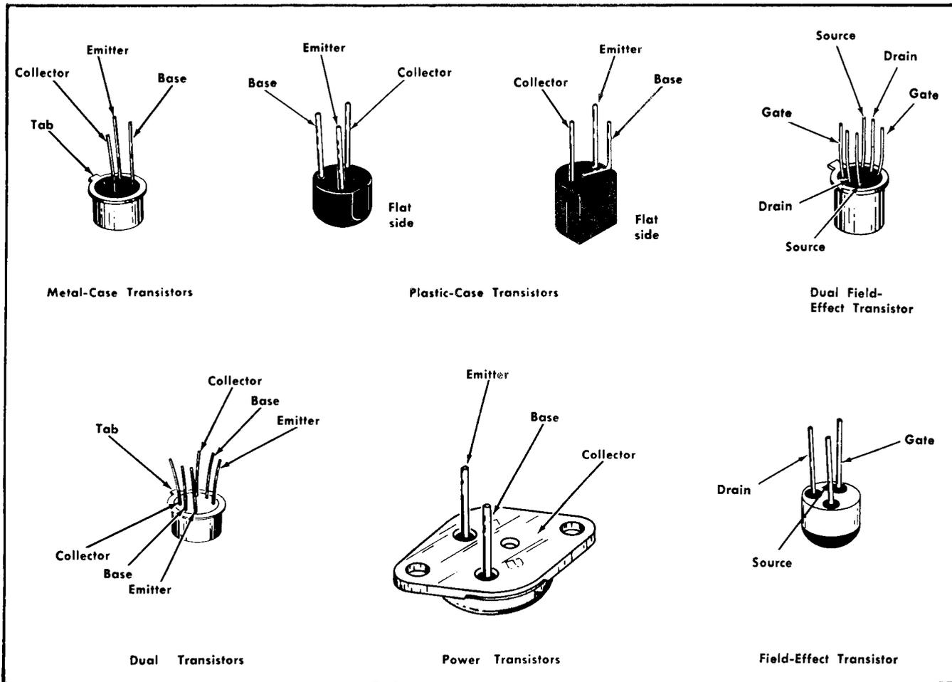
Fig. 4-2. Electrode configuration for semiconductors in this instrument.
