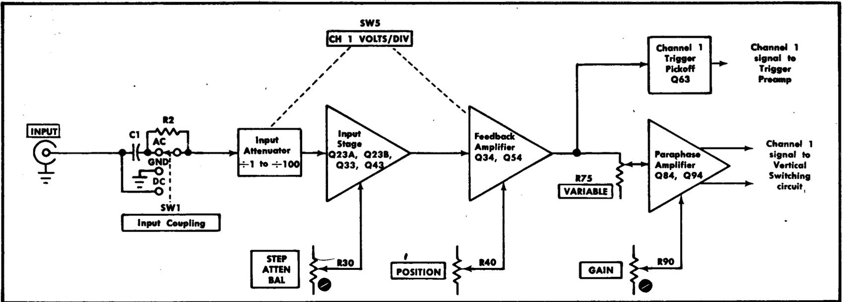
Fig. 3-2. Channel 1 Vertical Preamp detailed block diagram.
