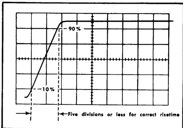
Fig. 6-58. Typical CRT display when checking Calibrator risetime.
