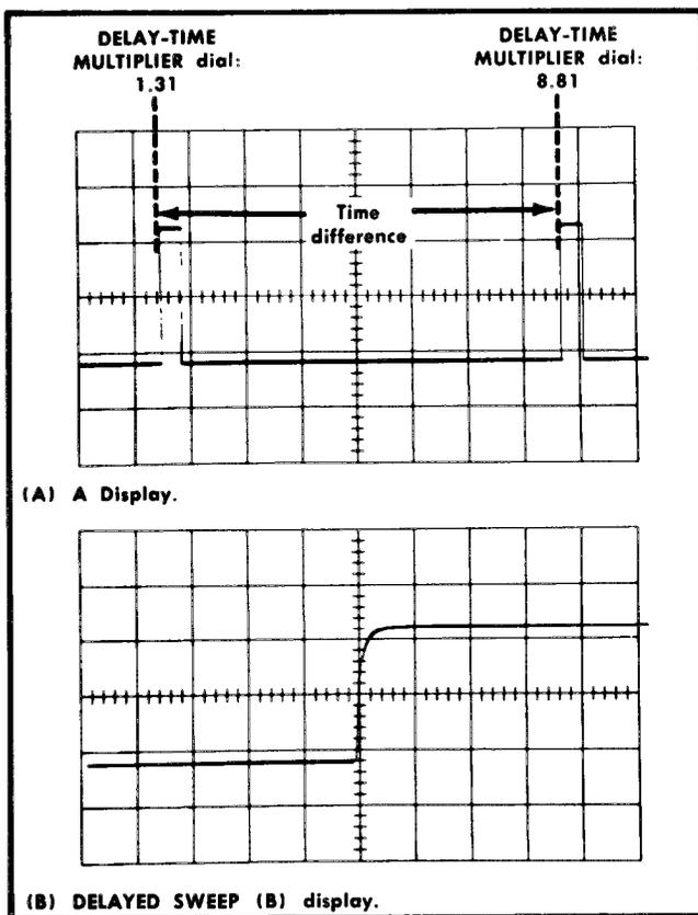
Fig. 2-20. Measuring time difference using delayed sweep.
