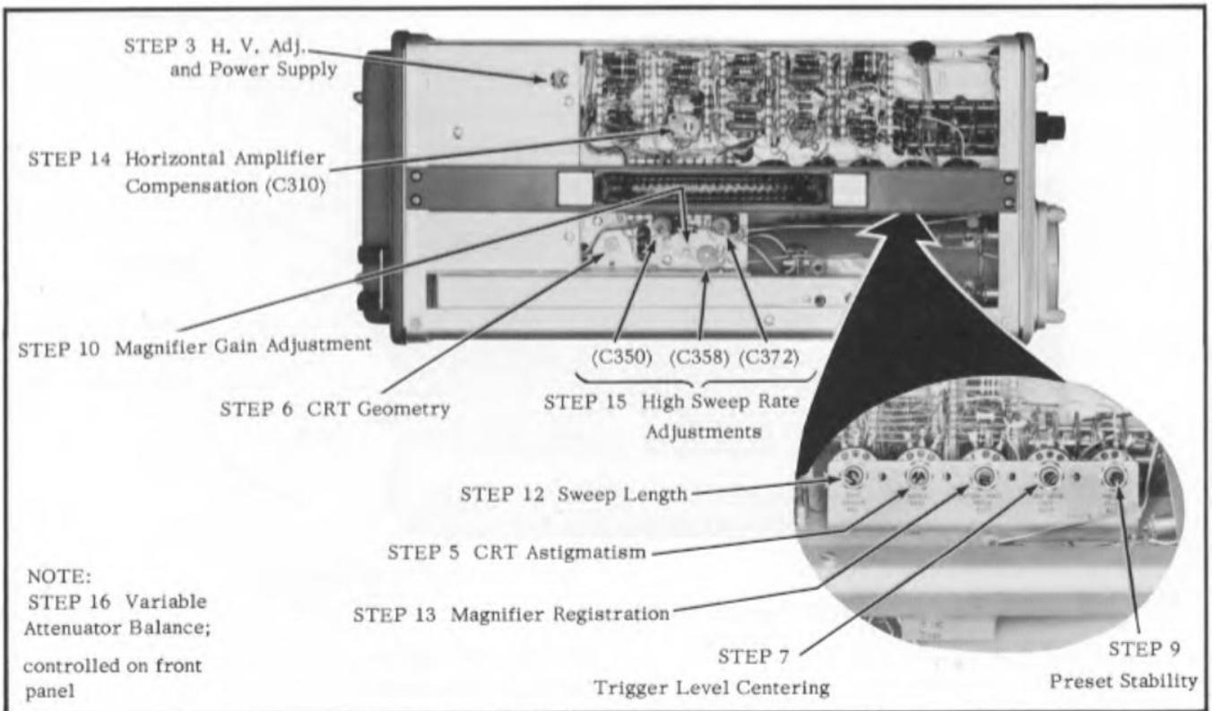
Fig. 5-13. Top View of the Type 316.
