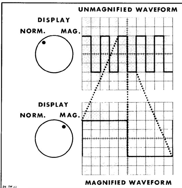
Fig. 2-7. Effects of the Sweep MAGNIFIER control.
