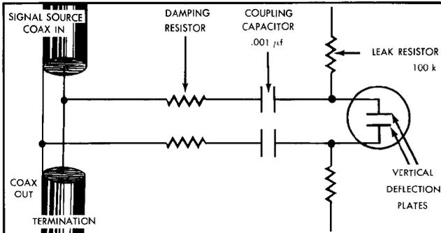
Fig. 2-8. Connecting to the crt deflection plates by AC coupling.
