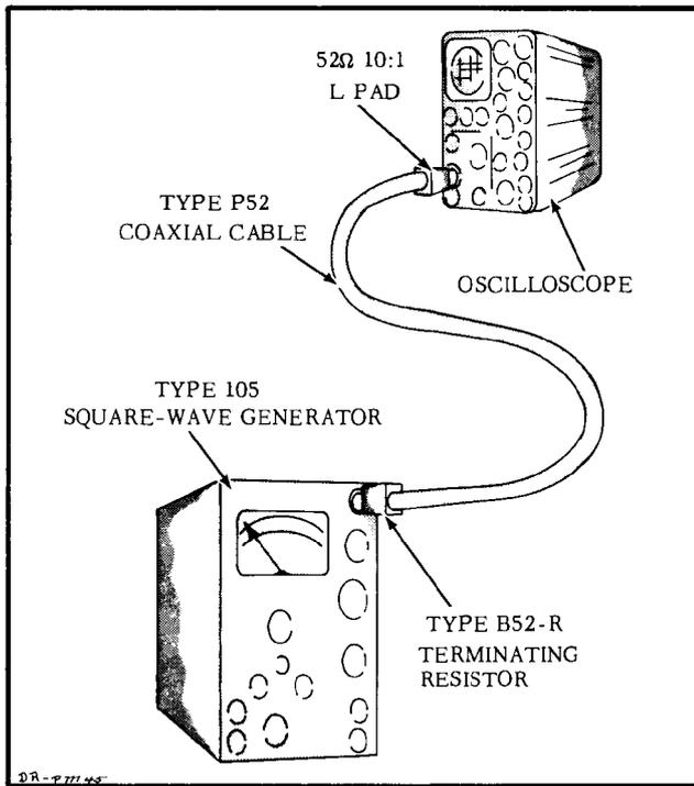
Fig. 5-5. Connecting the Type 105 Square-wave Generator to the oscilloscope.
