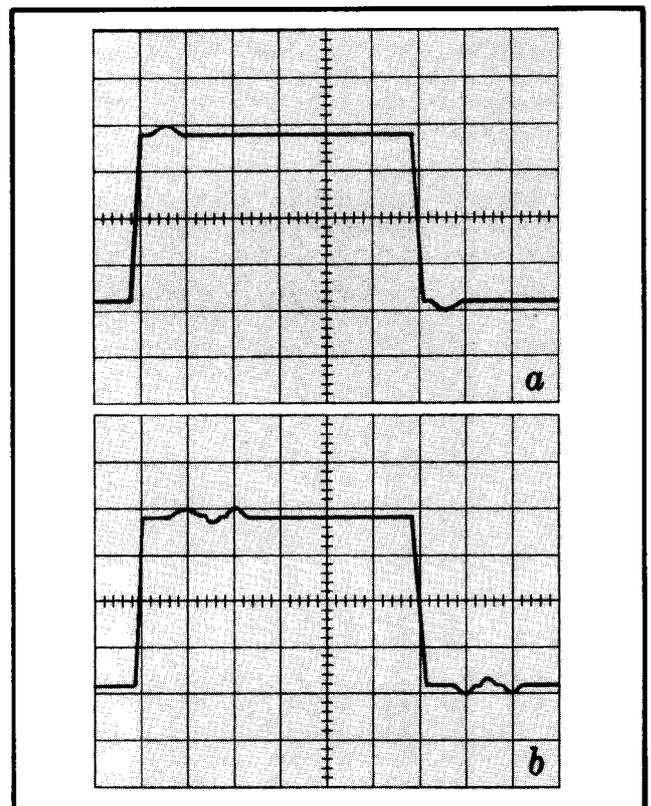
Fig. 5-9. Two types of "bumps" caused by delay-line misadjustment.
