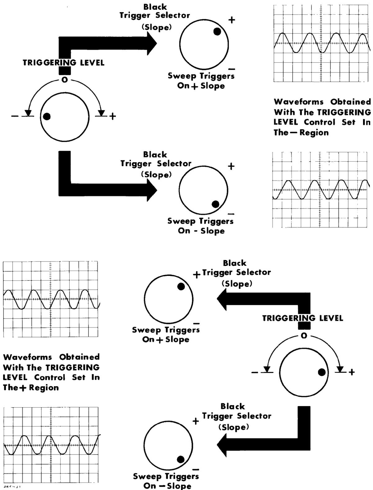
Fig. 2-5. Effects on the oscilloscope display produced by + and - settings of the TRIGGERING LEVEL control. When the TRIGGERING LEVEL control is set in the + region, the sweep is triggered on the upper portion of the input waveform; when it is set in the - region, the sweep is triggered on the lower portion of the input waveform. The TRIGGER SLOPE control determines whether the sweep is triggered on the rising portion or the falling portion of the input waveform.
