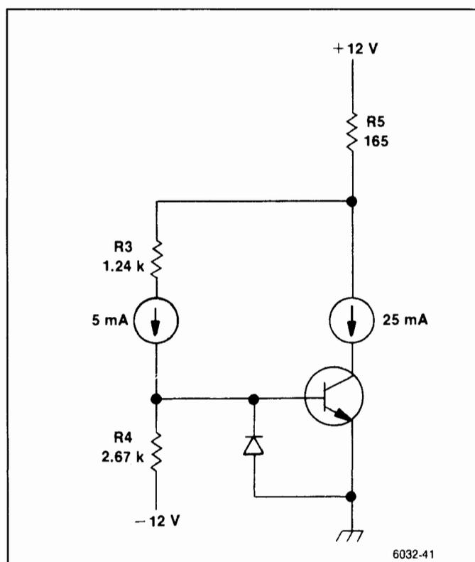
Figure 7-5. Equivalent dc circuit of an 829 MHz amplifier.
