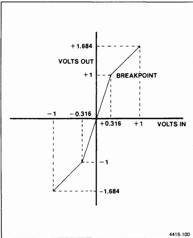
Figure 7-9. Log amplifier gain curve showing break points.
