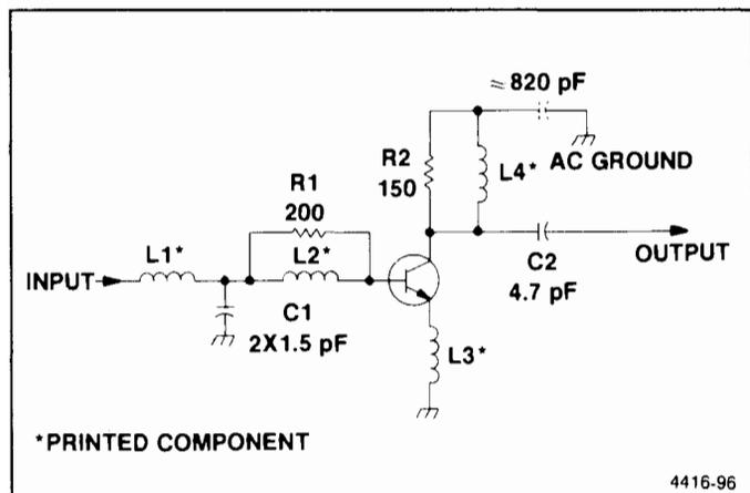
Figure 7-4. Equivalent ac circuit of an 829 MHz amplifier.
