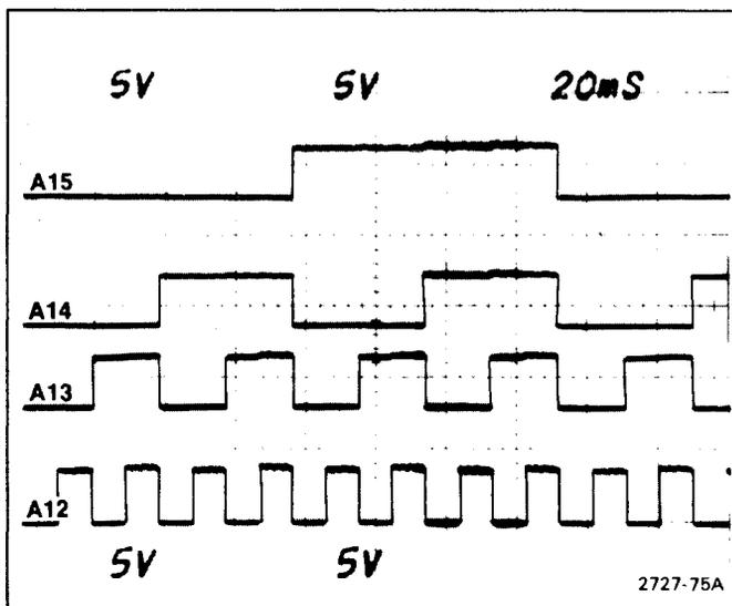
Figure 6-27. A15 through A12 in microcomputer test mode.
