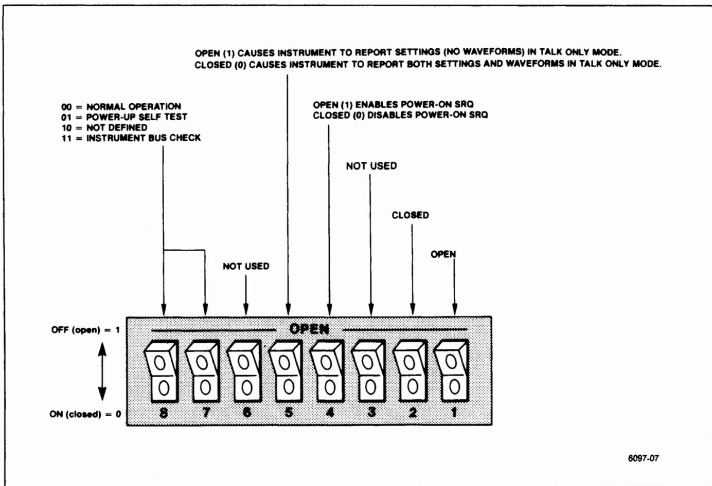
Figure 7-33. Options switch bank on the Memory board.
