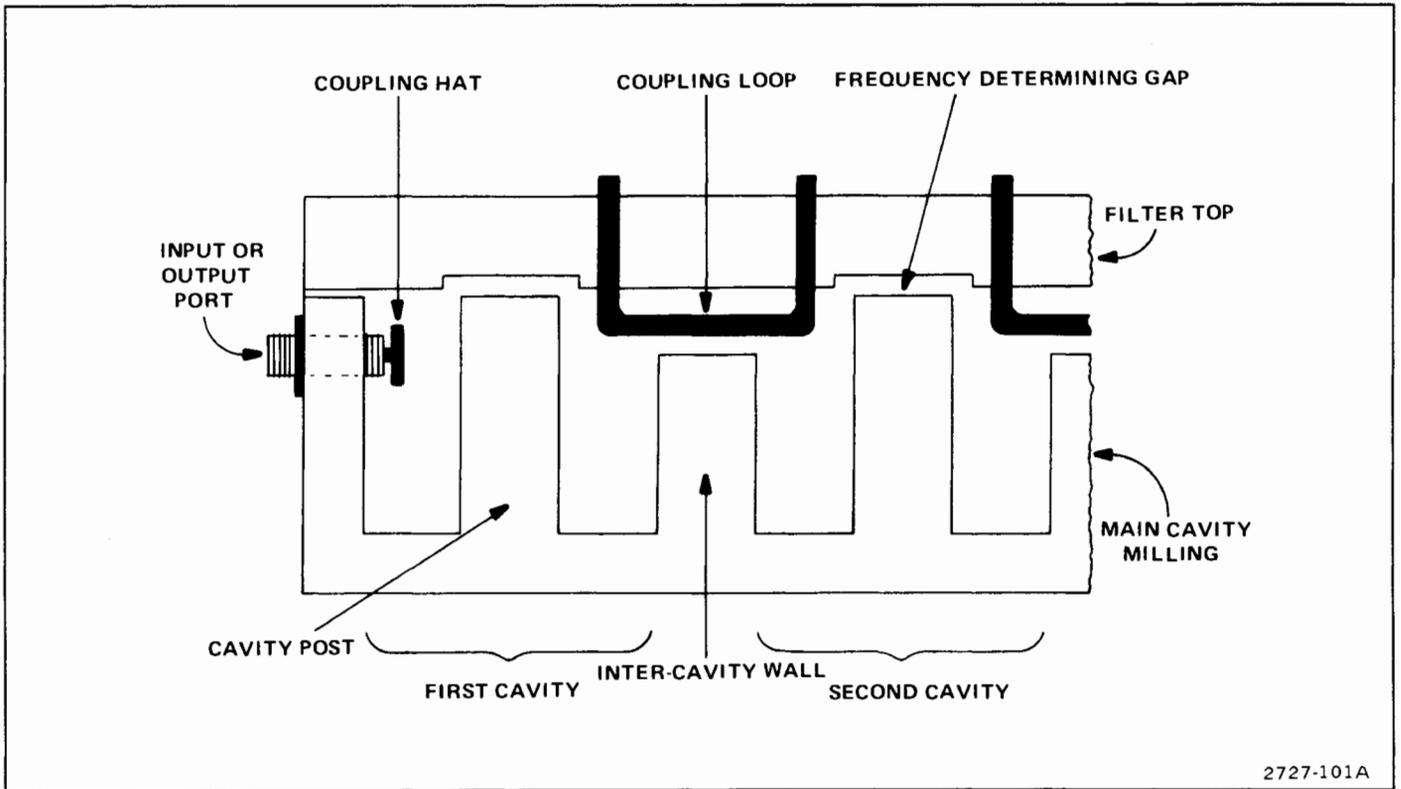
Figure 7-1. Cross section of a four-cavity filter.
