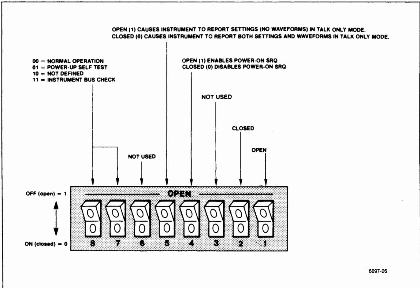
Figure 6-26. Options switch on the Memory board.
