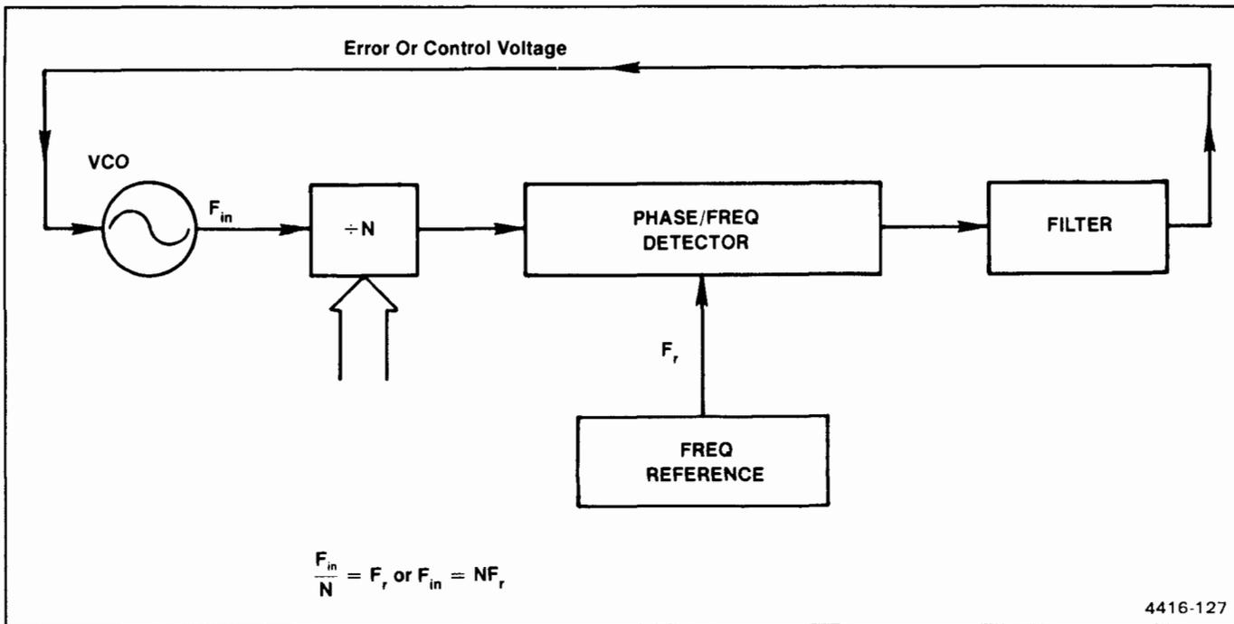
Figure 7-28. Block diagram of a basic synthesizer.
