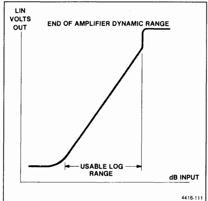
Figure 7-10. Curve showing end-of-range for a log amplifier.
