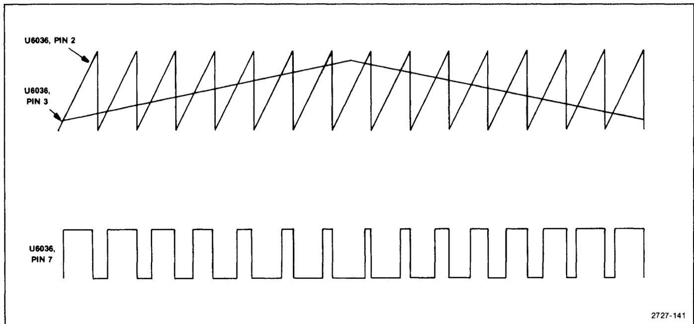
Figure 7-34. Primary regulator input and output waveforms.
