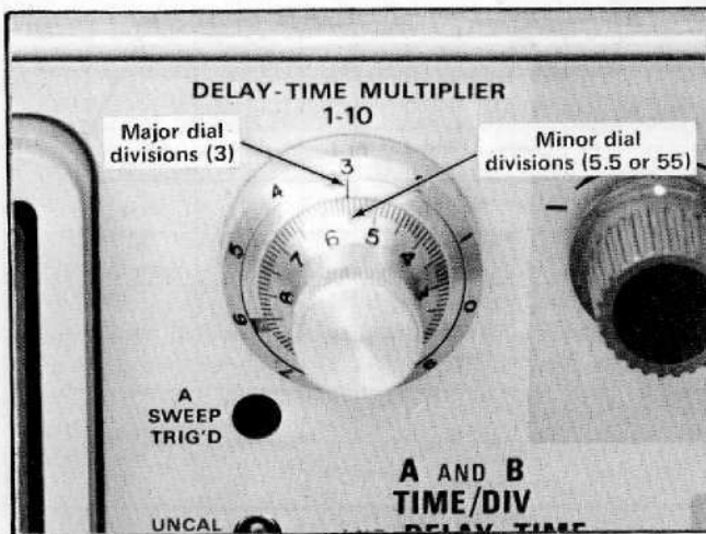
Fig. 2-16. DELAY-TIME MULTIPLIER dial. Reading shown: 3.55.
