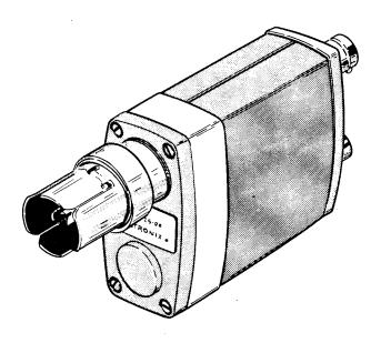
The 067-0625-00 Peak-To-Peak Detector is designed to measure the output voltage flatness of 50 OHM, constant-amplitude signal generators. The Detector has a frequency range of 50 Hz to 500 MHz and requires a 1.2V p-p input. Higher input voltages can be measured by attaching the appropriate attenuator.
