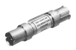
The Tektronix Type 067-0595-00 Calibration Fixture is a 200 MHz Notch Filter designed for use with Type 067-0594-00 Harmonic Generator. These calibration fixtures, together with a time-mark generator provide frequency markers suitable for calibrating microwave spectrum analyzers.
