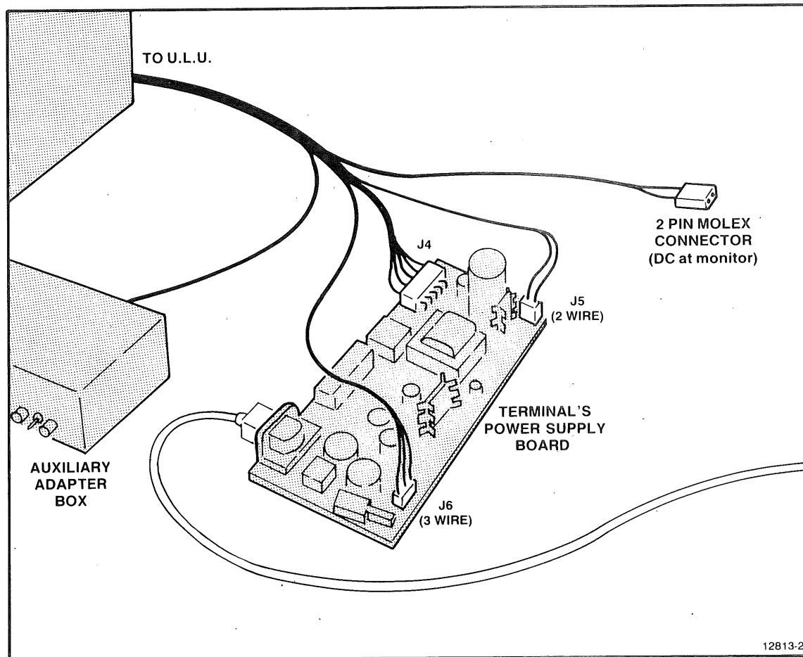
Figure 3-2. Connecting the Terminal to the Universal Load Unit and Auxiliary Box.
