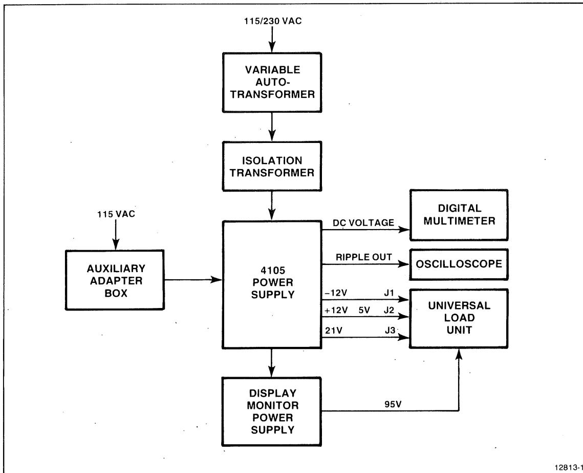
Figure 3-1. Performance Check Set Up.
