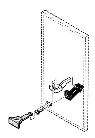
FIG. 1 PLUG-IN LATCH Latch assembly detail
