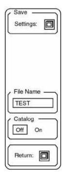
**Save Settings** Pressing this key will save the current analyzer settings to the file specified in the File Name field.
