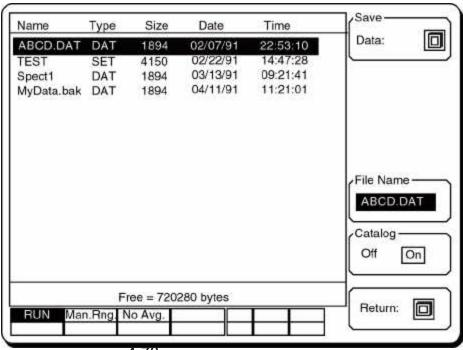
The first file will be highlighted and the file name will appear in the File Name field. Activating the cursor by pressing the [MARKER] key allows the knob to scroll through the directory. The highlighted file name will be copied into the File Name field. If the Save Data key is now pressed, the data will be saved under an existing file name and the previous version of that file will be lost. To create a new file name, use the File Name key.
