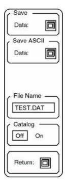
The Save Data submenu is used to save the active trace data and the associated limit and data tables. The graph parameters, frequency span, measurement, display, units and window are all saved with the data.
