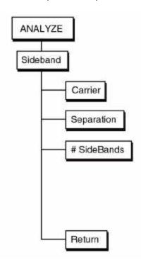
Sidebands are identified according to the formula Sideband n = Carrier ± n•Separation where n varies from 1 to the # of sidebands.
