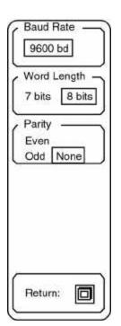
**Baud Rate** The Baud Rate key allows the knob to adjust the RS232 baud rate. The baud rate can be set to any standard value
