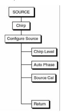
The Chirp source provides an equal amplitude sine wave at each bin of the measurement span. The phases of each sine wave are arranged so that they do not add in phase and the output does not peak. The chirp is EXACTLY periodic over a time record and requires no window. Because of cancellation, the amplitude of each sine wave is NOT constant over the time record. Windowing the time record actually removes necessary spectral information. **USE THE UNIFORM WINDOW WITH THE CHIRP SOURCE.**
