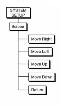
The screen position is stored in non-volatile memory and is retained when the power is turned off. To restore the screen to the default position, power the unit on with the [<-} (backspace) key pressed.
