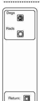
When Phase is being displayed on the active trace, the Units menu appears as shown to the left. Phase values are always between -180 and +180 degrees. The analyzer does not "unwrap" phase.
