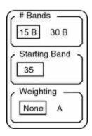
To choose the number of bands displayed, the starting band and the weighting function, use the FREQ menu. The FREQ menu will display the band selection menu shown at the right whenever octave analysis is on.
