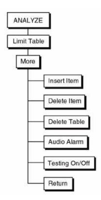
Insert Item This function inserts a new line before the highlighted line. The new line
