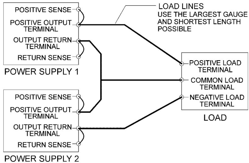
**Figure 4-25 Split Supply Operation of Multiple Supplies (Positive-Negative Supply)**
