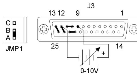
**Figure 4-5 Programming Output Voltage with a 0-10 Vdc Source**
