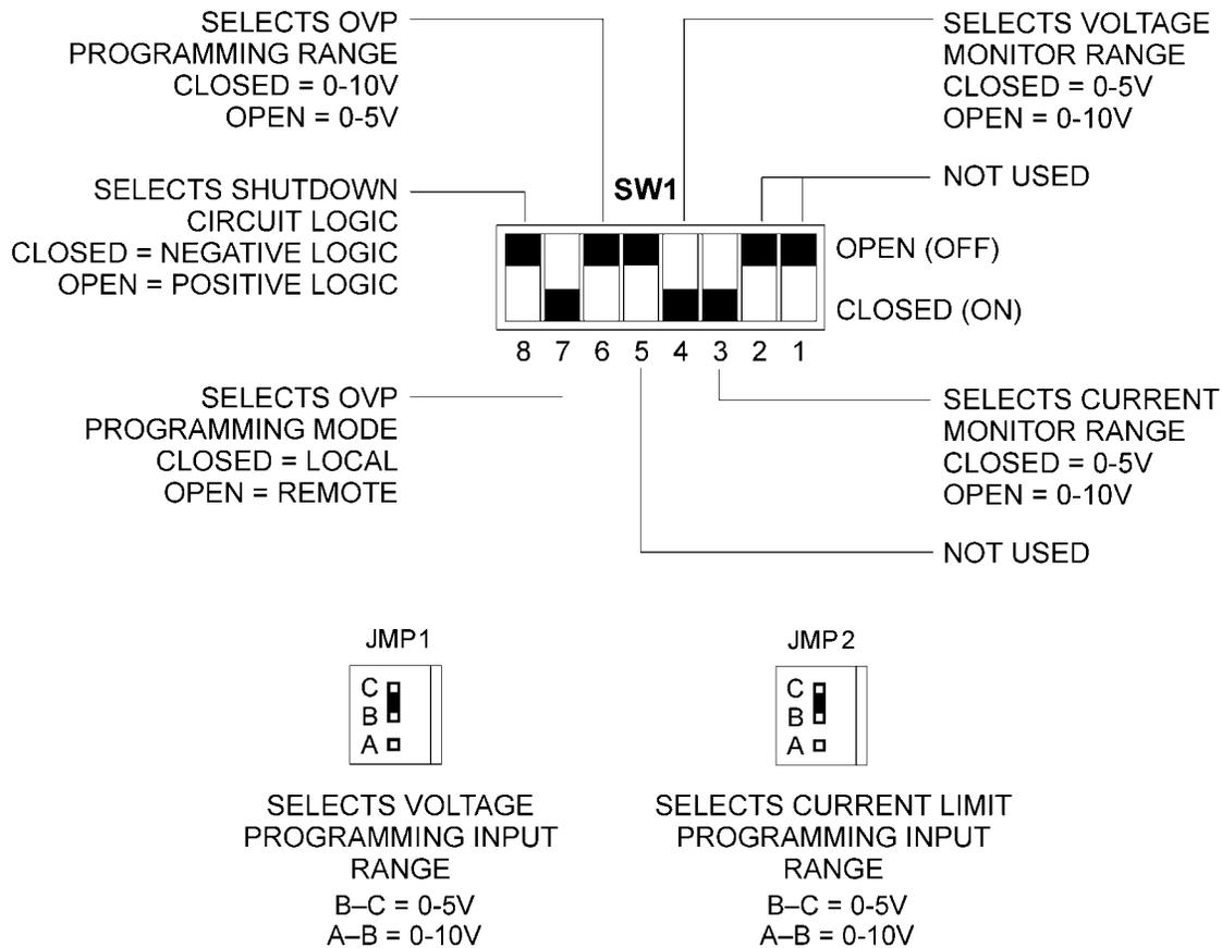
**Figure 4-2 Internal Jumpers and Switch (Default Settings Shown)**
