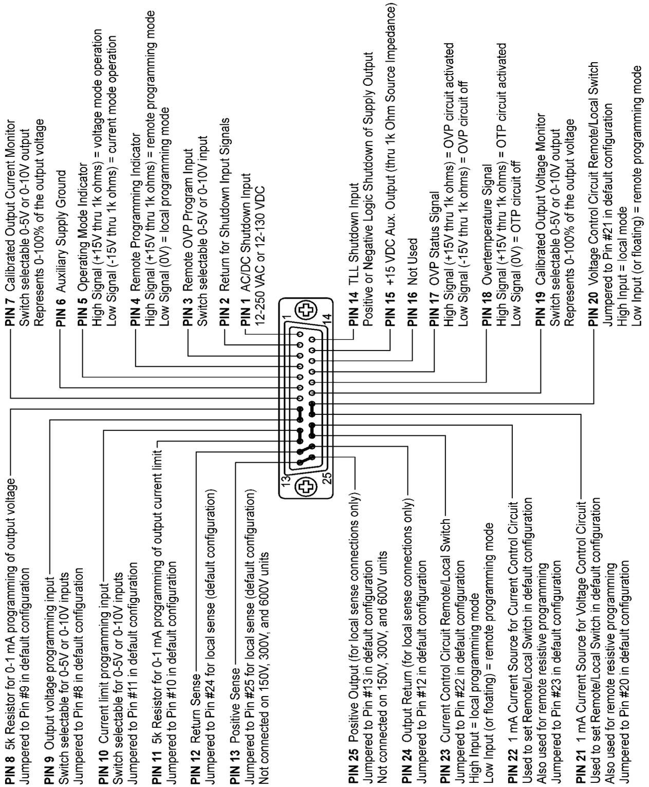
**Figure 4-1 Connector J3 Pin Descriptions
