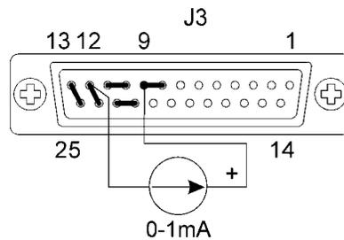
**Figure 4-6 Programming Output Voltage with a 0-1 mA Source**
