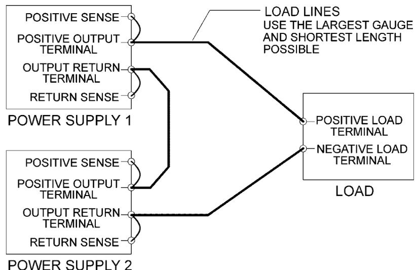
**Figure 4-22 Series Operation of Multiple Supplies**
