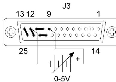
**Figure 4-4 Programming Output Voltage with a 0-5 Vdc Source**
