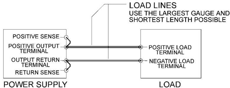
**Figure 2-9 Single Load with Local Sensing (Default)**
