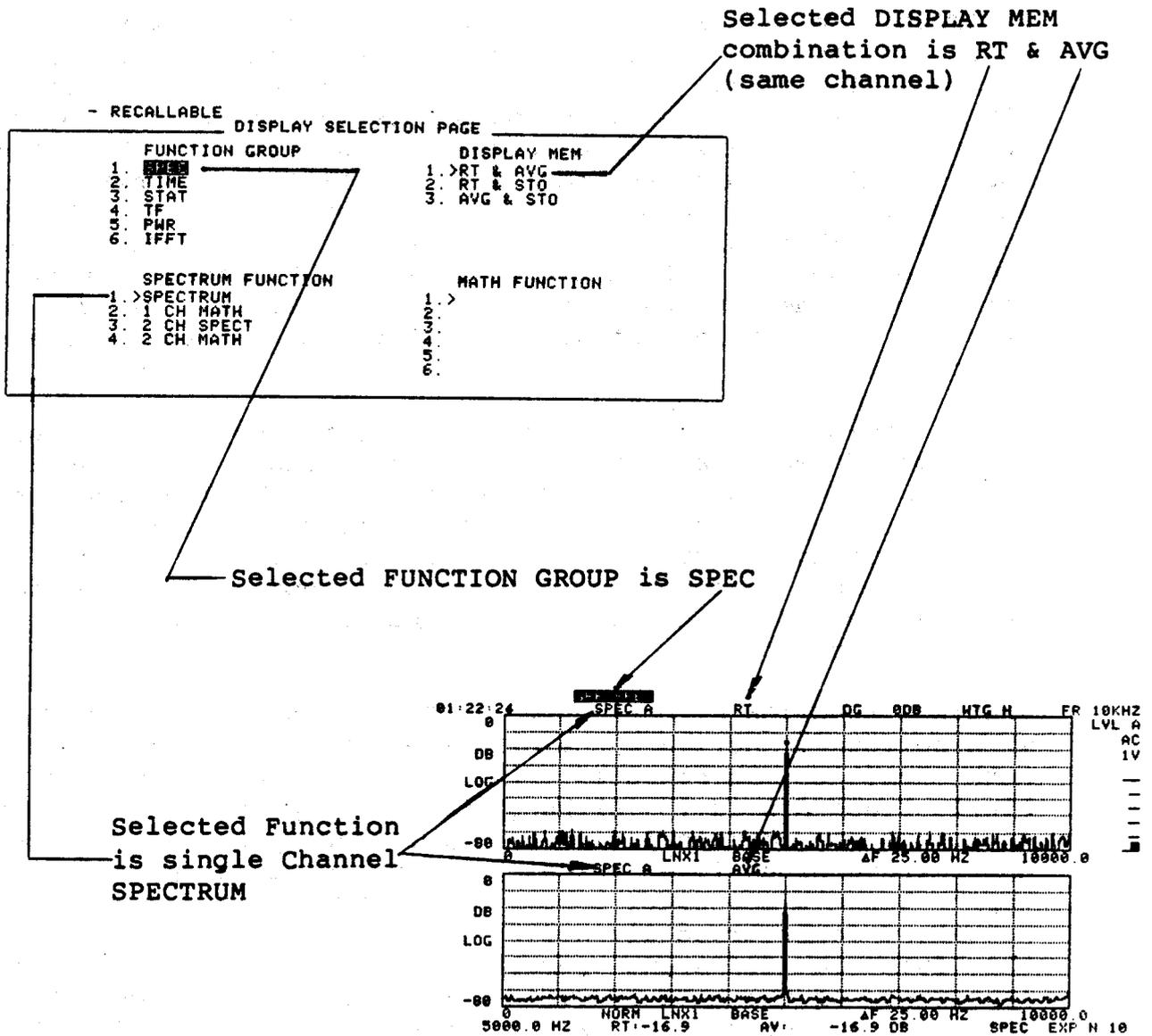
Figure 3-DISP-1. Operation of Setup Page 3 DISPLAY SELECTION PAGE
