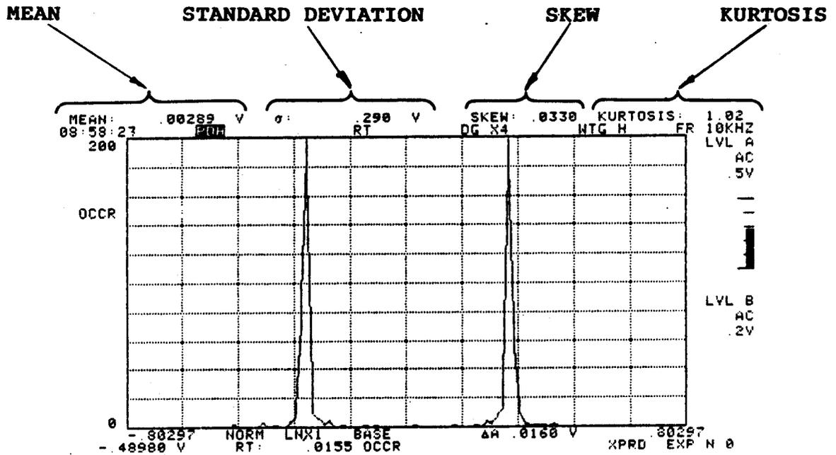
Figure 3-DSP/SEL-19. PDF Distribution of the Square Wave Shown Figure 3-DSP/SEL-18.
