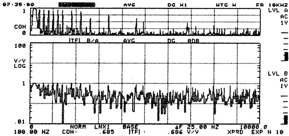
Figure 3-DSP/SEL-37. TRANSFER FUNCTION Selection 2, |TF| & COH
