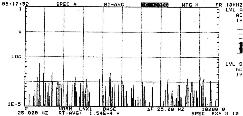
Figure 3-DSP/SEL-4. MATH FUNCTION Menu Selection 2, RT - AVG; i.e., Upper Trace, Real Time Spectrum Data Minus the Lower Trace Averaged Spectrum Data
