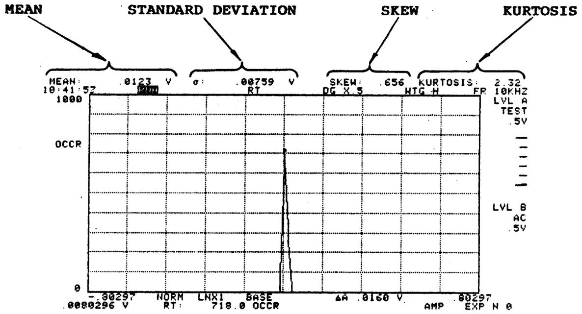
Figure 3-DSP/SEL-28. PDF Distribution of Random Noise Shown in Figure 3-DSP/SEL-27.
