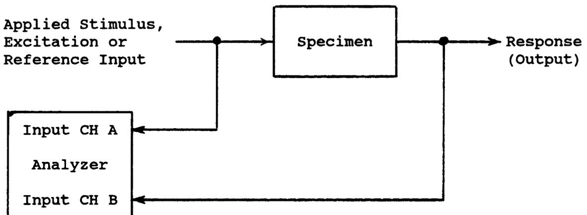
Figure 3-DSP/SEL-34. Basic Transfer Function Interconnect
