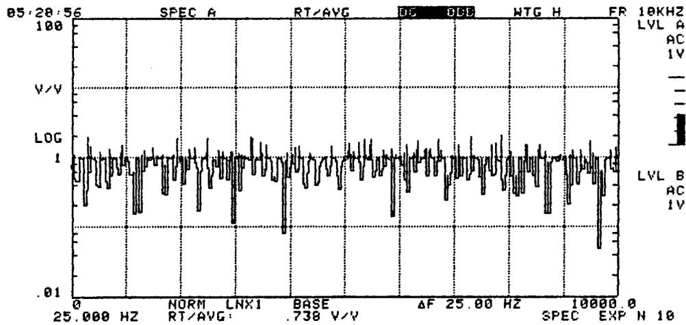
Figure 3-DSP/SEL-7. MATH FUNCTION Menu Selection 5, RT/AVG; i.e., Upper Trace, Real Time Spectrum Data Divided by the Lower Trace, Averaged Spectrum Data
