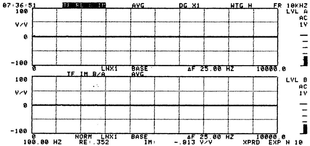
Figure 3-DSP/SEL-38. TRANSFER FUNCTION Menu Selection 3, TF RE & IM
