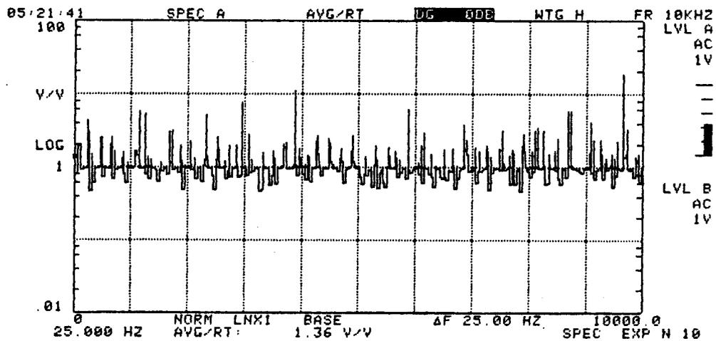
Figure 3-DSP/SEL-8. MATH FUNCTION Menu Selection 6, AVG/RT; i.e., Lower Trace, Averaged Spectrum Data Divided by the Upper Trace, Real Time Spectrum Data
