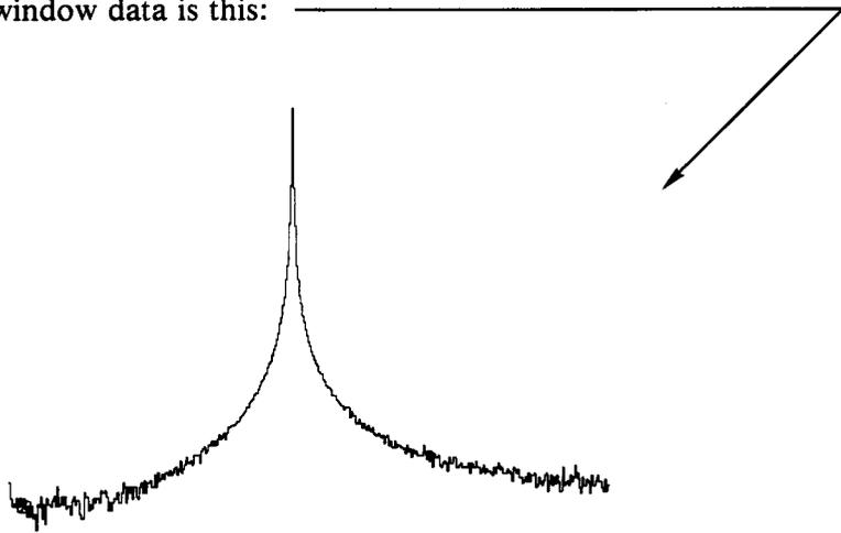
This phenomenon is called “flaring” or “skirting” and is frequently referred to as “Rectangular” weighting and actually entails no weighting at all (the data is FFT’d as is). Weighting cleans this up by making the “ends” of the time sample smoothly go to zero.
