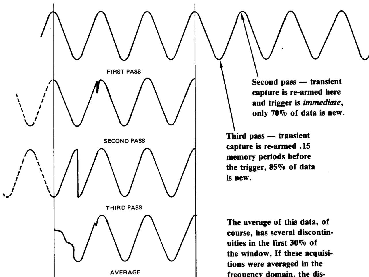
The average of this data, of course, has several discontinuities in the first 30% of the window, If these acquisitions were averaged in the frequency domain, the discontinuities in the second and third passes would show up as flaring of the spectrum.
