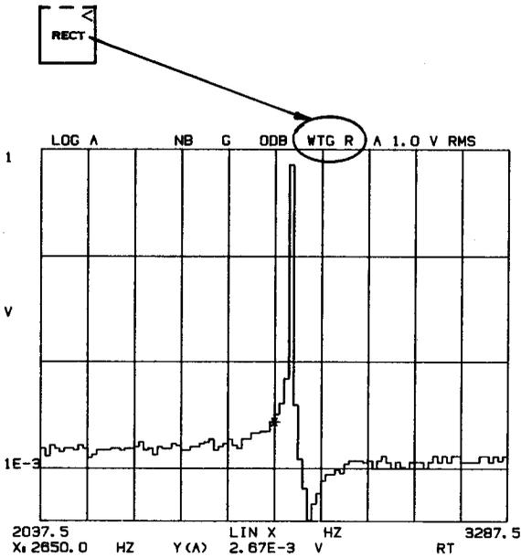
Figure 3-9. Examples of Hanning, Flat Top and Rectangular Weighting.
