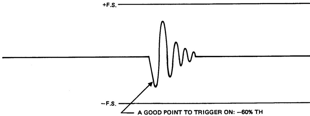
When this signal level is detected by Transient Capture circuitry, the input memory is placed in the HOLD mode.
