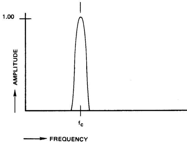
A digital spectrum analyzer carries the spectrum analysis concept even farther; it displays the output of 400 such *digital* filters, equally spaced, simultaneously. This is done with a high speed discrete Fourier Transform called the FFT. FFT analysis allows the rapid transformation of discrete time domain data into the frequency domain. The end result is 400 values representing the simultaneous output of 400 high Q filters.
