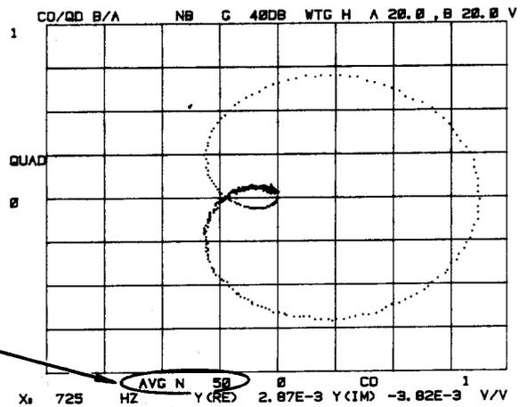
To select the number of ensembles to be averaged or averaging time, in seconds, press AVG N (ensemble averaging) or AVG T (averaging over a selected time interval) in the PARAMETERS group. The following annotation will appear in the upper right-hand corner of the display grid:
