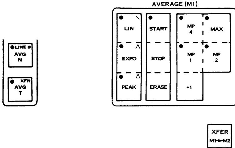
When the operator of the SD375 presses Average START he is, fundamentally, telling the analyzer “accumulate signal data in the averager memory” (M1). If the operator has enabled auto trigger (AUTO TRIG) or transient auto (TRANS AUTO), this accumulation is qualified by “when the designated signal level has occurred”. (AUTO TRIG and TRANS AUTO are covered in subsection 3.4.2.4.)
