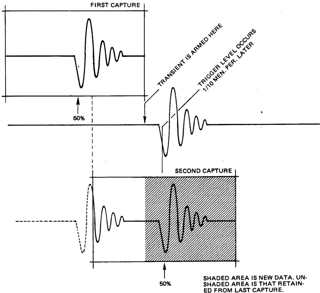
When you manually operate the transient capture feature you can bypass this corruption of the current transient by the previous transient, by simply re-arming the capture.
