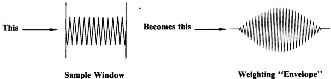
An effect of the different weighting functions (on the data) is the effective *shape* of the digital filters (they overlap) that yield the 400 point (line) display.
