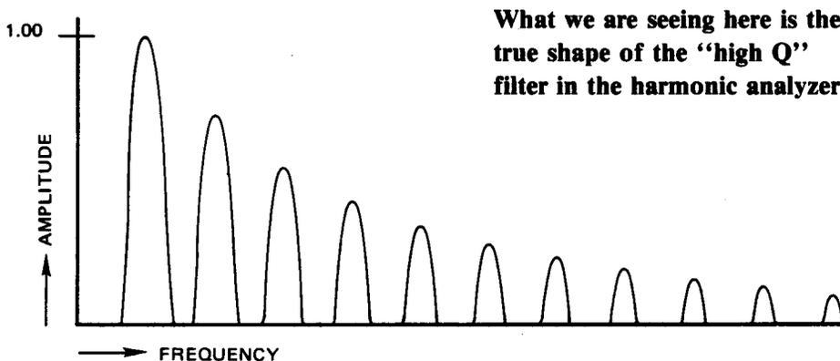
The harmonic plot of the previous sketch is the result of sweeping a filter of this shape over a stationary signal with more than one frequency component. If you were to leave the filter at some frequency and sweep the signal through that frequency, the filter response would be:
