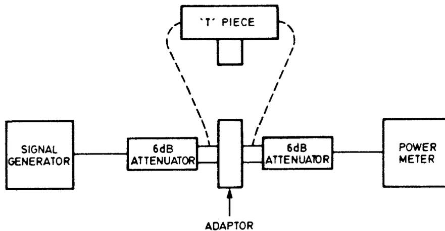
T Piece Insertion Loss Check Connections
