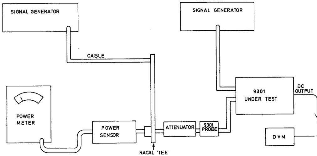
20dB and 40dB Attenuator Test Connections Fig.5.11
