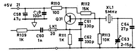
5MHz REFERENCE OSCILLATOR ON MAIN PCB. (EARLY MODELS)
