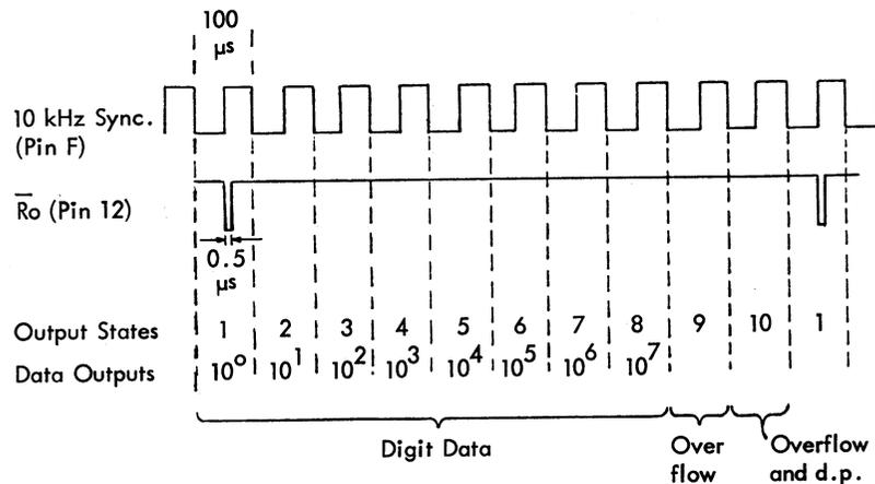
Fig. 2 Data Sequence Diagram
