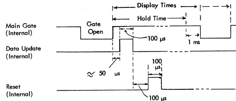
Fig. 3 Control Sequence Diagram
