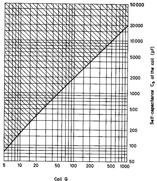
Fig. 4 Upper measurement-range limit for self-capacitances as a function of coil Q
