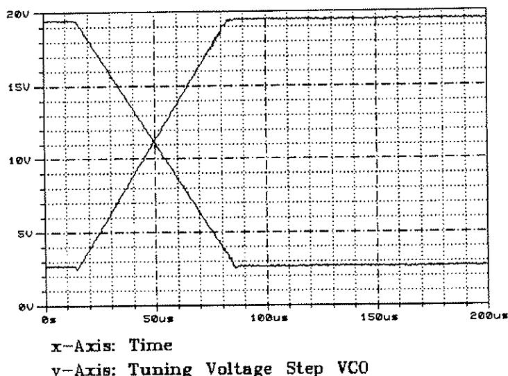
The voltage characteristic of both frequency changes (103 to 117MHz, 117 to 103MHz) is simultaneously shown in the oscilloscope. Since the board cover is not fitted, the level of the tuning voltage is slightly higher than the level in the adjusted state with cover fitted (103MHz/2V, 117MHz/18V).
