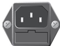
The AC supply connector comprises a standard, IEC low-temperature connector and contains a fuse holder for two miniature fuses. The fuse holder can be taken out with a screwdriver.
