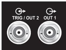
The BNC connector OUT1 outputs an analog signal with a voltage between 0V and 3.3 V. It can be used to output a voltage that is proportional to the measured value (e.g. for level regulation) or a digital signal for threshold monitoring.
