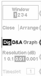
The digital display (**Dig**) displays measured values as a number with additional information next to the reading.
