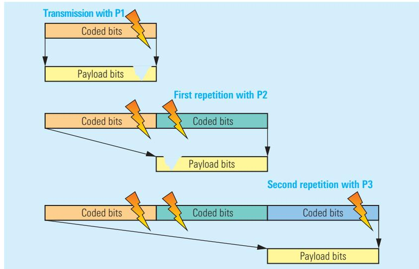
**FIG 2** With incremental redundancy, the incorrectly transmitted block is not repeated but the data is transmitted with the next puncturing scheme. Both blocks are then used for error correction. This increases the probability of correcting transmission errors. In the example, all three transmissions are flawed. By combining the three received data blocks, data can, however, be decoded without error.
