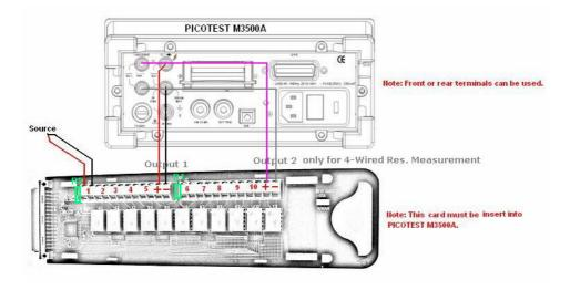
Note: The output 2 is only for 4-wired resistance measurement. Please refer to the above picture for more connection information. When you use 4-wired resistance measurement with scanner card, please note that the channel 1 is relative to the channel 6, channel 2 to channel 7 and so on.
