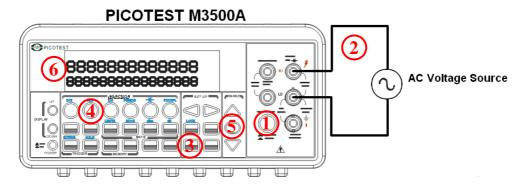
Input Impedence =  $1M\Omega$  in parallel with < 100pF (Warning: Maximum Input = 750V RMS, 1000V peak,  $8 \times 10^{'}$  V·Hz)
