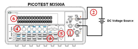
Input Resistance =  $10M\Omega$  on 1000V and 100V ranges; >  $10G\Omega$  on 10V, 1V and 100mV ranges.
