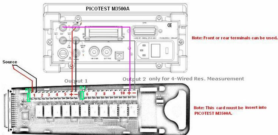
※ Note: The output 2 is only for 4-wired resistance measurement. Please refer to the above picture for more connection information. When you use 4-wired resistance measurement with scanner card, please note that the channel 1 is relative to the channel 6, channel 2 to channel 7 and so on.
