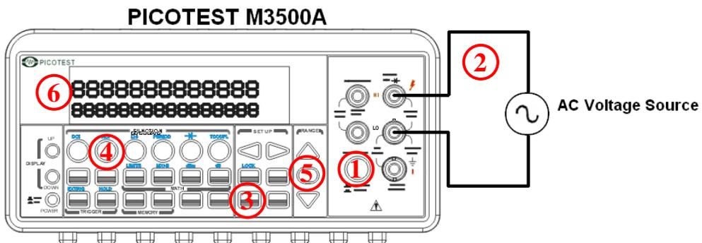
Input Impedance = 1MΩ in parallel with < 100pF
