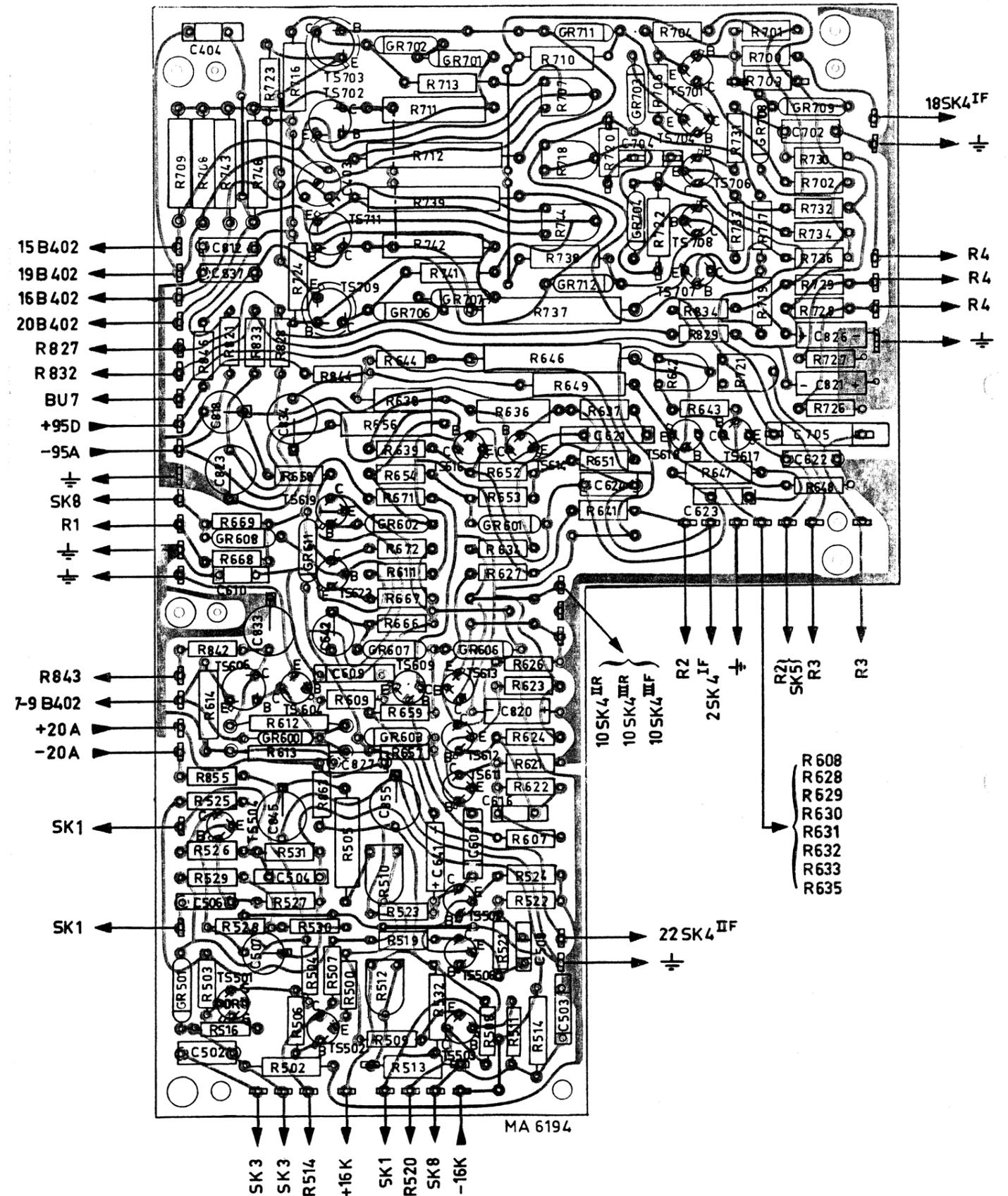
Fig. 33. Printed wiring board of time base generator and horizontal amplifier
