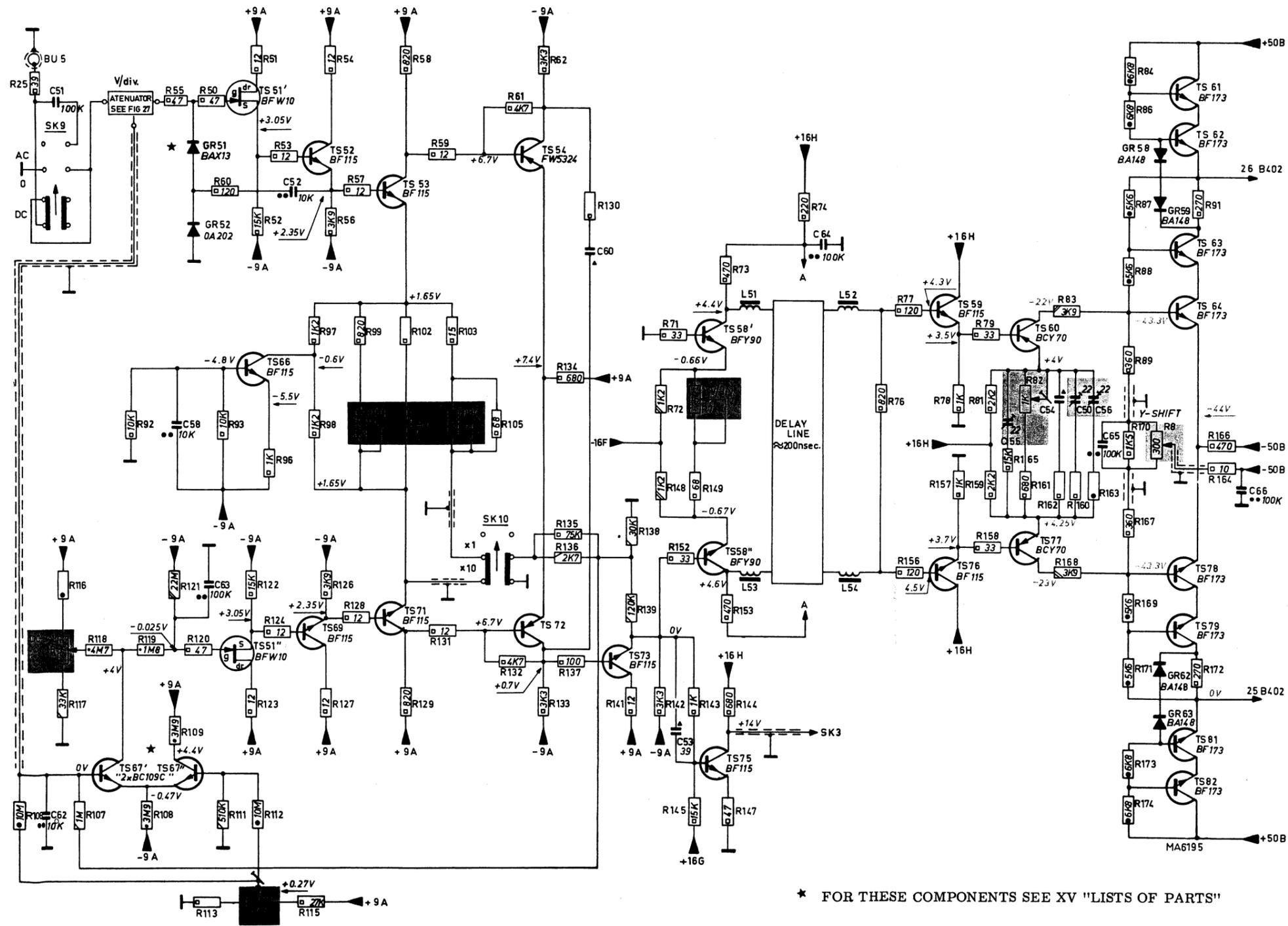
Fig. 30. Circuit diagram of vertical amplifier for channel A
