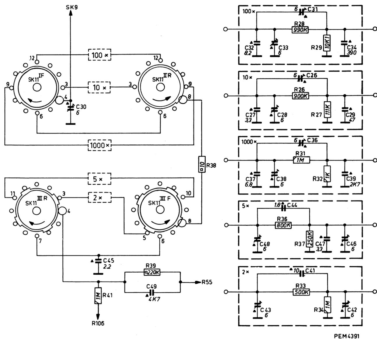
Fig. 27. Circuit diagram of the attenuator for channel A
