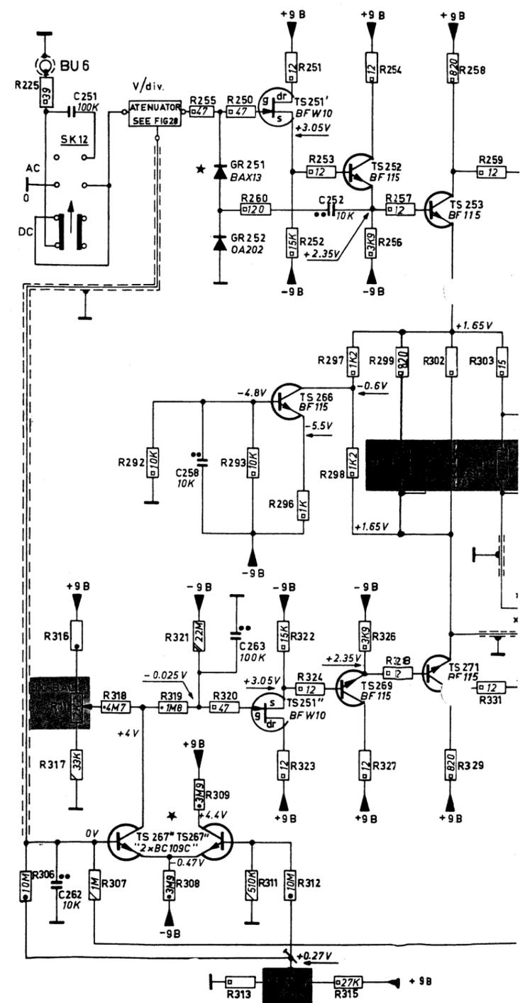
Fig. 31. Circuit diagram of vertical amplifier for channel B
