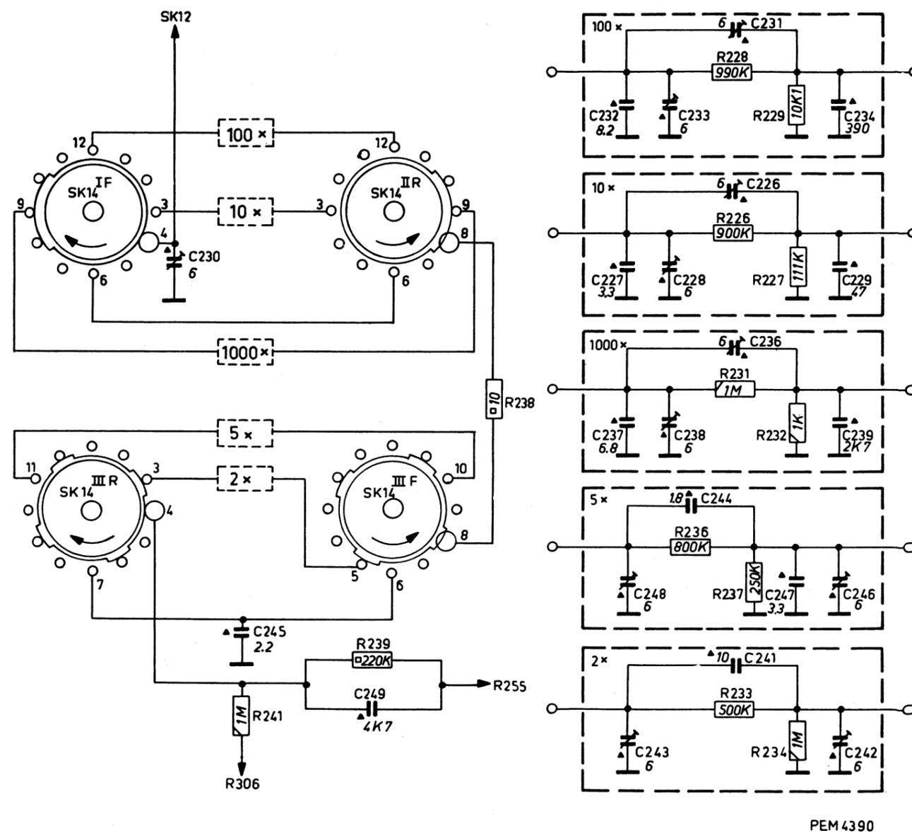
Fig. 28. Circuit diagram of the attenuator for channel B
