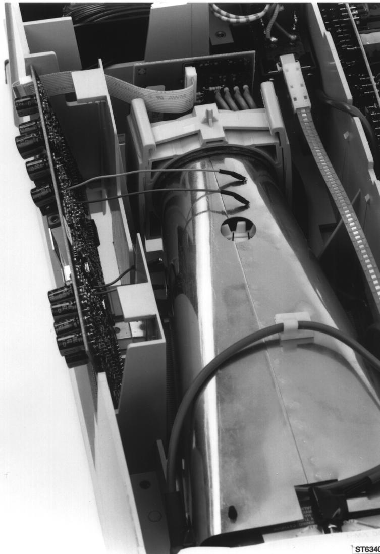
Figure 8.4 Final XYZ amplifier in inclined position
