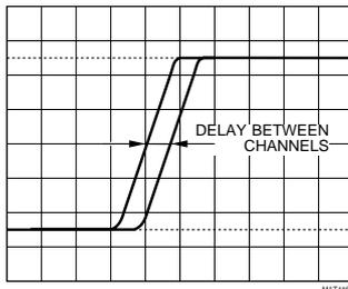
*Figure 6.3 Delay difference  $\leq 0.13$  div in PM3390B/94B or  $\leq 0.05$  div in PM3370B/80B/84B.*
