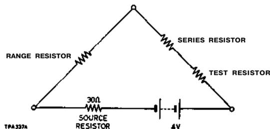
Fig. 2.3 Circuit used in measuring low-wattage resistors
