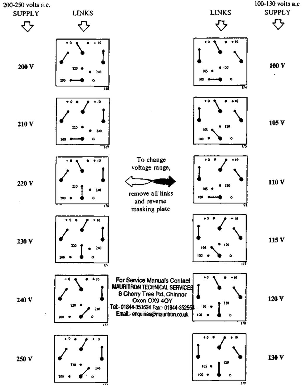
Fig. 4.1 Supply voltage plus settings
