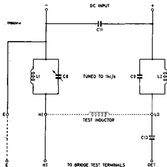
Fig. 3.6 Simplified circuit of d.c. choke adaptor
