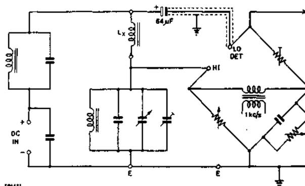
Fig. 2.4 Choke adaptor connected to bridge
