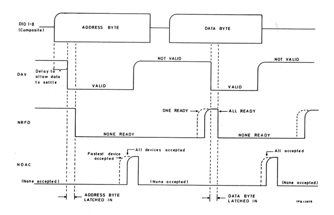
Fig. 7 Handshake procedure - AB1
