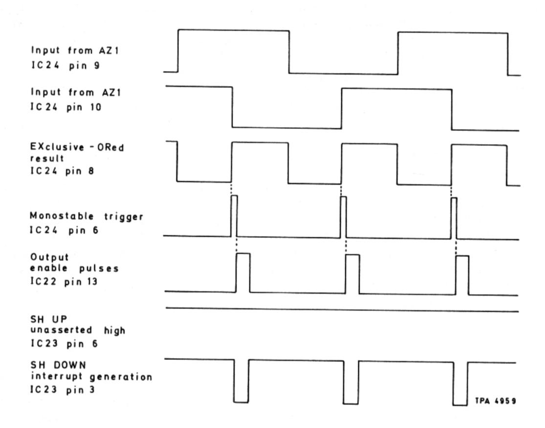
Fig. 5 SET REF LEVEL control direction detector operation. Example shows down movement - AB1
