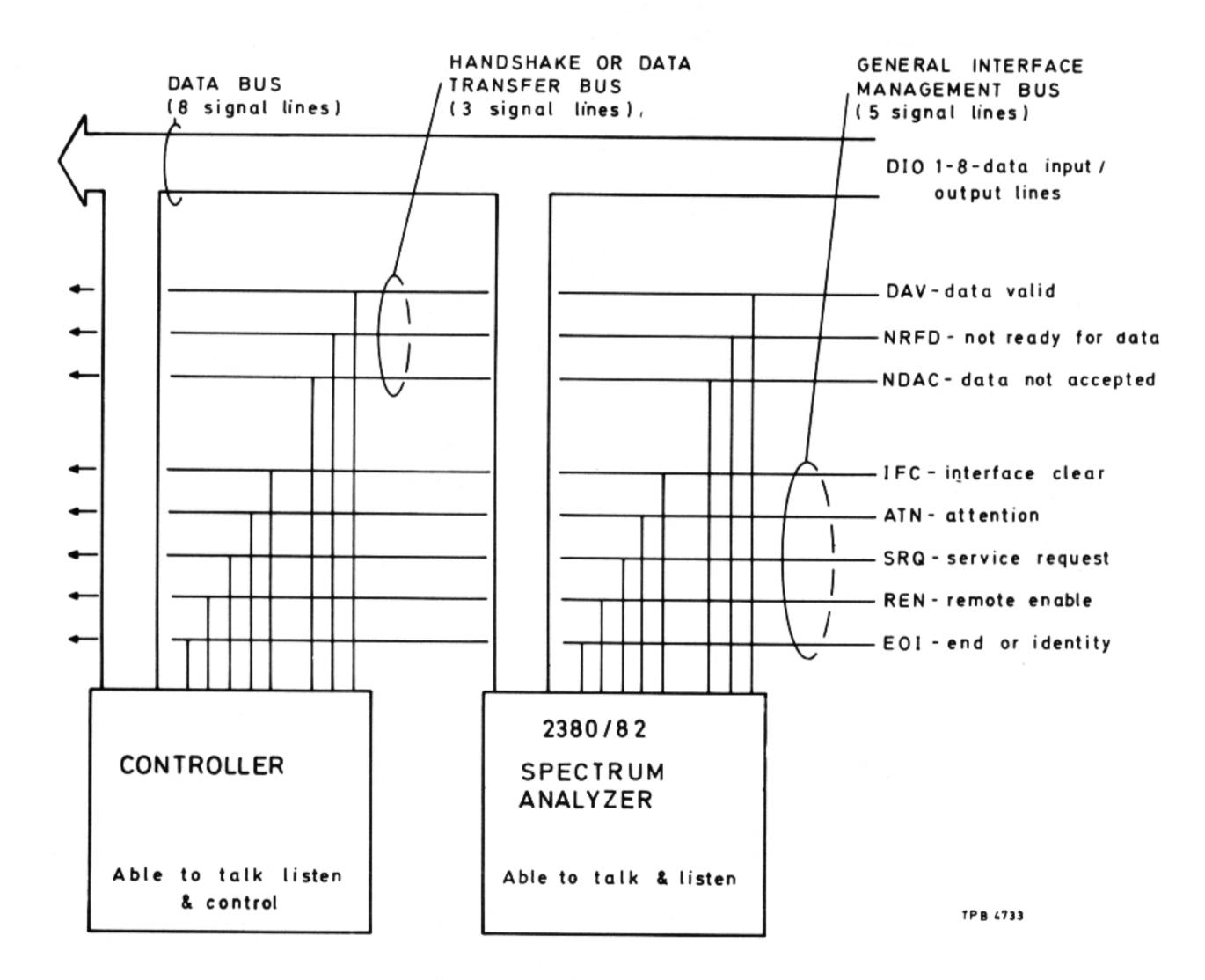
Fig. 6 General Purpose Interface Bus (GPIB) structure - AB1
