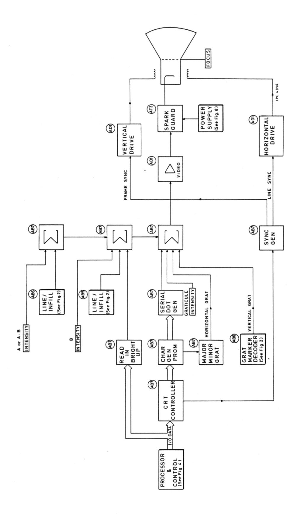
Fig. 3 Display block diagram showing main functions of boards
