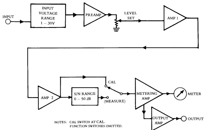
Fig. 3-5 Simplified block diagram for S/N measurement.
