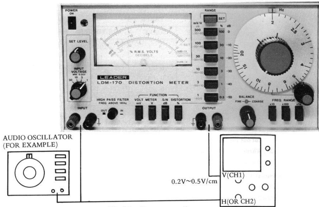
Fig. 2-4 Scope connections.
