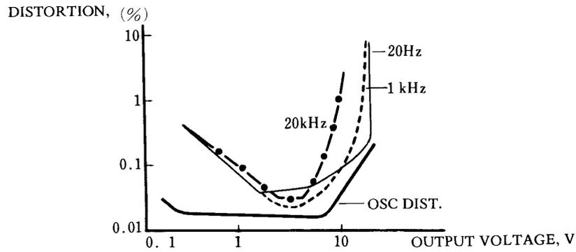
Fig. 2-9 A : Amplifier output VS. distortion.
