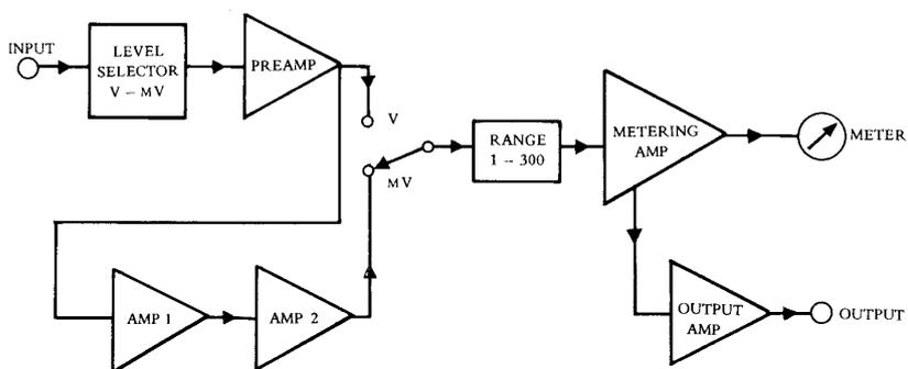
Fig. 3-6 Simplified block diagram for voltage measurement.
