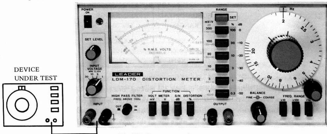
Fig. 2-2 Input connections.
