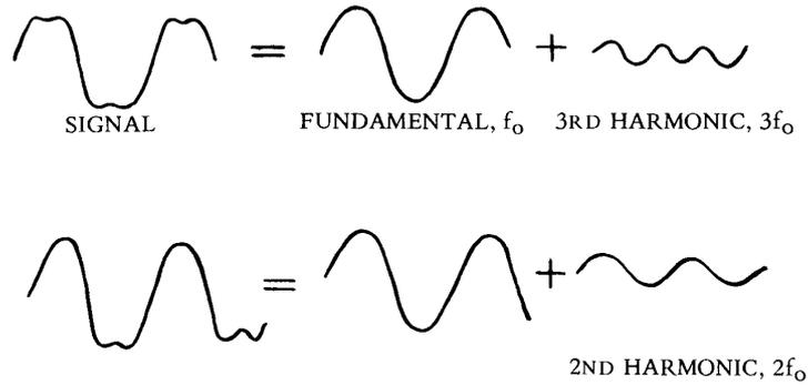
Fig. 3-1 Distorted waveforms.
