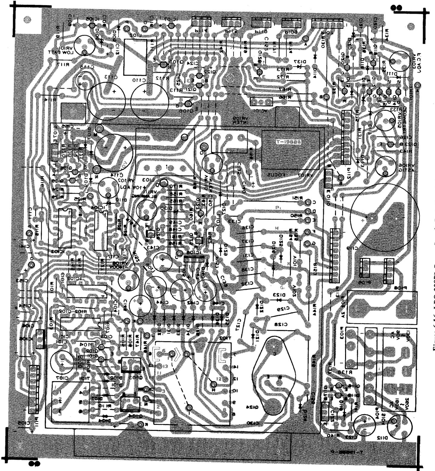
Figure 6-16. LBO-308PL Power Supply P. C. Board T-1988B
