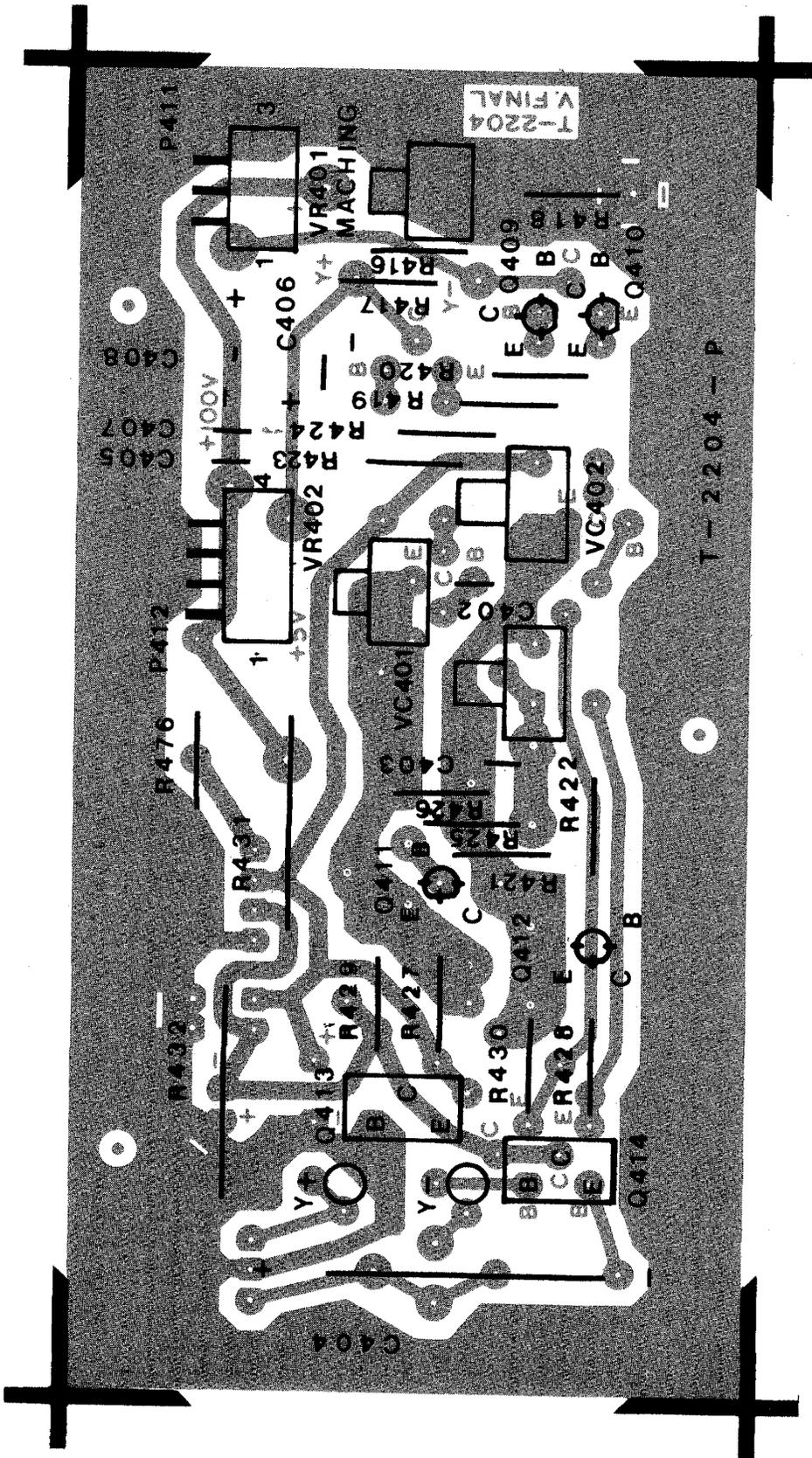
Figure 6-14 LBO-308PL Final Vertical Amp. P. C. Board T-2204
