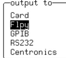
2. Press the button to select a printer, plotter, or graphic protocol (TIFF, BMP, or
