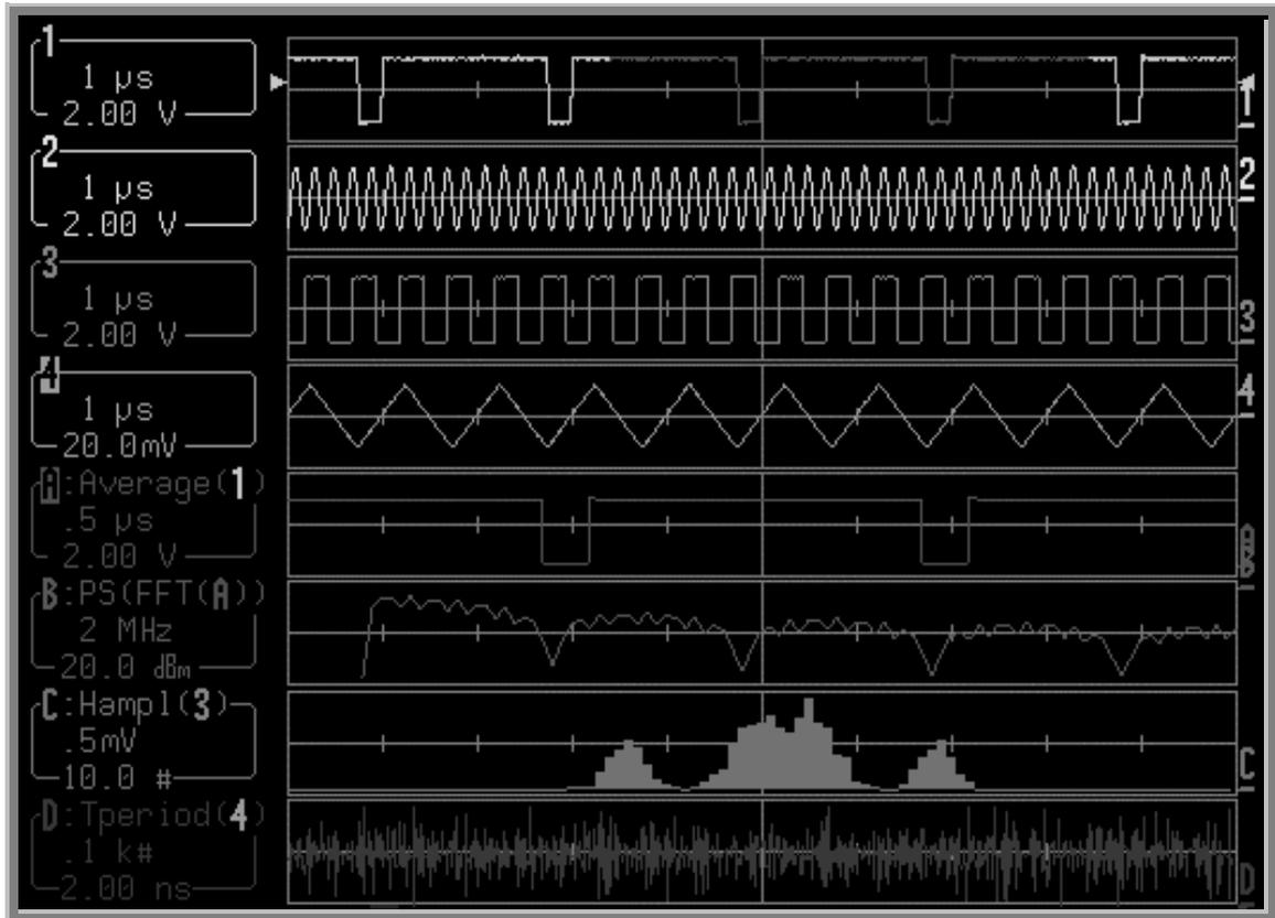
Waveform source descriptions, trace labels and the information they contain will always take the color of their respective traces, as in this four-channel model's Octal-grid, eight-trace display.
