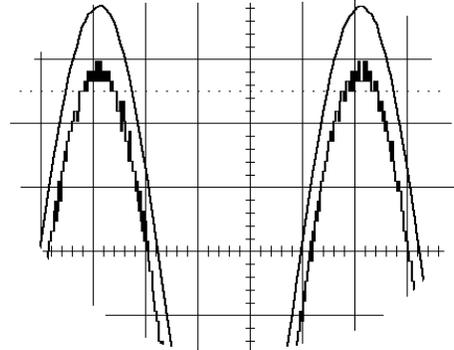
**To reduce noise:** The example below shows enhanced resolution of a noisy signal. The original trace (below left) has been processed by a two-bit enhanced resolution filter. The result (below right) shows a “smooth” trace, where most of the noise has been eliminated.
