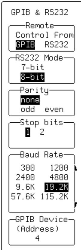
2. Use these menus to set up communication with the PC via GPIB or RS232.
