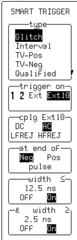
Use these menus to set up to trigger on a glitch, or to create an exclusion trigger (see page 93).
