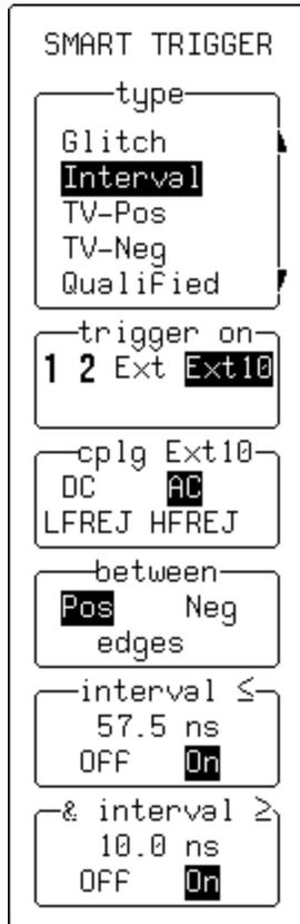
Use these menus to set up for triggering on an interval.
