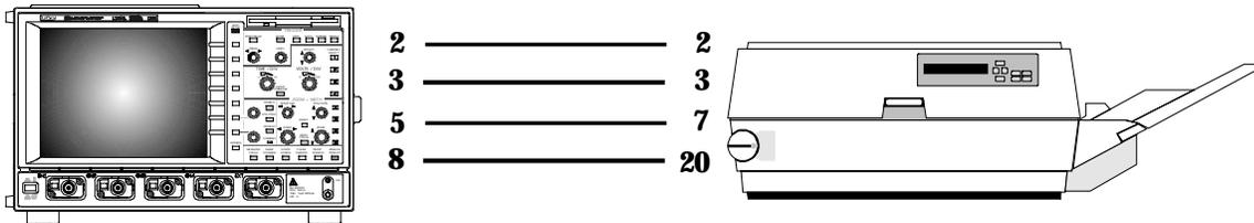
*RS-232-C printer cabling: Connect your scope to a variety of external printers using the rear RS-232-C port. You could also connect to PC via GPIB, and use the computer to control a printer connected via RS-232-C. See Chapter 12, “Use Waverunner with PC,” for computer cabling.*
