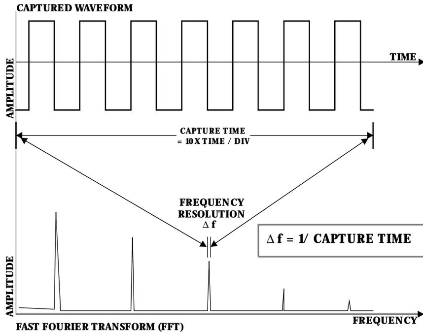
Figure 1. Capture time determines the frequency resolution  $\Delta$ .
