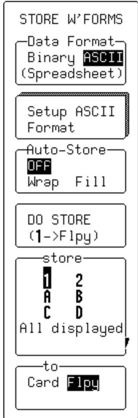
3. Then use these and the menus on the next page to save your displayed waveform to a storage device in an ASCII data format.
