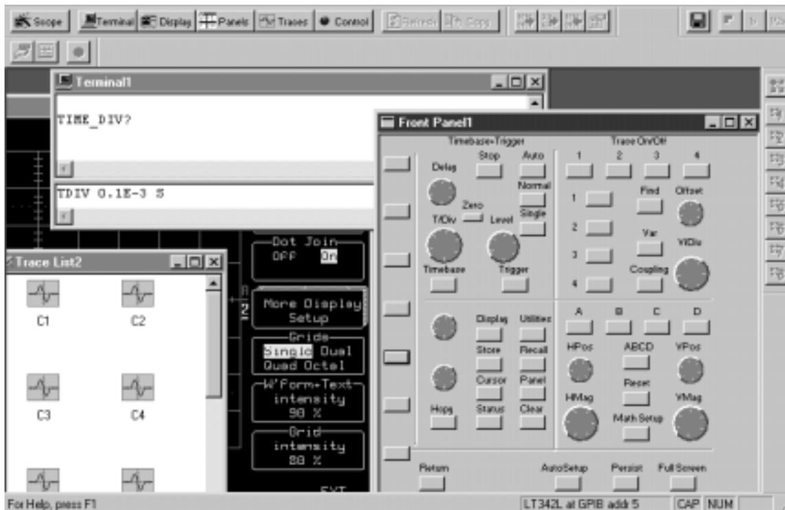
*ScopeExplorer now has a virtual front panel to allow full control of remote scopes.*
