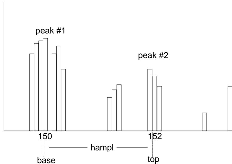
In this histogram, **hampl** is  $152 \text{ mV} - 150 \text{ mV} = 2 \text{ mV}$ .
