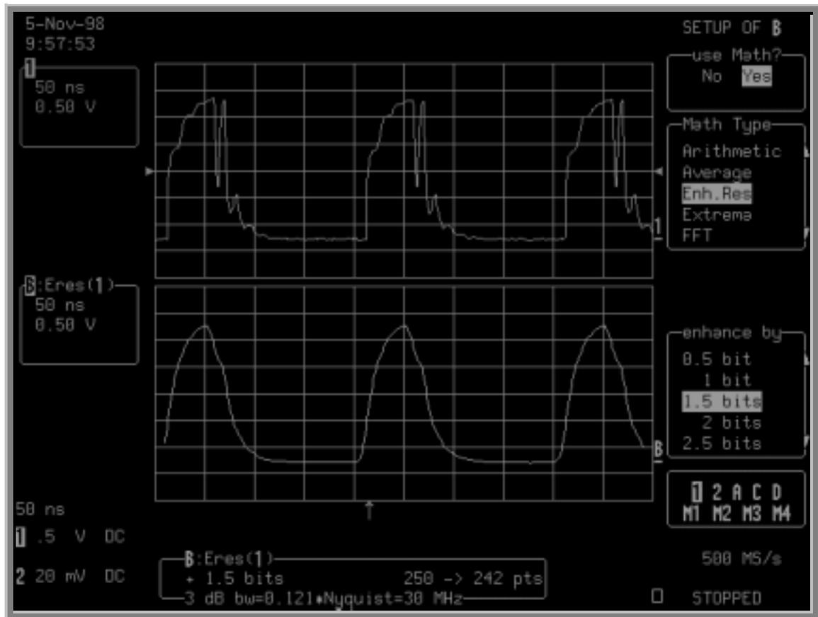
The glitch in the waveform displayed on the top grid has been clearly eliminated by ERES: the result is the waveform on the lower grid. Trace B's label indicates this as the filtered waveform. And the information field below the grids tells you that Trace B is an ERES function of Channel 1, that the waveform has been enhanced by 1.5 bits, and that filtering has reduced the number of points from 250 to 242 (see NOTE on page131) and the bandwidth to 30 MHz.
