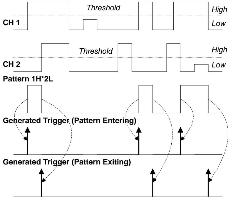
**Pattern Trigger: Triggers when all pattern conditions are met. Bold arrows pointing upward show where triggers occur. Information summarizing the pattern setup is displayed.**
