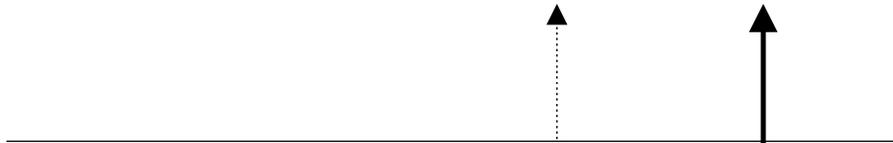
Figure 4. Interval Trigger that triggers when the interval width is smaller than the selected interval. The broken, upward-pointing arrow indicates a potential trigger, while the bold one shows where the actual trigger occurs — on the positive edge within the selected interval.
