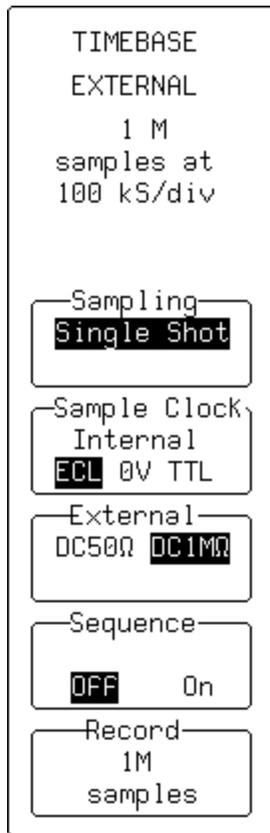
Use an external clock at a fixed frequency (see Appendix) to control and synchronize the sampling with an external signal source connected to the Waverunner rear EXT signal input.
