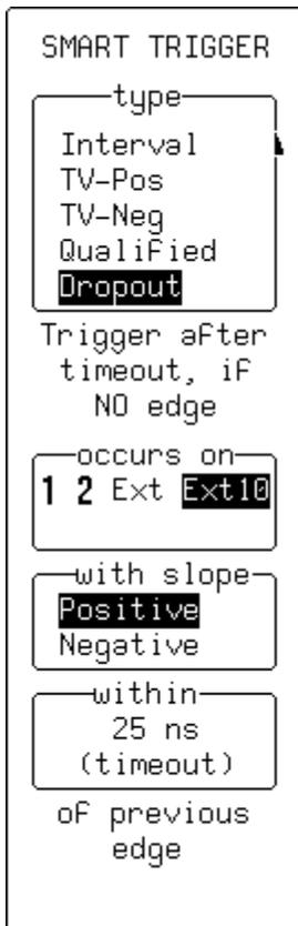
Use these menus to set up the Dropout trigger.
