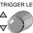
to adjust the trigger’s level to one division from the top of the pulse, for example.
