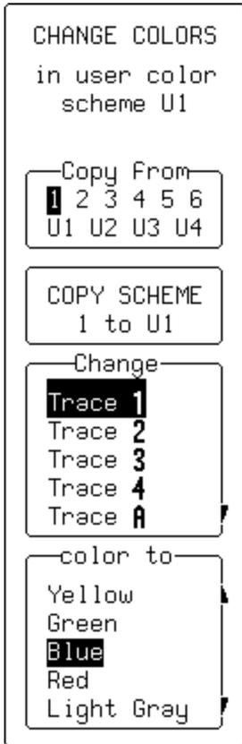
Create your own color scheme; assign colors to traces, grids, or any other on-screen object; or copy a default scheme into a custom one to make personalizing quicker and easier.
