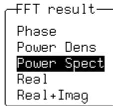
**Power Spectrum** is the signal power, or magnitude, represented on a logarithmic vertical scale: 0 dBm corresponds to the voltage (0.316 V peak), which is equivalent to 1 mW into 50  $\Omega$ . Power Spectrum is suitable for characterizing spectra that contain isolated peaks (dBm).
