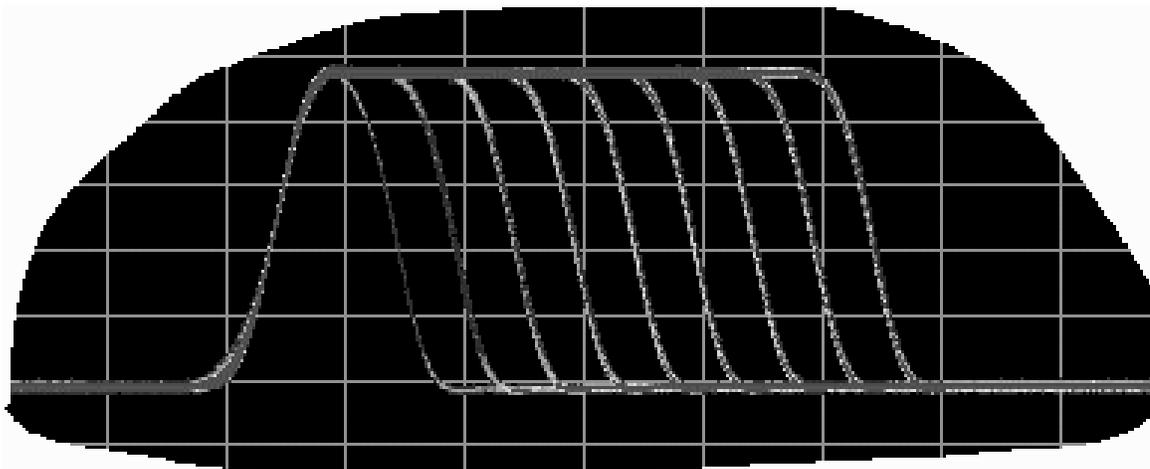
*The same waveform as that shown on page 113 displayed using Color-Graded persistence shows the persistence waveform in a spectrum of colors rather than shades of a single color.*
