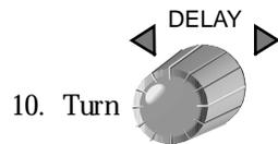
10. Turn to set the trigger point to allow display of the signal's "last normal" period.
