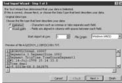
2. The Spreadsheet format generated by WaveRunner uses “,” to delimit columns. Select **Comma** as the delimiter.
