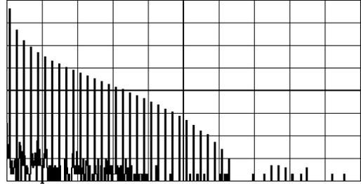
**In low-pass filtering:** The spectrum of a square signal before (above left) and after (above right) enhanced resolution processing. The result clearly illustrates how the filter rejects high-frequency components from the signal. The higher the bit enhancement, the lower the resulting bandwidth.
