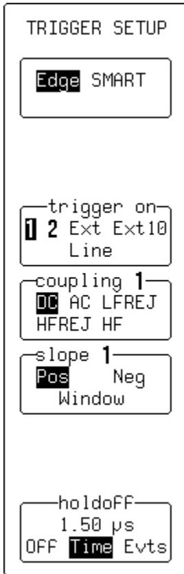
Use them to select the trigger source, the source's coupling, the slope — positive or negative — and the amount of trigger holdoff by time or events.
