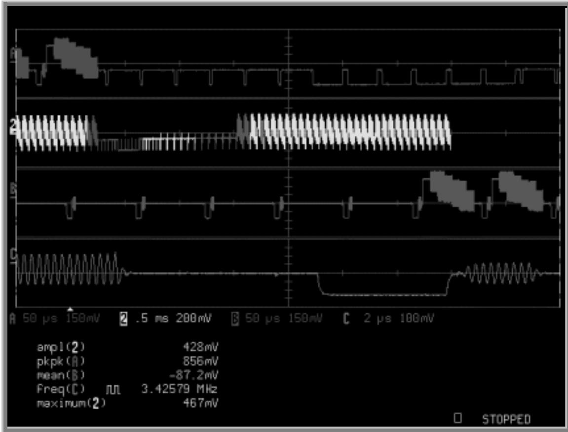
*A special display is automatically used with parameters, whose data are listed beneath the grid (see next page for display setup). Shown here: a Full-Screen, Quad-grid parameter display. Top of facing page: the Standard, Single-grid, parameter display.*
