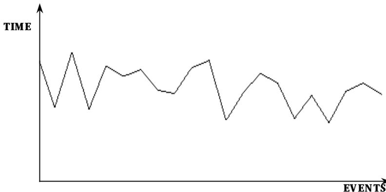
*Figure 3. A trend's horizontal axis is in units of events, with the earlier events in the leftmost part of the waveform and later ones on the right. The vertical axis is in the same units as the trended parameter.*
