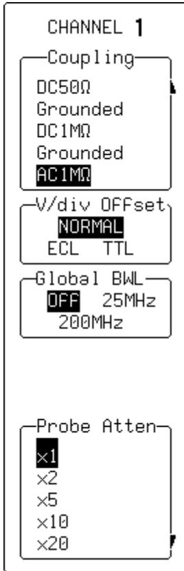
21. Use these menus to set input signal coupling and grounding, the channel bandwidth limit, and the probe attenuation.
