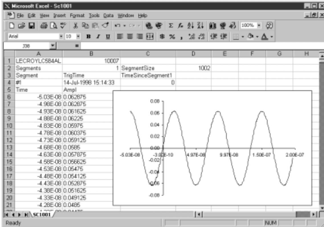
The header created for the spreadsheet contains all the information you'll need to extract various elements from a sequence waveform. Use the following formulae to extract information such as the start and end row of the data for a given segment, or the trigger time of a given segment:
