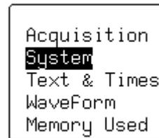
10. Press the top button to highlight and select **System**. The screen will show your Waverunner's serial number, the version of software installed and the date of its release, as well as a full list of your currently installed software and hardware.
