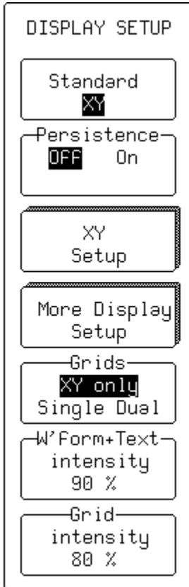
3. Use these menus to set up your XY display, and to access other display setup menus if desired.
