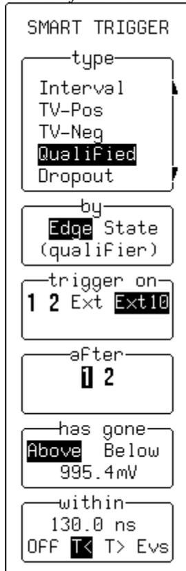
Use these menus to set up an Edge or State Qualified trigger.
