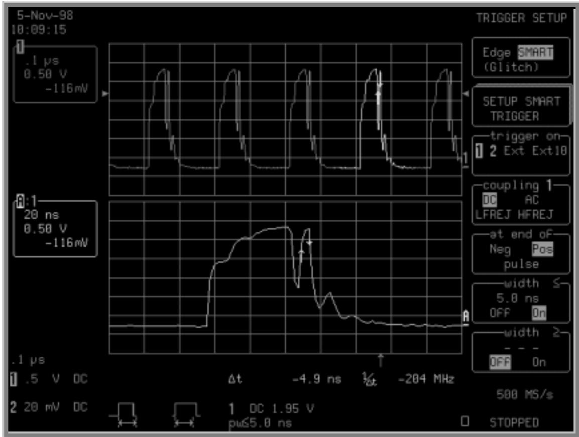
Trigger on a glitch of width  $\leq 5.0$  ns on the negative slope. Here, the glitch is marked by arrow cursors on the waveform. Trace A on the lower grid is a zoom of the waveform on the top grid. Information on the trigger is given beneath the grid.
