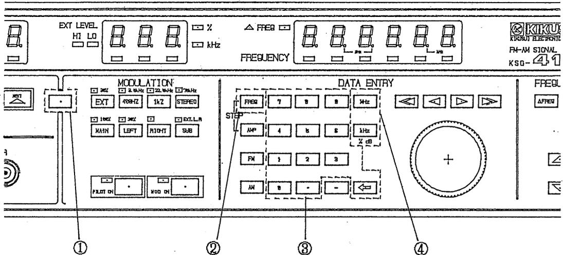
Input is set in the sequence ①, ②, ③, ④ shown in the diagram above.
