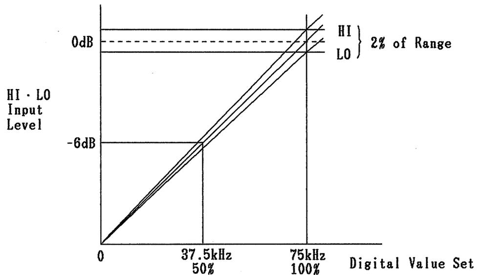
The diagram above shows the relationship between modulation input levels. When the input level is adjusted and is within the HI, LO range, the error in the setting will be  $\pm 2\%$ . The modulation is set internally to the digital set value based on the HI, LO levels.
