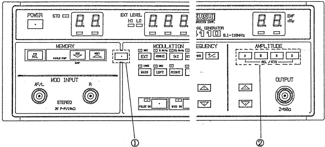
The four keys ② **A** to **D** shown in the diagram above can store output levels without using the main memory.
