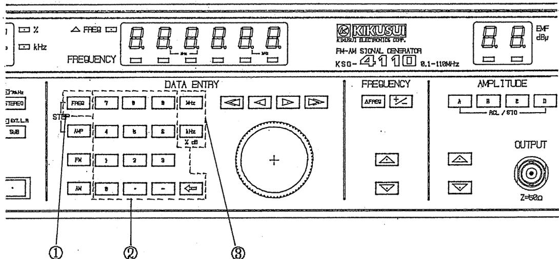
Press the **FREQ** key and input the desired values using the Numeric Keys. Operate in the sequence indicated by the numerals ①, ② and ③ in the diagram above.
