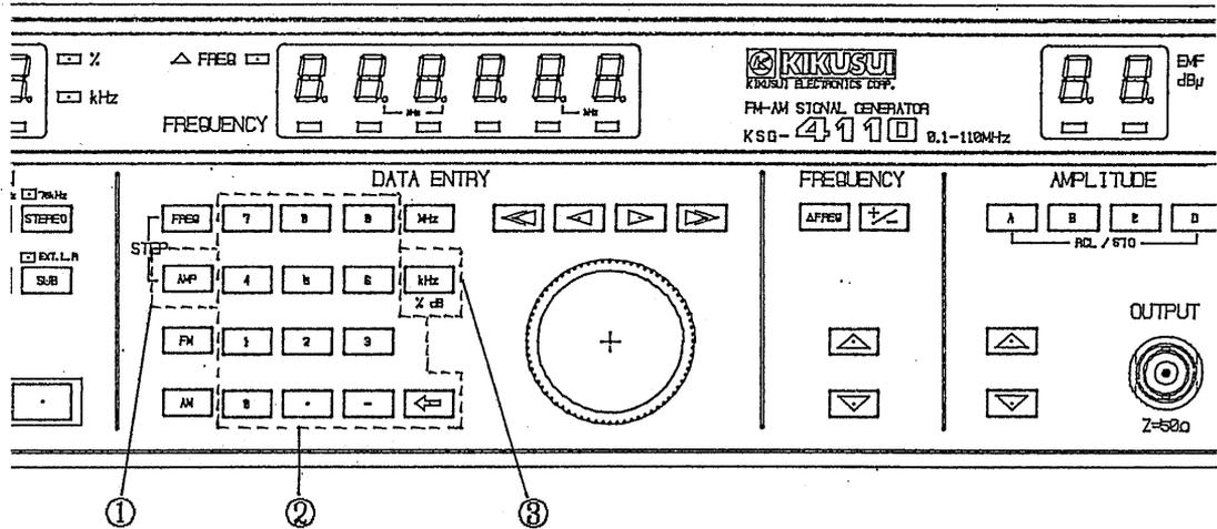
Press the **AMP** key and continuously input desired values using the numeric keys. Operation is in the sequence ①, ②, ③ shown in the diagram above. If a key other than those shown inside the dotted lines is pressed, the value displayed before the **AMP** key was pressed will again be displayed.
