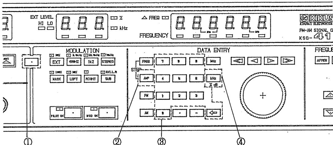
Input is set in the sequence ①, ②, ③, ④ shown in the diagram above.
