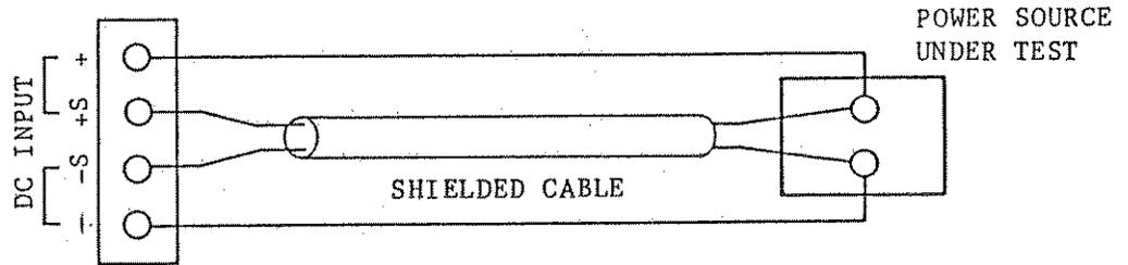
Note that power leads may be connected to the DC INPUT terminals on either the front or rear of the Load.
