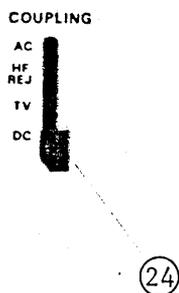
AC: Trigger signal is applied through an AC coupling circuit.
