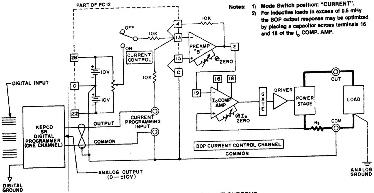
FIG. 3-15 DIGITAL CONTROL OF THE BOP OUTPUT CURRENT
