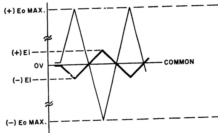
FIG. 3-8 GRAPHS OF POSSIBLE BOP INPUT/OUTPUT WAVE-SHAPES
