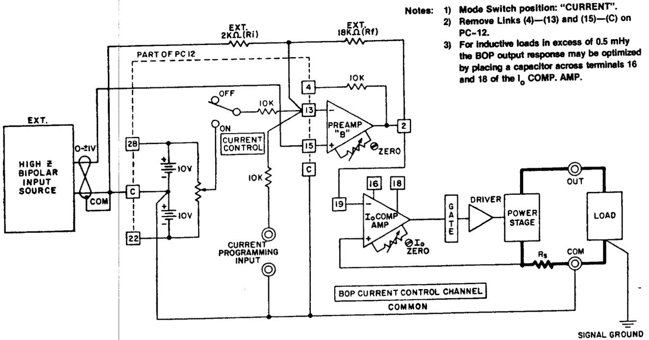
FIG. 3-16 BOP OUTPUT CURRENT CONTROL WITH A HIGH IMPEDANCE (±)1 VOLT SIGNAL SOURCE
