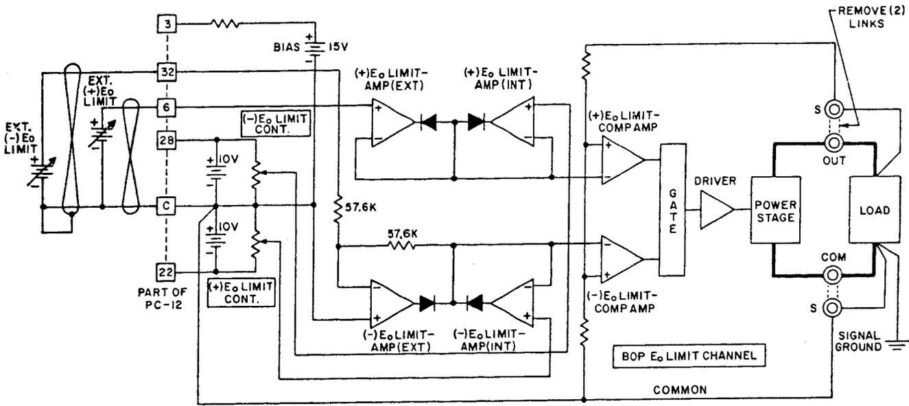
FIG. 3-25 INDEPENDENT REMOTE CONTROL OF THE BOP
