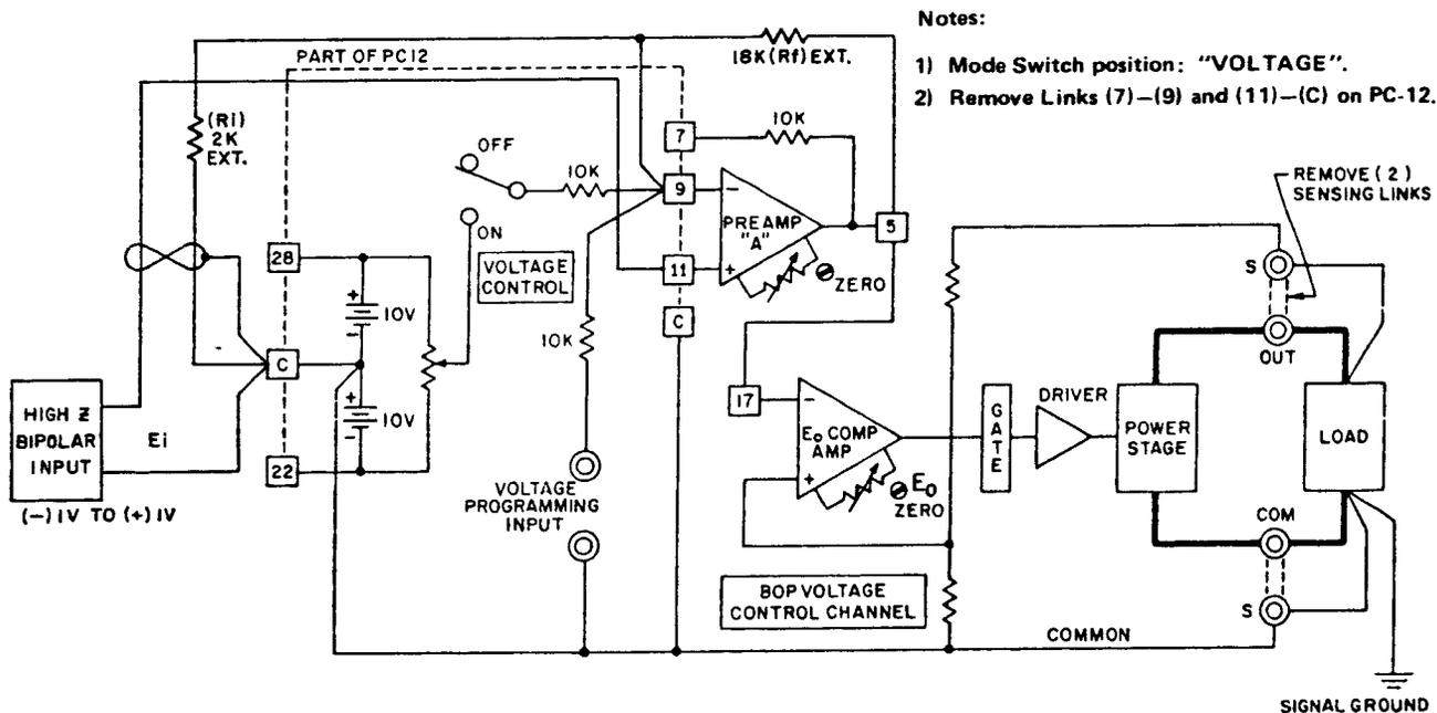
FIG. 3-7 BOP D-C OUTPUT VOLTAGE CONTROL WITH A HIGH IMPEDANCE. (±) 1V SIGNAL SOURCE.
