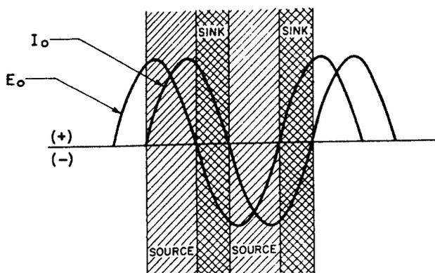
FIG. 1-3 BOP OUTPUT WAVE FORM WITH PHASE SHIFT
