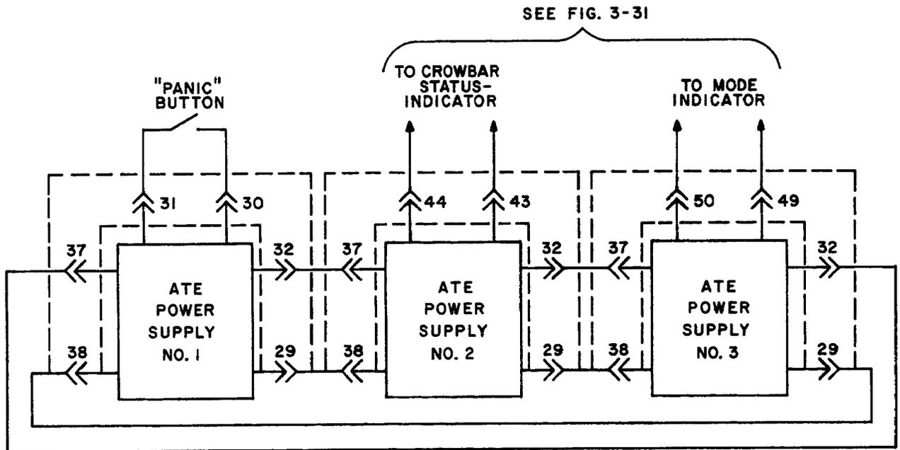
FIG. 3-19 MULTIPLE POWER SUPPLY FAULT DETECTION LOOP.
