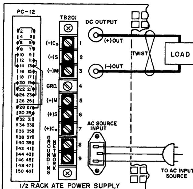
FIG. 3-3 LOAD CONNECTION METHOD I, LOCAL ERROR SENSING.
