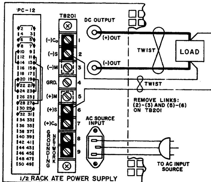
FIG. 3-4 LOAD CONNECTION, METHOD II USING REMOTE ERROR SENSING.
