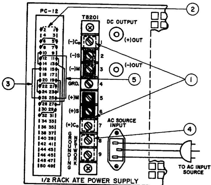
STEP 1: Remove Links (1)-(2) and (6)-(7) on TB201. This removes the output capacitor ( $C_o$ ).
