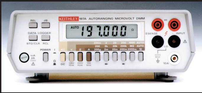
The Model 197A is a lightweight, portable DMM with a battery pack option. It combines 5½-digit resolution (on a 220,000-count display) with 1μV, 1nA, 1mΩ sensitivity. Basic DCV accuracy is 0.011%.
