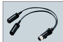
Converts 13-pin ACC connector to 7-pin + 8-pin ACC connector for connection with IC-PW1/1EURO.
