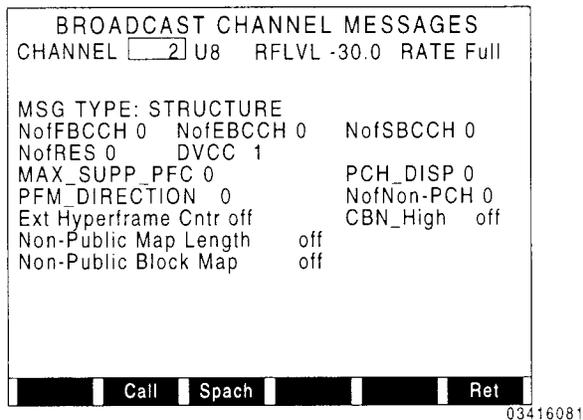
Select the channel, band, RF level, and rate to use. Move cursor to MSG TYPE and select the message to be sent. Once the message is selected, the appropriate data fields appear. Set the fields to the desired settings. Any change made to any of the data fields is reflected immediately in the data stream in the FDCCH signal.
