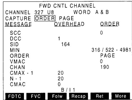
6. Move cursor to CHANNEL and use DATA ENTRY Keys to enter a Control Channel and associated cellular band. Press **ENTER**.
