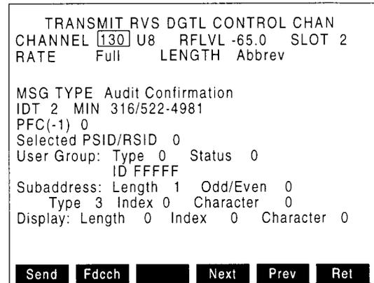
Select the RF Level, cellular channel and band and TDMA slot in which to transmit. Move cursor to the RATE field and, pressing **ENTER**, toggle the rate to Full or Half. Move cursor to the LENGTH field and, pressing **ENTER**, toggle the LENGTH to normal or abbreviated.
