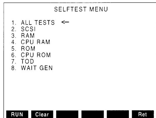
2. Using Field Select keys, move arrow to "1. ALL TESTS" and press **RUN F1** to automatically execute each test in sequence, starting with "2. SCSI". P or F appears beside each test indicating a pass or fail. Press **Abort F5** at anytime to abort the automatic running of the self tests. (The Abort Softkey appears only when running "ALL TESTS.")
