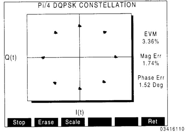
When the Pi/4 DQPSK Constellation screen appears, the CSA begins to continually sample the signal from the Base Station. The constellation of decision points is repeatedly plotted from each sample. In addition, the values of RMS Error Vector Magnitude (EVM), RMS Magnitude Error and RMS Phase Error are repeatedly updated.
