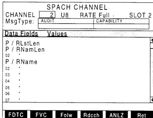
Select the cellular channel, band and TDMA slot to monitor. Move cursor to the RATE field and, pressing **ENTER**, toggle the rate to Full or Half.
