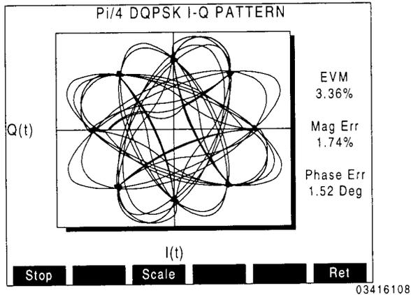
When the Pi/4 DQPSK I-Q Pattern screen appears, the CSA begins to continually sample the signal from the Mobile Station. The I/Q pattern and constellation is repeatedly plotted from each sample, clearing the pattern display area at the end of each plot sequence. In addition, the values of RMS Error Vector Magnitude (EVM), RMS Magnitude Error and RMS Phase Error are repeatedly updated from each sample.
