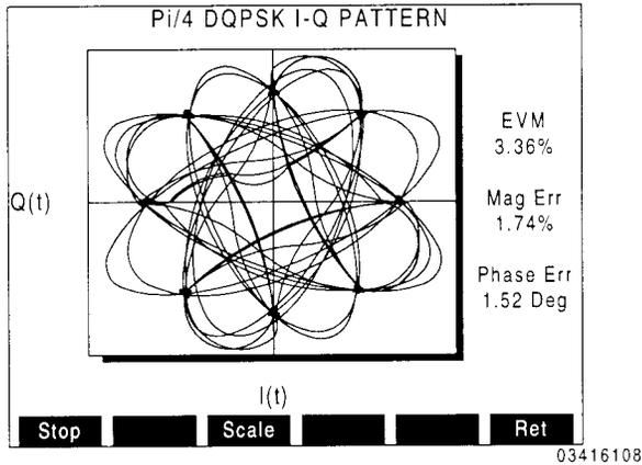
When the Pi/4 DQPSK I-Q Pattern screen appears, the CSA begins to continually sample the signal from the Mobile Station. The I/Q pattern and constellation is repeatedly plotted from each sample, clearing the pattern display area at the end of each plot sequence. In addition, the values of RMS Error Vector Magnitude (EVM), RMS Magnitude Error and RMS Phase Error are repeatedly updated from each sample.
