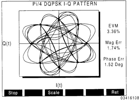
When the Pi/4 DQPSK I-Q Pattern screen appears, the CSA begins to continually sample the signal from the Base Station. The I/Q pattern and constellation is repeatedly plotted from each sample, clearing the pattern display area at the end of each plot sequence. In addition, the values of RMS Error Vector Magnitude (EVM), RMS Magnitude Error and RMS Phase Error are repeatedly updated from each sample.
