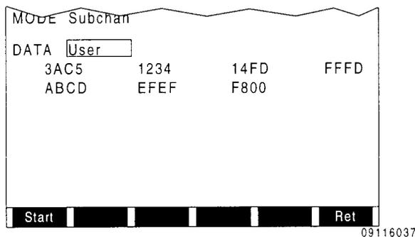
Press **Start F1** to begin sending the repetitive data words on the RDCCH. Press **Stop F1** to stop transmitting on the RDCCH.
