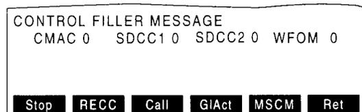
*Call F3* displays the Call Screen. *GIAct F4* displays the Global Action screen. *MSCM F5* displays the Mobile Station Control screen.
