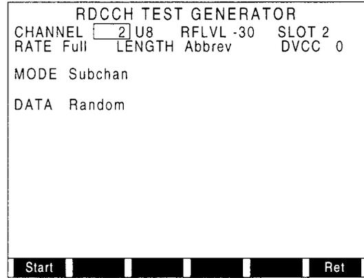
Select the RF level, cellular channel, band and TDMA slot in which to transmit. Move cursor to the RATE field and, pressing *ENTER*, toggle the rate to Full or Half. Move cursor to the LENGTH field and, pressing *ENTER*, toggle the LENGTH to normal or abbreviated. Select the DVCC (0 to 255). Move cursor to the MODE field and, pressing *DATA SCROLL* ↑, select Contiguous (every TDMA block or 1/2 frame) or Subchannel (every 6th TDMA block) transmission; press *ENTER*.
