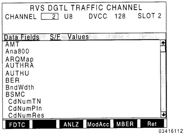
Press **ModAcc F4** to display the Mobile Station Modulation Accuracy and Power screen:
