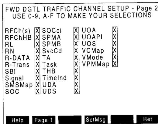
Use the FIELD SELECT Keys to move the cursor and use the DATA ENTRY Keys to select the additional fields shown.
