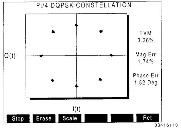
When the Pi/4 DQPSK Constellation screen appears, the CSA begins to continually sample the signal from the Mobile Station. The constellation of decision points is repeatedly plotted from each sample. In addition, the values of RMS Error Vector Magnitude (EVM), RMS Magnitude Error and RMS Phase Error are repeatedly updated.
