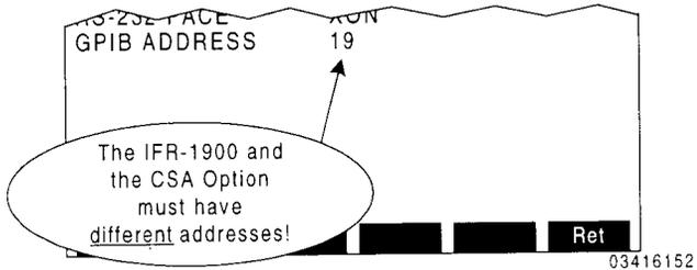
2. Using cursor and specify GPIB address for the CSA.
