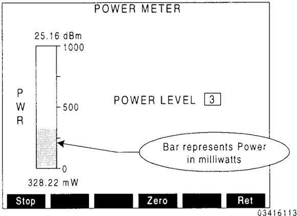
When the Power Meter screen appears, the CSA begins to continually sample the signal from the Base Station. The values and graphical representation of power is repeatedly updated from each sample. Press **Stop F1** to stop sampling and freeze display.
