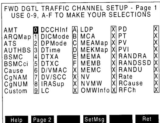
The data fields displayed on the FDTC screen are selected from this menu. Use the FIELD SELECT Keys to move the cursor and use the DATA ENTRY Keys to select the fields as shown.
