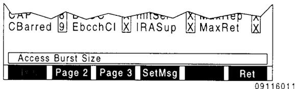
Pressing **SetMsg F4** provides preset data field selections by message type. Press **DATA SCROLL** ↑ until desired message type appears in the shaded field. Press **ENTER** to accept the current message type presets; otherwise, press **ESC F6**. All data field selections made prior to using the SetMsg function are not retained; however, manual changes afterward are allowed.
