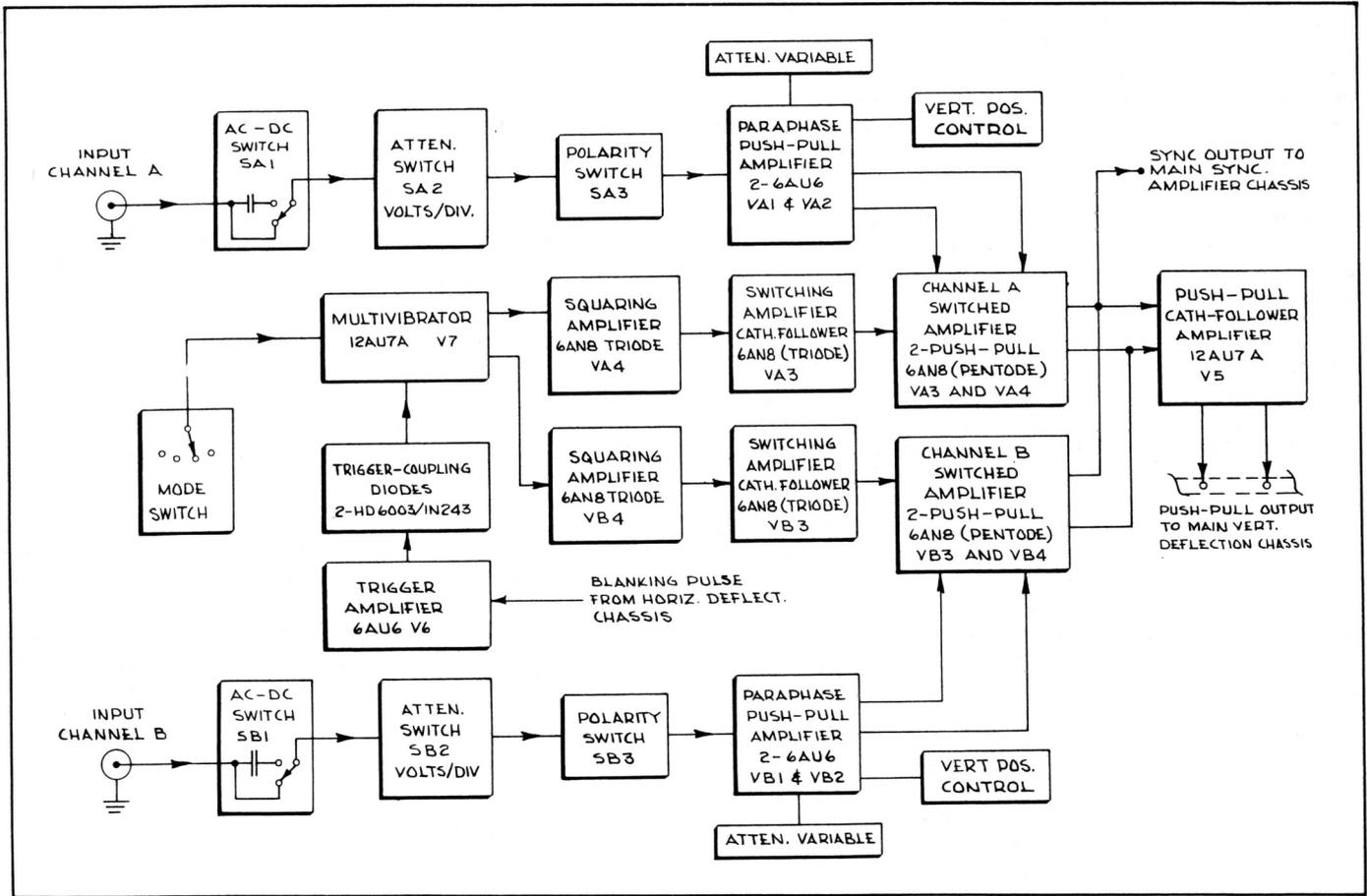
Figure 20. Block Diagram, WB/DI/11 or WB/DI/11-D Dual Trace Preamplifier
