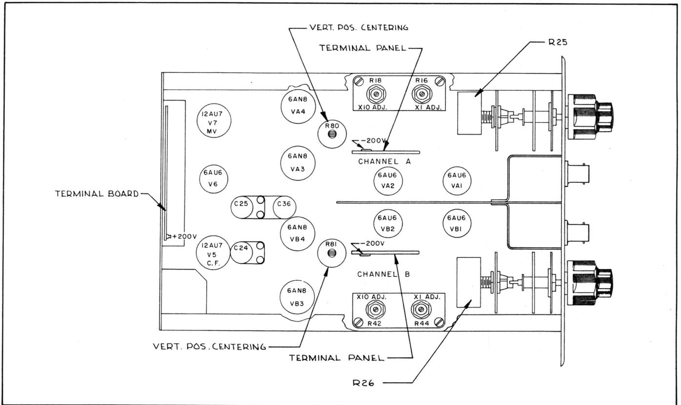
Figure 22. Internal Adjustment Controls and Tube Layout, WB/DI/11 or WB/DI/11-D Dual Trace Preamplifier
