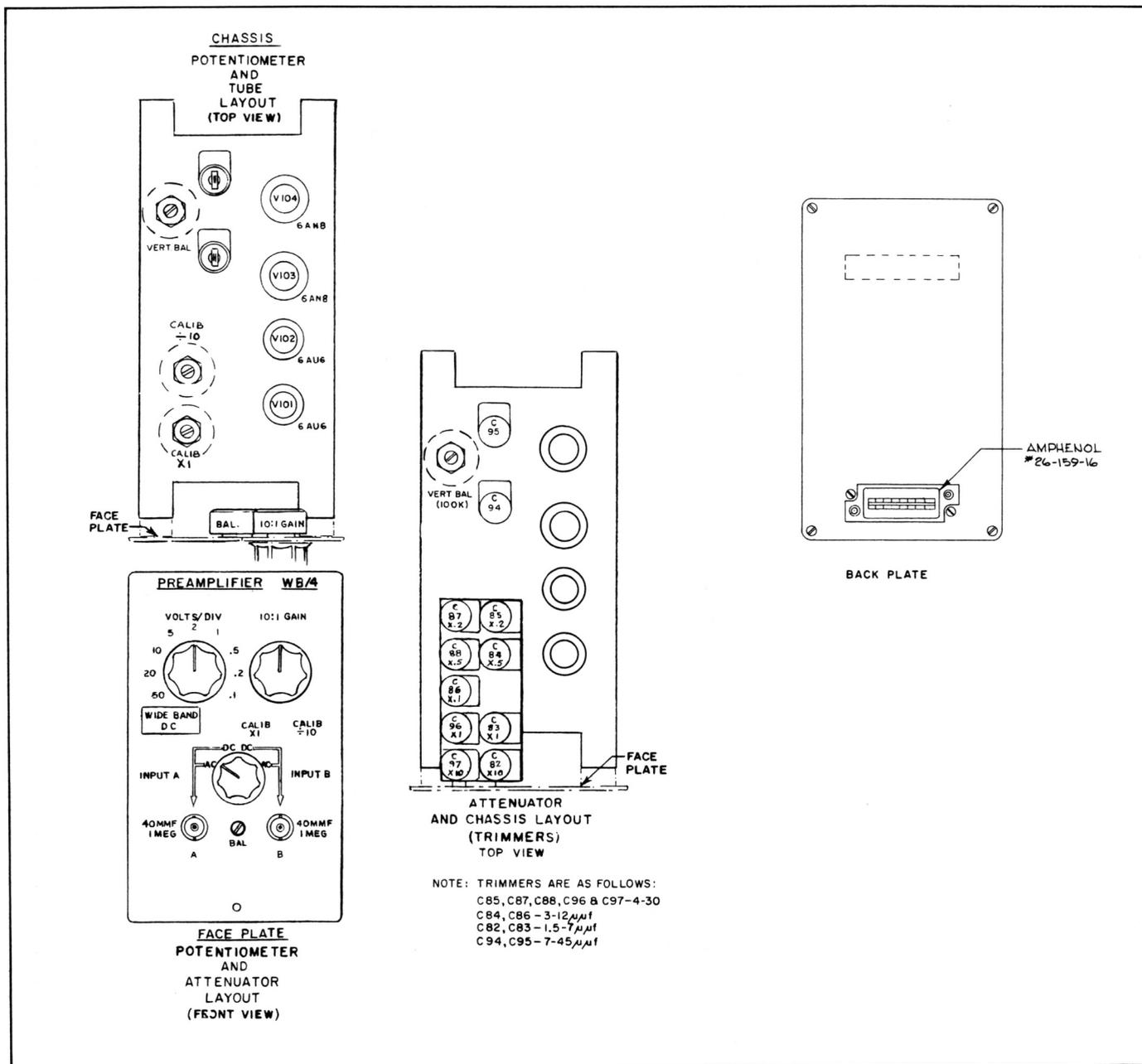
Figure 16. Tube, Potentiometer, and Trimmer Layout, WB/4 Preamplifier
