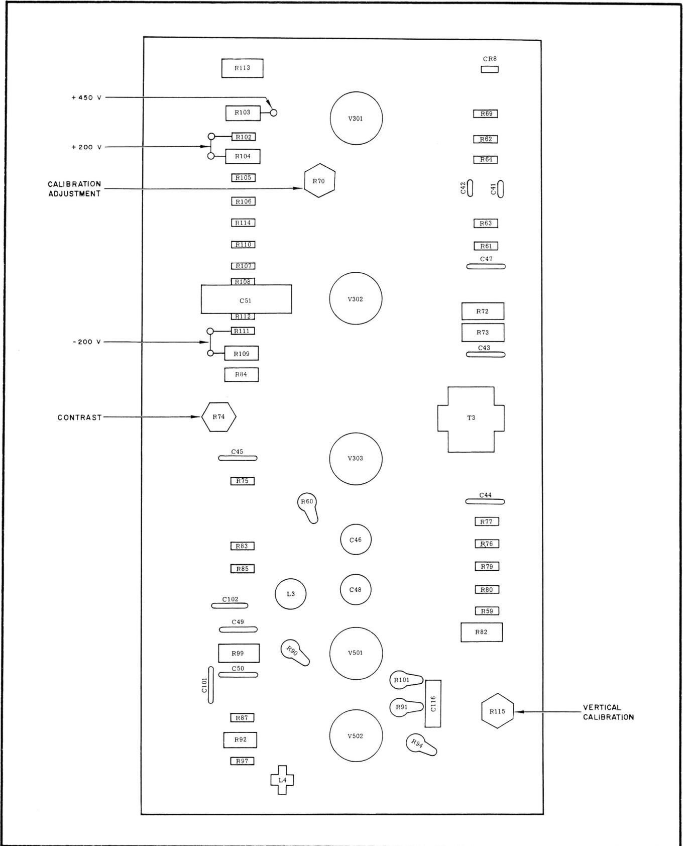
Calibrate Voltage, Storage Circuit, and Vertical Amplifier Location of Parts
