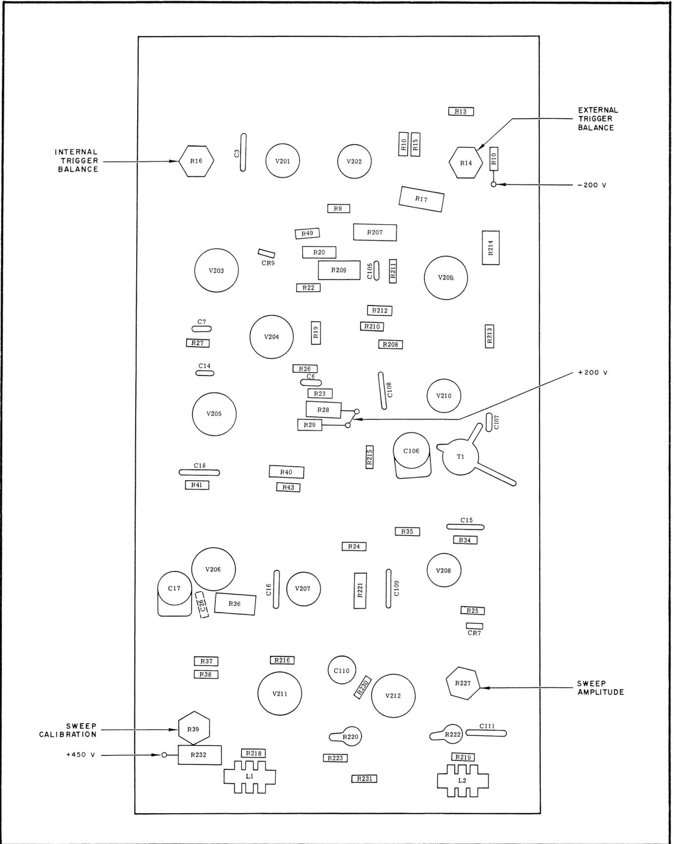
Sweep Circuits, Blanking, and Horizontal Amplifier, Location of Parts
