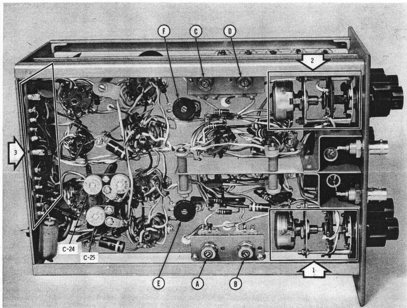
Figure 24. Left-Hand Side View, WB/DI/11 or WB/DI/11-D Dual Trace Preamplifier
