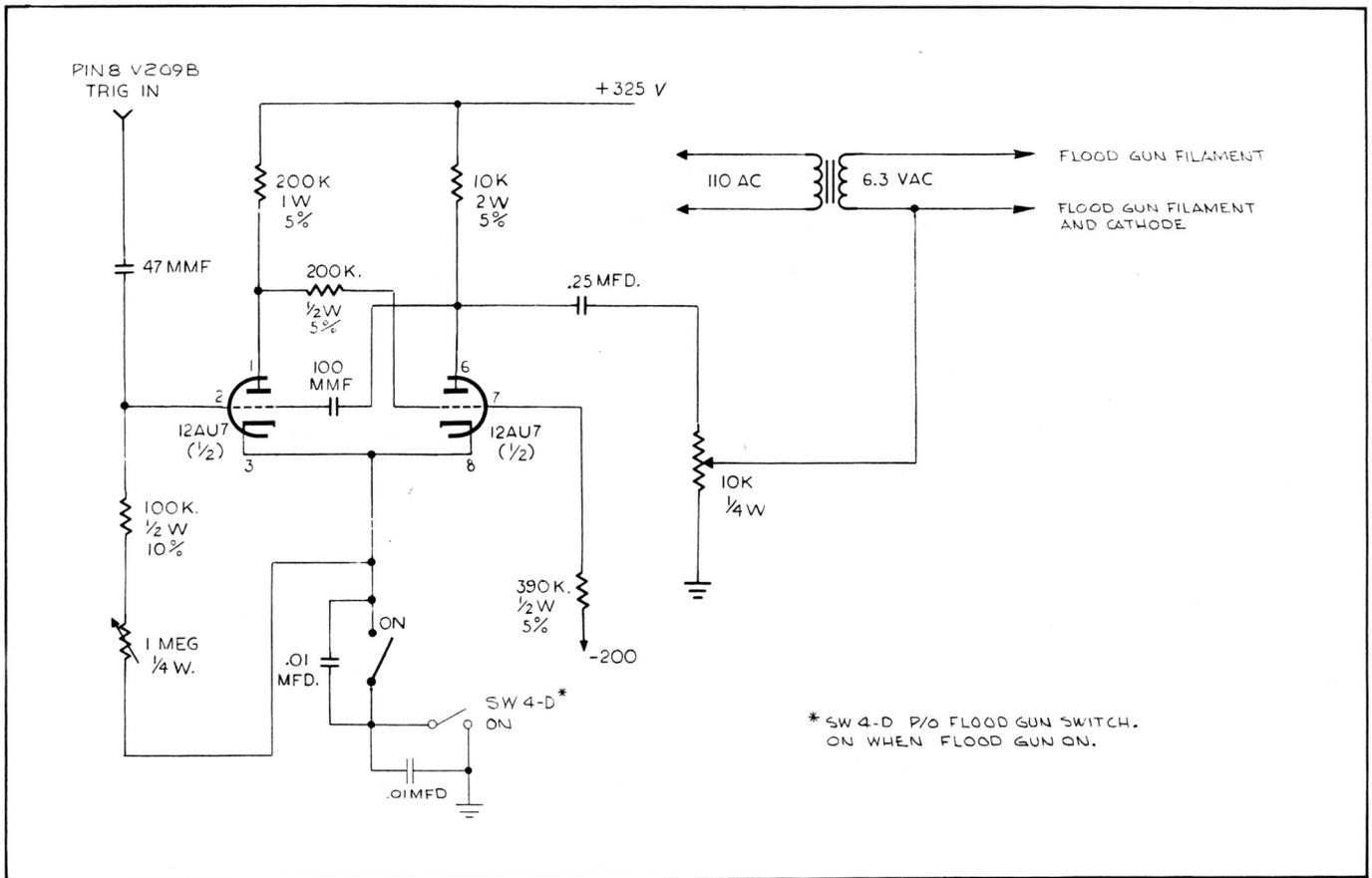
Figure 14. Schematic, Speed Enhancement Circuit
