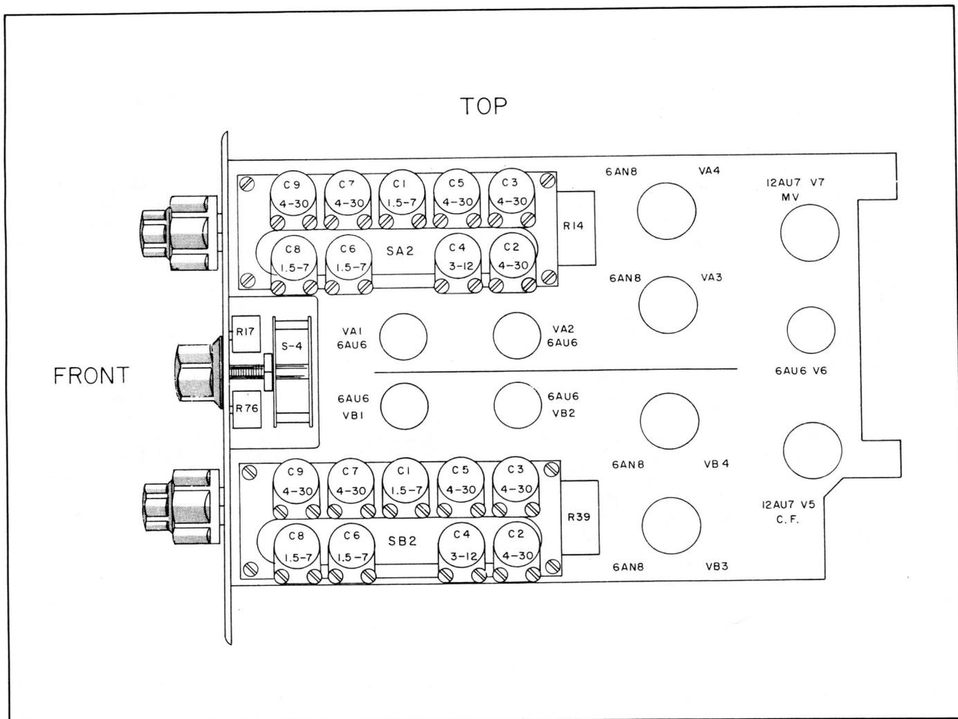
Figure 21. Controls and Tube Layout, WB/DI/11 or WB/DI/11-D Dual Trace Preamplifier
