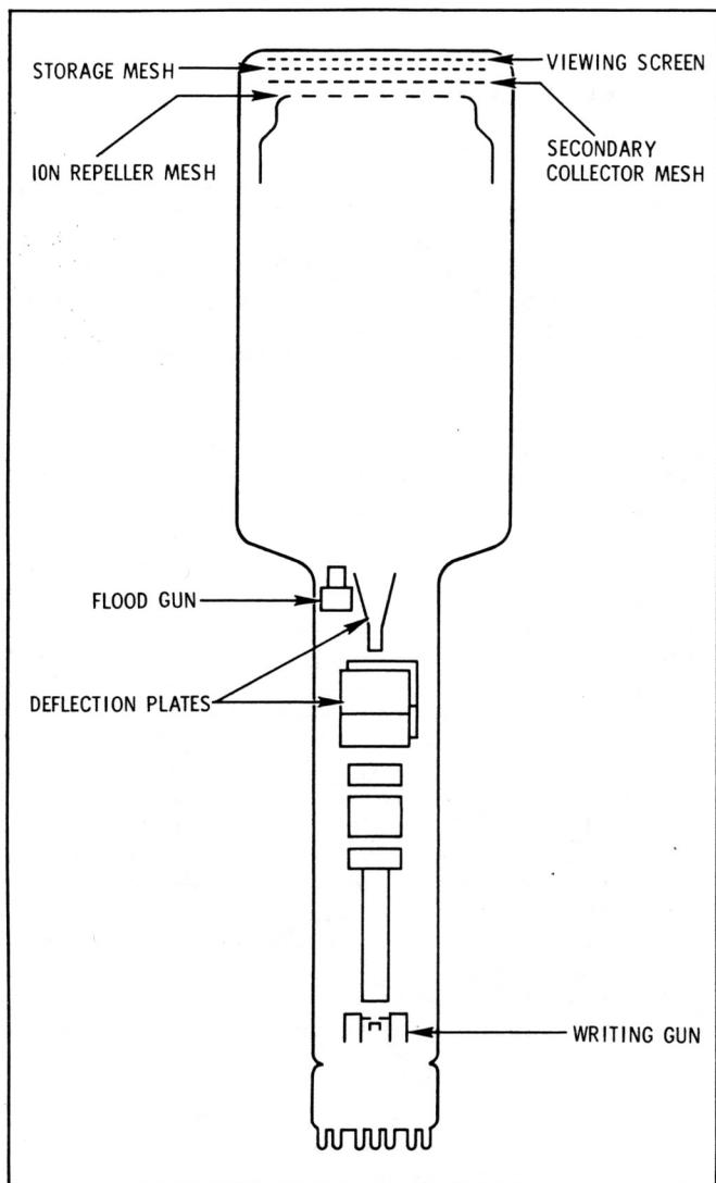
Figure 2. MEMOTRON Tube,
