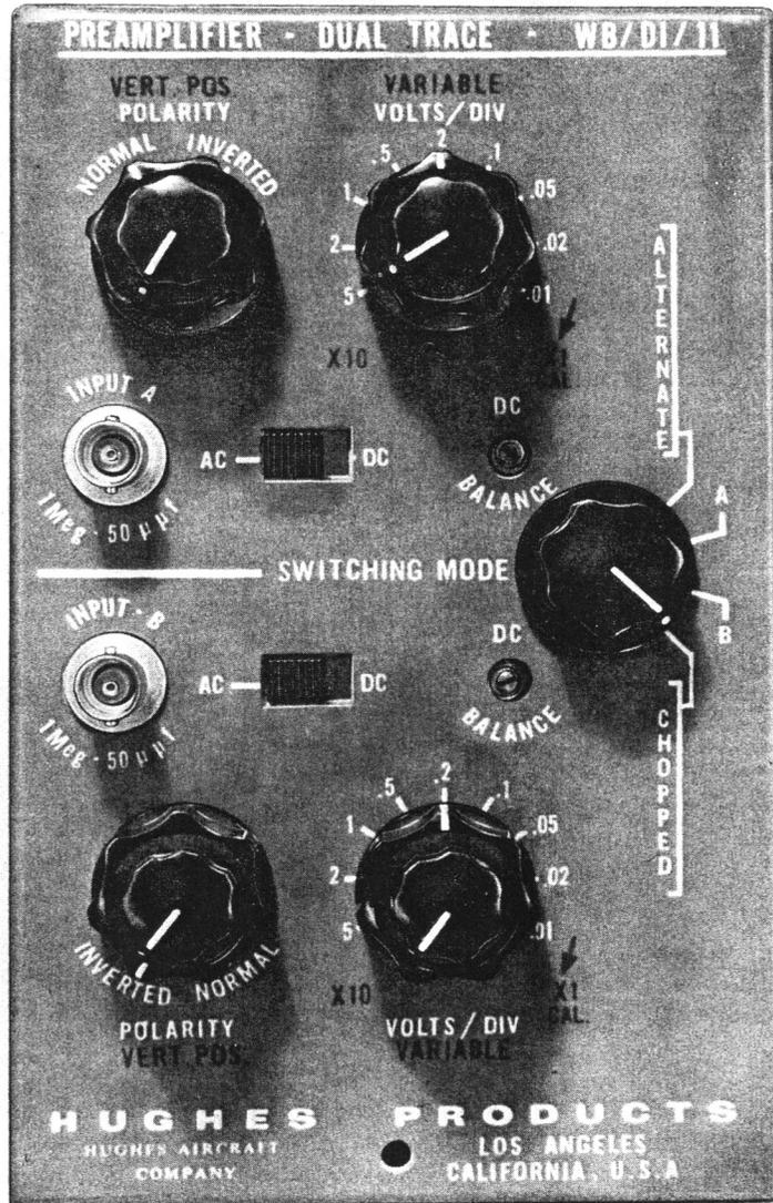
Figure 18. Front Panel, WB/DI/11 or WB/DI/11-D Dual Trace Preamplifier
