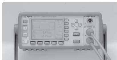
Figure 14. E4417A power meter configured to show a trace display (upper window) and a dual numeric display (lower window)
