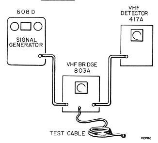
Measure direct input impedance of long cable length (250-500 ft) terminated in approximate  ${\rm Z_0}$ . 803A is direct reading. 1
