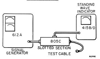
Cut cable to approximately 1/8 wavelength. Plot open circuit and short circuit impedance on Smith Chart. Convert to reactance. 2
