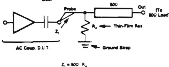
If all circuits to be tested are ac coupled, then, of course, a shunt resistor directly to ground could be used to lower the load impedance. For dc coupled outputs, such a resistor might dissipate excessive power (0.5W for 50 ohms and 5V bias), and complicates the measurement of circuit dc currents and voltages.
