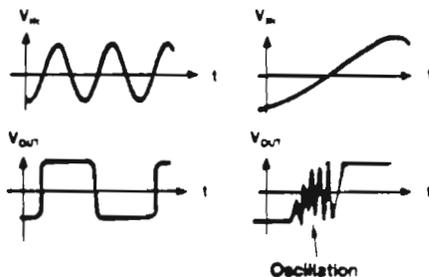
Some digital circuits require a fast risetime input, and will not function properly with a low frequency input (making them the digital counterpart of the analog bandpass circuit). As risetime requirements drop into the nanosecond range for circuits like GaAs prescalers, traditional probing methods are no longer adequate.
