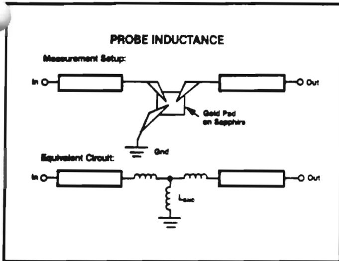
Probe inductance was measured as shown here. For confirmation, a similar measurement was made of the inductance of two probes in series (by using a monitor line connected directly to the input line at the input probe, instead of the output line shown here).
