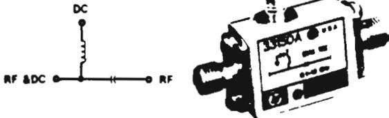
Bias T's combine dc biases and RF signals to the circuit under test. A 50-ohm termination on the RF port provides a controlled impedance for lines which do not carry RF signals. The bias T shown is specified from 0.1 to 18 GHz, and is small enough to be supported by a short semi-rigid cable from the coaxial connector in the probe frame.
