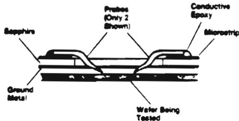
A small bending jig is used to form the probes to the shape shown. If the probes are chemically etched parts, then strips of 20 or more probes can be bent (and sharpened) simultaneously. During assembly, probes are aligned by hand under a microscope to contact the pads of the type circuit to be tested. Tacky conductive epoxy holds the probes in place. After curing, a layer of non-conductive epoxy (not shown) is added over the probes for extra strength.
