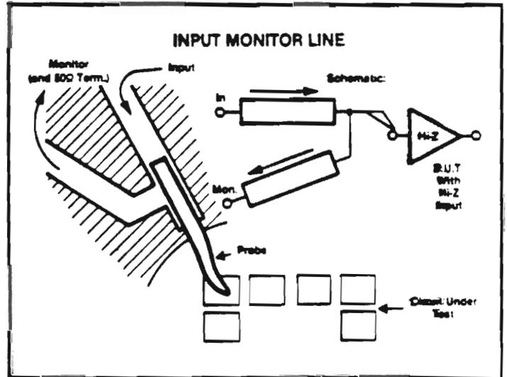
The type of monitor line shown above also provides a 50 ohm termination for the input line, which is usually desirable for minimizing measurement errors. However, it is possible to take advantage of the open-circuit voltage-doubling effect to get a larger input voltage than the source provides into 50 ohms; two methods are shown here. (B) is less susceptible to mismatch errors on the monitor line. Bias T's on all lines (not shown) allow dc bias to be applied to the input.
