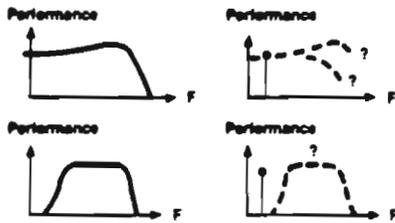
Full frequency testing eliminates marginal chips, and can dramatically improve yields at later stages of assembly. For bandpass circuits, low frequency testing may be worthless. ("Performance" could refer to gain, output power, return loss, relative harmonics, signal-to-noise ratio, etc.)
